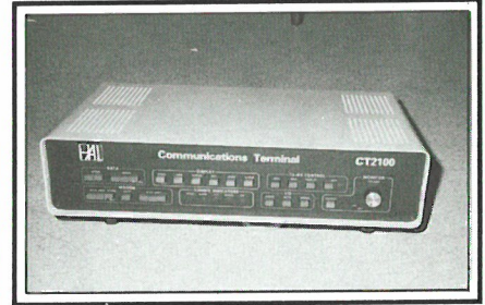
The heart of the system is the CT-2100 communications terminal. It measures about 16 1/2" x 4" x 10 1/2".
