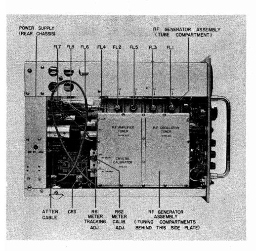
Figure 7-1. Signal Generator TS-510A/U Left Side View, Cover Removed
