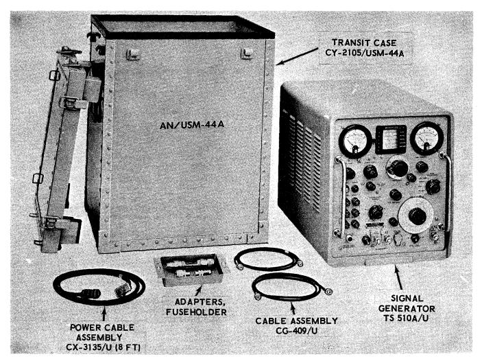
Figure 1-2. Signal Generator AN/USM-44A (Hewlett-Packard), Equipment Supplied
