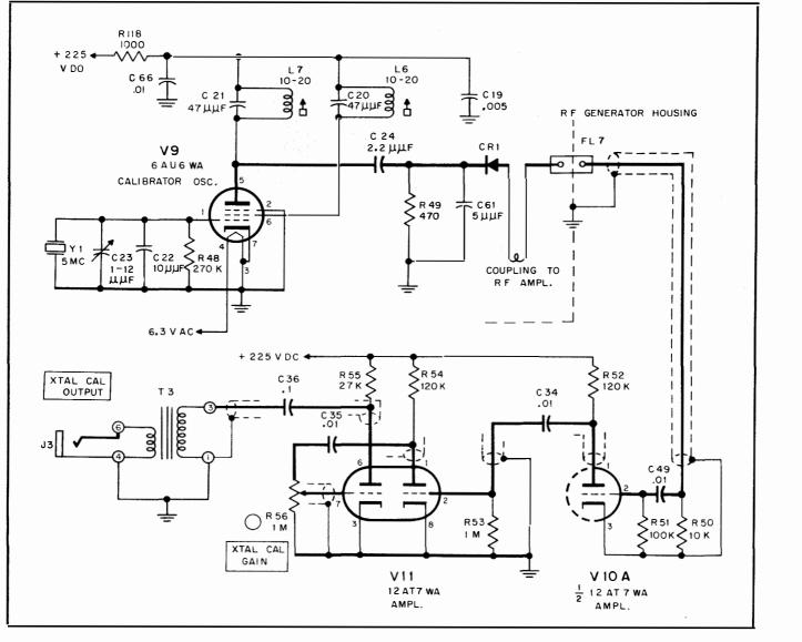
Figure 4-7. Schematic Diagram of Crystal Controlled Frequency Calibrator
