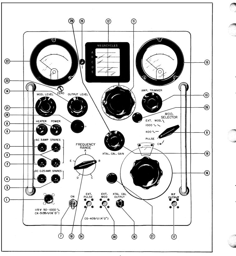
Figure 1-3. Signal Generator TS-510/U, Front Panel Controls
