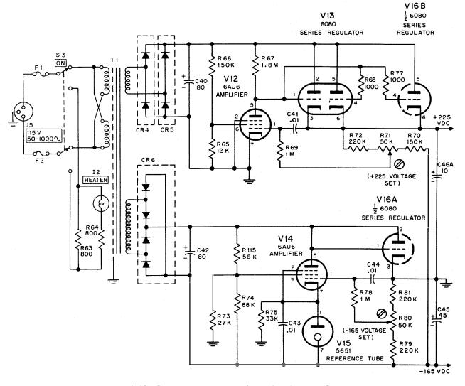
Figure 4-13. Schematic Diagram of Regulated Power Supplies
