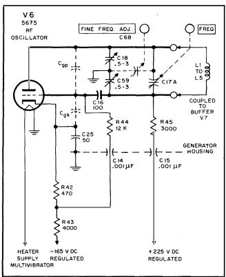
Figure 4-3. Schematic Diagram of Radio Frequency Oscillator
