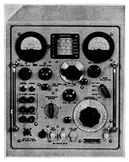
Figure 1-2B. Signal Generator TS-510A/U(\*)
