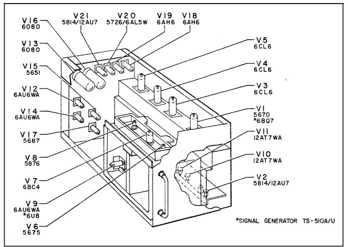
Figure 4-1. Tube Location Diagram
