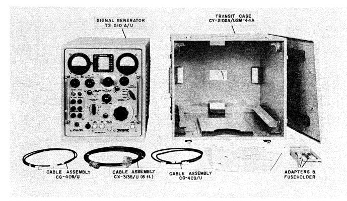
Figure 1-1B. Signal Generator AN/USM-44A (Nuclear Electronics), Equipment Supplied
