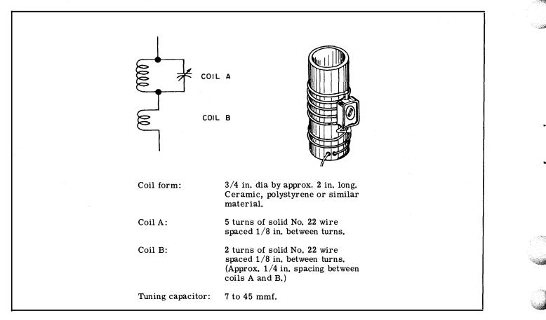
Figure 6-9. Special R-F Transformer Used for Measuring Percentage Modulation
