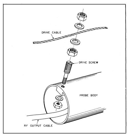
(a) Probe and Cable Attaching Parts
