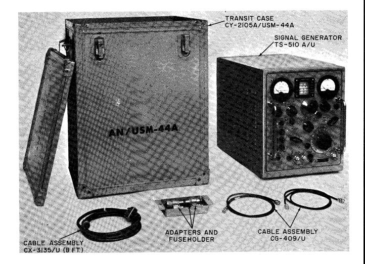
Figure 1-1C. Signal Generator AN/USM-44A (Jetronic Industries), Equipment Supplied
