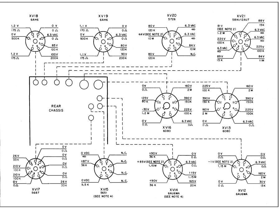
Figure 7-6. Tube Socket Voltage-Resistance Diagram, Power Supply Section
