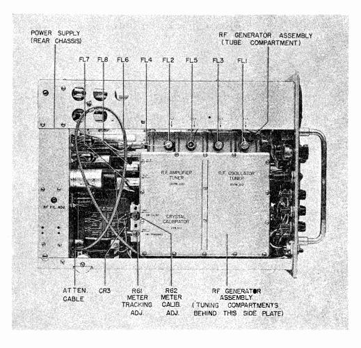
Figure 7-1. Signal Generator TS-510A/U Left Side View, Cover Removed Changed 15 January 1966
