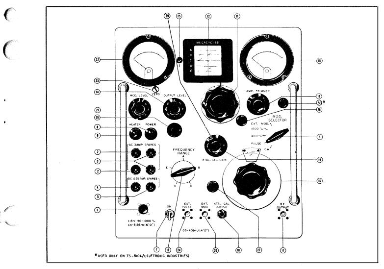
Figure 2-3. Signal Generator TS-510A/U (Nuclear Electronics and Jetronic Industries), Front Panel Controls
