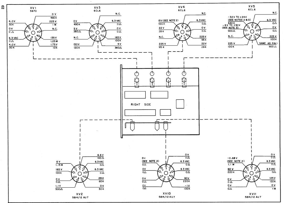
Figure 7-8. Tube Socket Voltage-Resistance Diagram, Modulator Section
