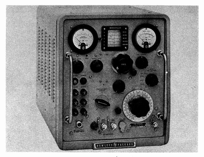
Figure 1-4. Signal Generator TS-510/U (Hewlett-Packard)
