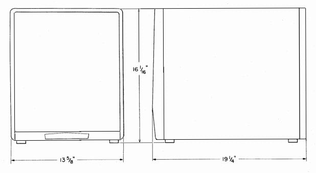
Figure 7-11. Signal Generator TS-510A/U Cabinet Dimensions
