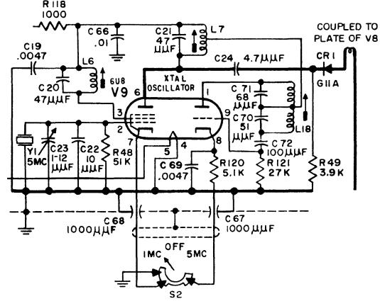
Figure 4-7A. Scehmatic Diagram of Crystal Controled Frequency Calibrator TS-510A/U
