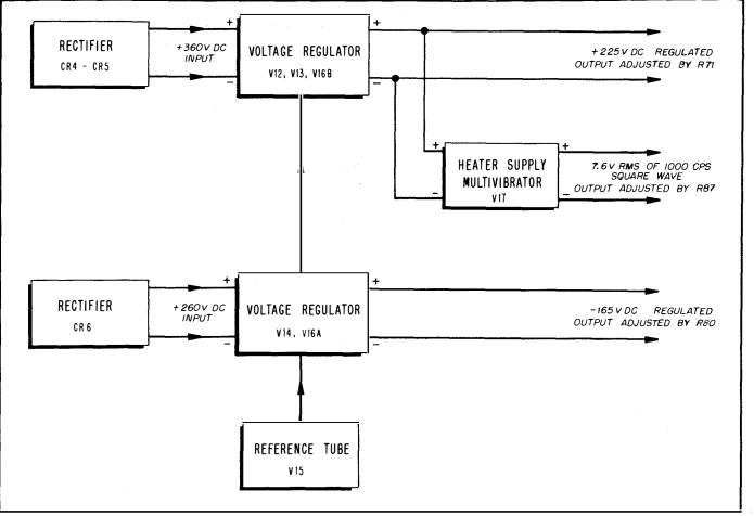
Figure 5-2. Power Supply Block Diagram
