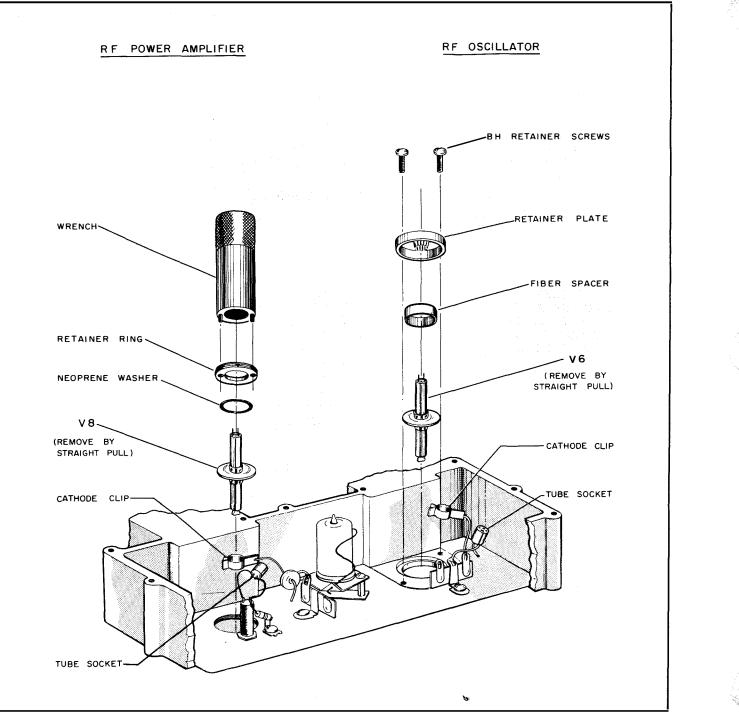
Figure 6-2. Exploded View for Replacement of R-F Oscillator and Amplifier Tubes
