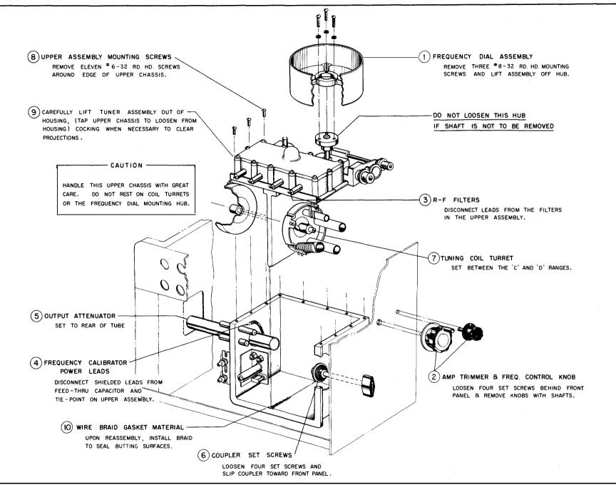
Figure 6-6. Diagram Showing Removal of Frequency Drive Assembly from R-F Generator Housing
