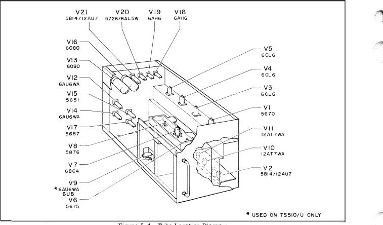
Figure 5-4. Tube Location Diagram
