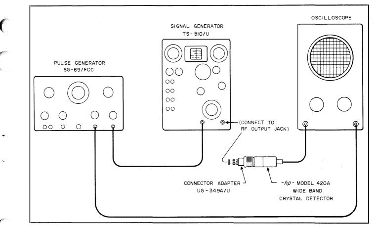
Figure 6-12. Test Set-Up for Measuring R-F Output Pulse
