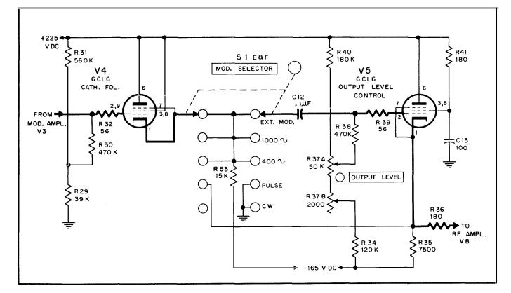
Figure 4-10. Schematic Diagram of Modulation Cathode Follower and Output Level Control Tube Revised 15 January 1960
