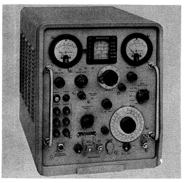
Figure 1-2A. Signal Generator TS-510A/U(\*\*)
