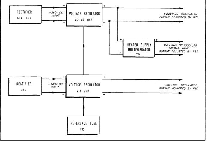
Figure 5-2. Power Supply Block Diagram
