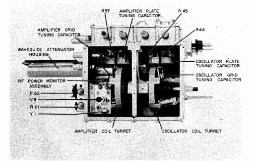
Figure 7-2. R-F Generator Assembly, Inside View of Tuner Compartments
