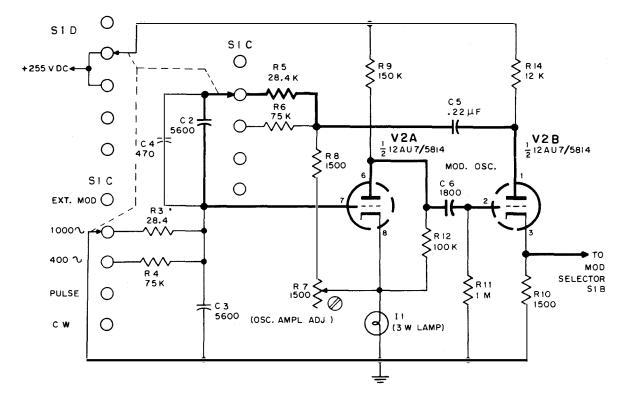
Figure 4-8. Schematic Diagram of Modulation Oscillator
