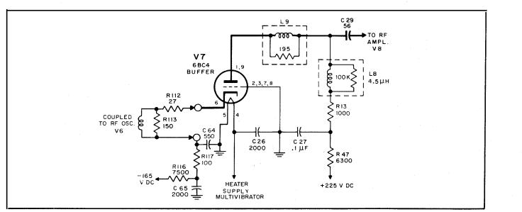
Figure 4-4. Schematic Diagram of Buffer Amplifier
