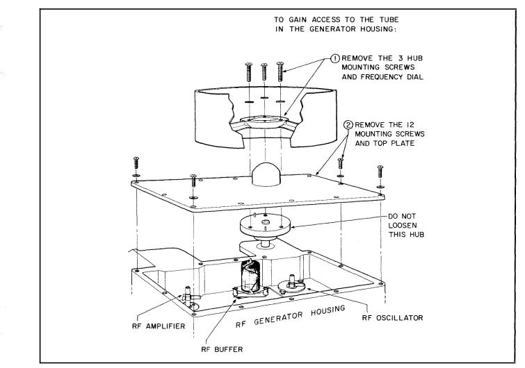
Figure 6-1. Diagram Showing Access to R-F Oscillator, Buffer and Amplifier Tubes
