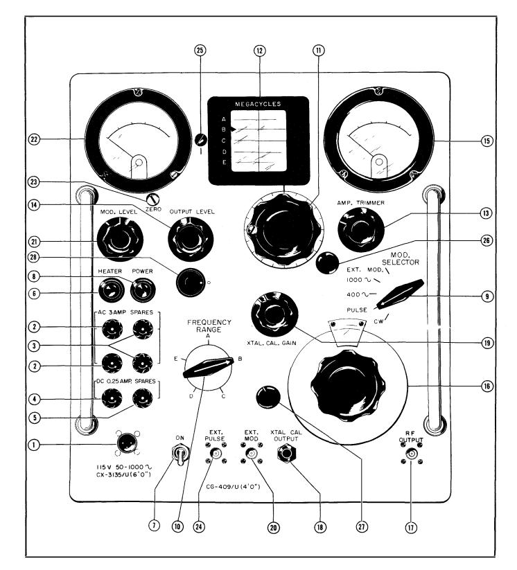
Figure 1-3A. Signal Generator TS-510A/U(\*), Front Panel Controls
