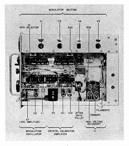
Figure 7-4. Signal Generator TS-510A/U Right Side View, Cover Removed
