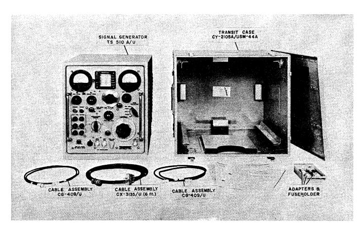
Figure 1-3. Signal Generator AN/USM-44A (Nuclear Electronics), Equipment Supplied
