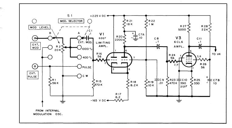
Figure 4-9. Schematic Diagram of Modulation Limiter and Amplifier
