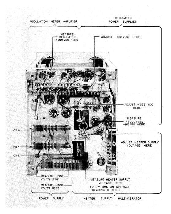
Figure 5-3. Power Supply Section Showing Points of Voltage Measurement and Adjustment
