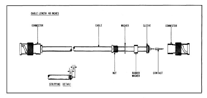
Figure 2-1. Fabrication of Video Cord CG-409/U
