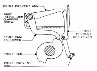
Figure 5-69. Print Prevent Arm Engaged With Print Prevent Rod Lever
