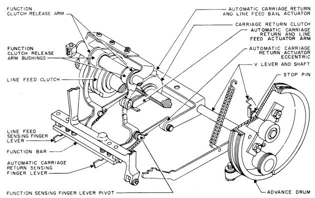
Figure 5-62. Automatic Carriage Return and Line Feed Linkage
