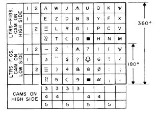
Figure 5-70. Plan View Of Print Cylinder
