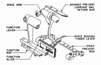
Figure 4-27. Function Selector, Space Linkage
