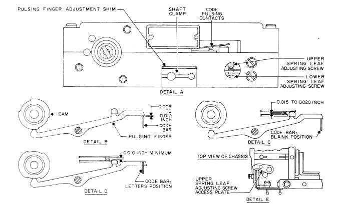
Figure 5-78. Keyboard Adjustment, Parts Location
