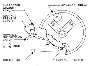
Figure 5-56. Advance Prevent Lever Engaged With Advance Suppression Latch
