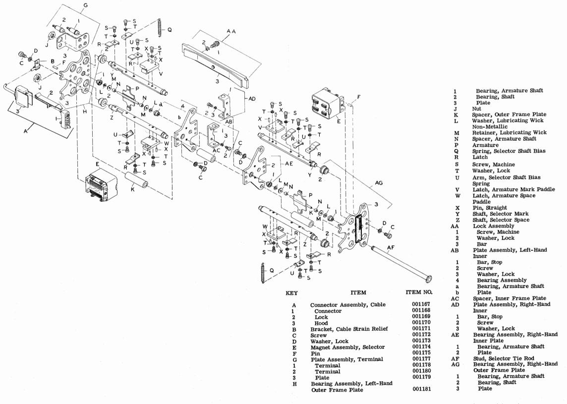
Figure 5-26 Selector Assembly (AN/TGC-14(V) Only) SL-4-03315 Figure 22
