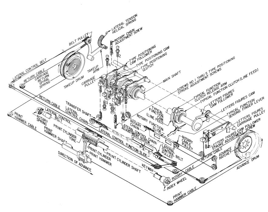
Figure 4-19. Print Cylinder and Print Hammer Positioning System
