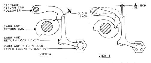
Figure 5-61. Carriage Return Lock Lever Eccentric Bushing Adjustment
