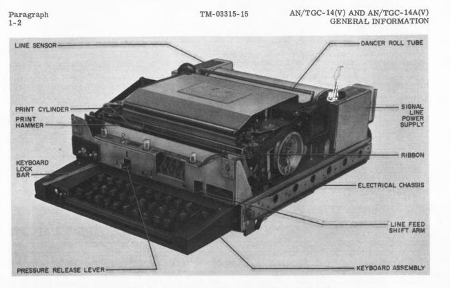
Figure 1-5. Teletypewriter Set, Case and Cover Removed
