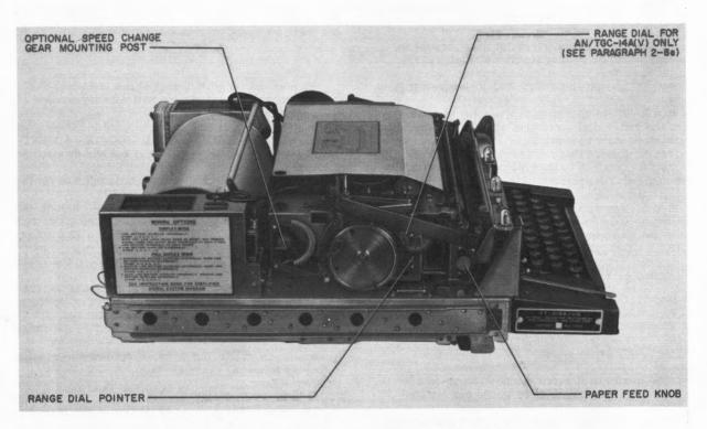
Figure 2-8. Printer and Electrical Chassis, Left-Side View
