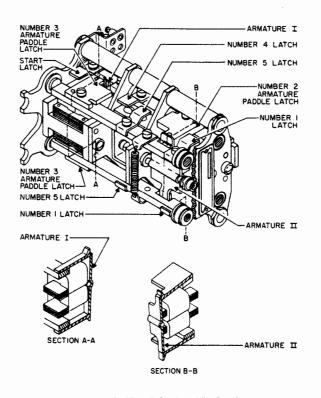
Figure 4-15. Selector Mechanism
