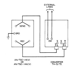
Figure 2-15. External Line Patching, Typical Connection Circuit
