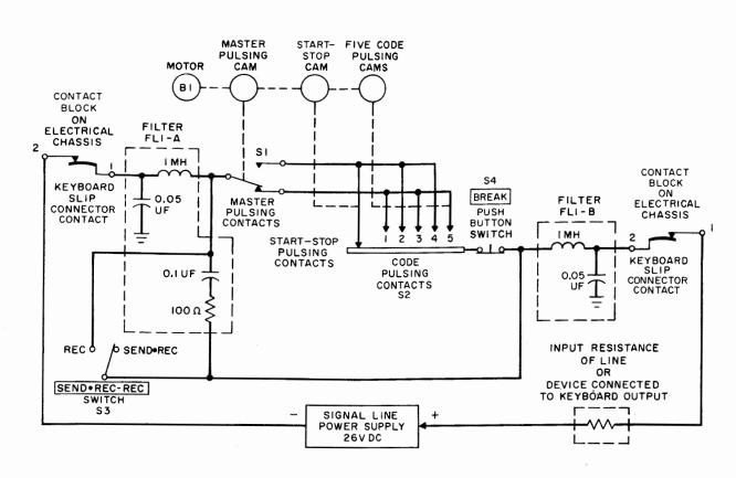
Figure 4-8. Keyboard 1A9, Simplified Schematic Diagram
