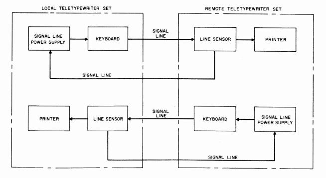
Figure 4-4. Full-Duplex Mode, Functional Block Diagram
