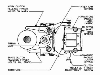
Figure 4-16. Selector, Clutch Release Mechanism
