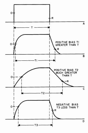
Figure 4-38. Effect of Series Inductance on Pulse Lengths
