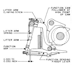
Figure 5-53. Function Shaft Adjustment
