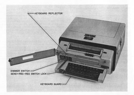
Figure A3-1. Control Locations of TT-299B/UG Teletypewriter
