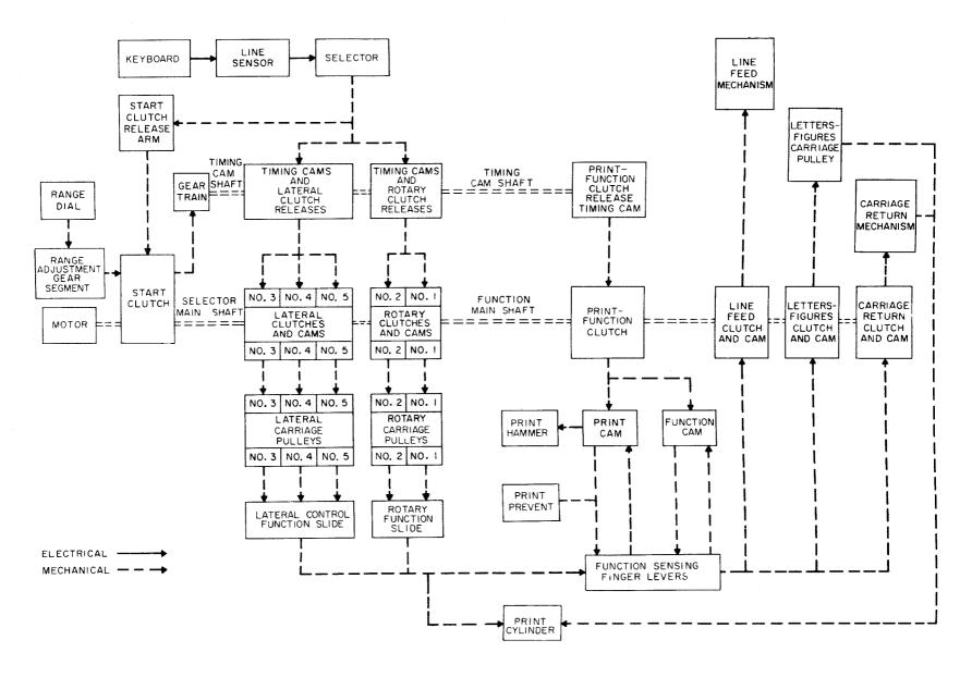
Figure 4-14. Printer 1A2, Functional Block Diagram
