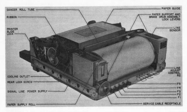
Figure 2-1. Printer and Electrical Chassis, Parts Location
