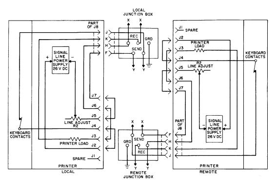
Figure 2-14. Patching Mode 5, Simplified Wiring Diagram
