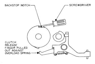
Figure 5-47. Advancing Clutches Manually
