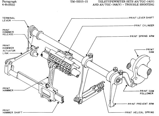
Figure 4-29. Function Selector, Character Printing Linkage
