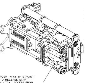
PUSH IN AT THIS POINT TO RELEASE START CLUTCH. (ACCESS FROM BOTTOM OF PRINTER)-----
