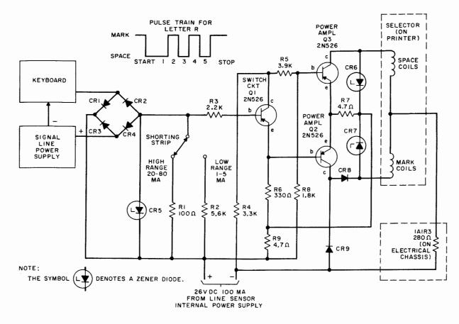
Figure 4-11. Line Sensor 1A3, Simplified Schematic Diagram
