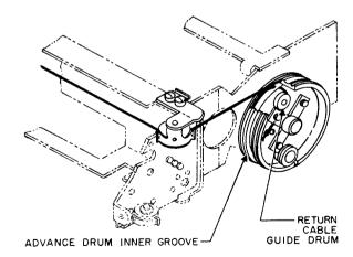
Figure 5-16. Return Cable Installation, Securing Cable to Advance Drum
