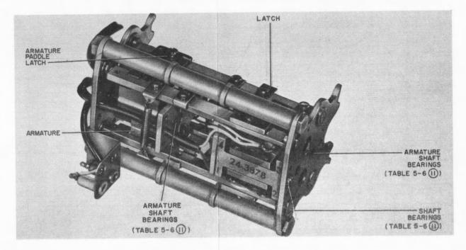
Figure 5-10. Selector Assembly, Lubrication Points
