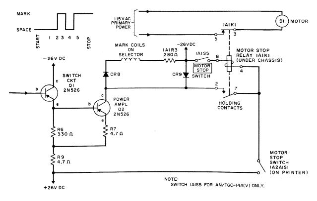
Figure 4-12. Line Sensor 1A3, Motor Stop Function, Simplified Schematic Diagram
