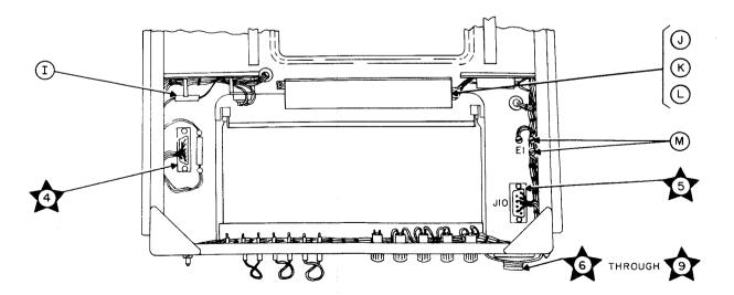
Figure 4-37. Electrical Chassis 1A1, Location of Test Points
