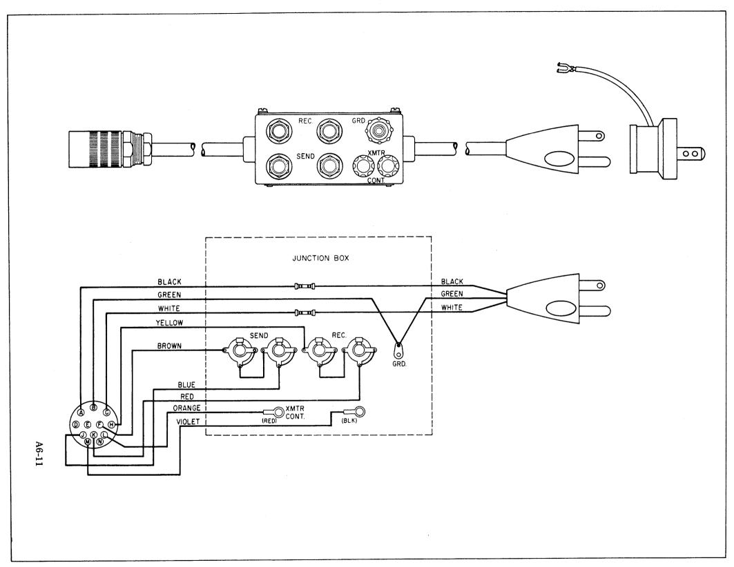
Figure A4-3. Bench Test Cable
