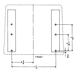
Figure 2-4. Tactical Case CY-2976/PG, Shock Mounted Installation, Mounting Holes Location
