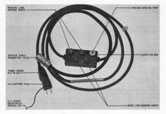
Figure 1-6. Service Cable Assembly
