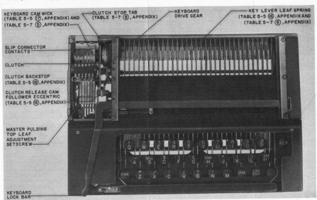
Figure 5-9. Keyboard Assembly, Top View
