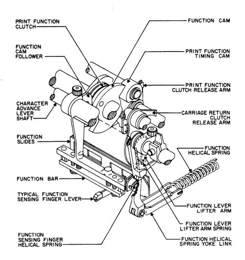
Figure 4-24. Function Selector, Start of Function Cycle
