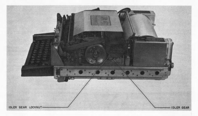
Figure 2-16. Printer and Electrical Chassis, Right-Side View
