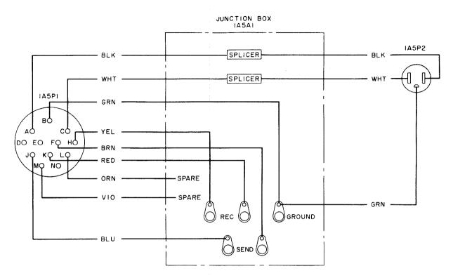
Figure 5-91. Service Cable, Wiring Diagram
