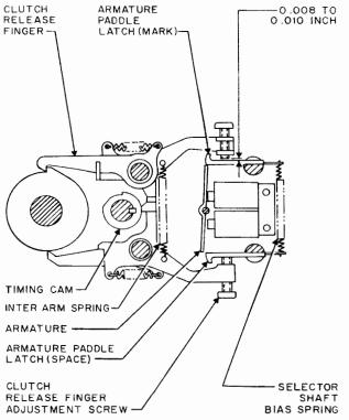
Figure 5-50. Selector Linkage Adjustment
