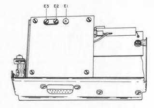
Figure 2-9. Line Sensor Range Adjustment, Parts Location
