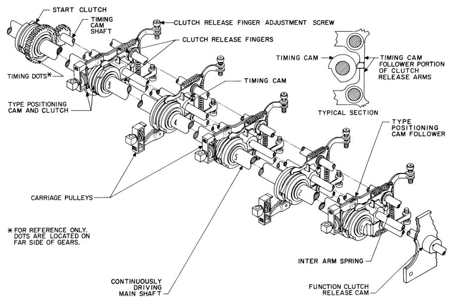
Figure 4-22. Print Cylinder Positioning Clutch Release System
