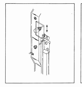
Figure A5-5. Pin Retaining Plate
