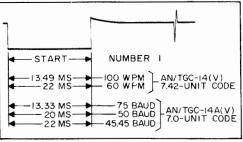
Figure 5-82. Waveform For Timing Adjustment
