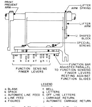
Figure 5-55. Function Bar and Function Sensing Finger Lever Alignment
