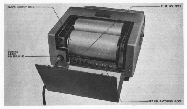
Figure 1-4. Teletypewriter Set, Rear View
