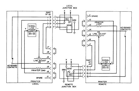
Figure 2-11. Patching Mode 2, Simplified Wiring Diagram
