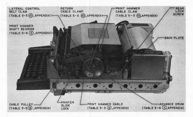
Figure 5-3. Teleprinter Assembly, Right-Side View
