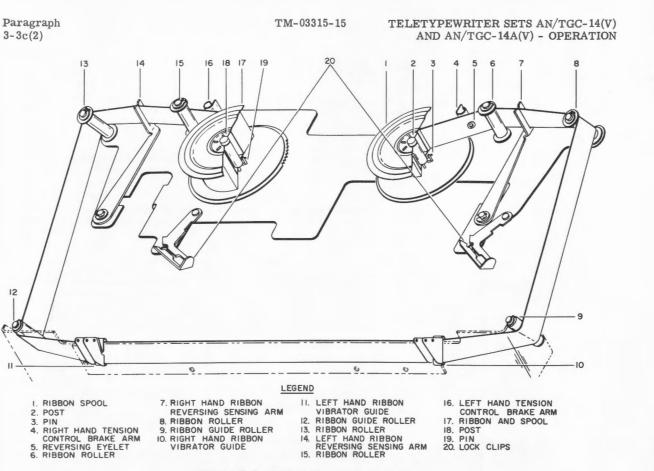
Figure 3-2. Ribbon Threading Diagram
