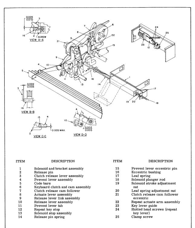
Figure A5-4. Keyboard Interlock Mechanism
