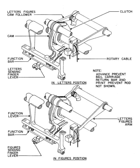
Figure 4-28. Function Selector, Letters Figures Linkage
