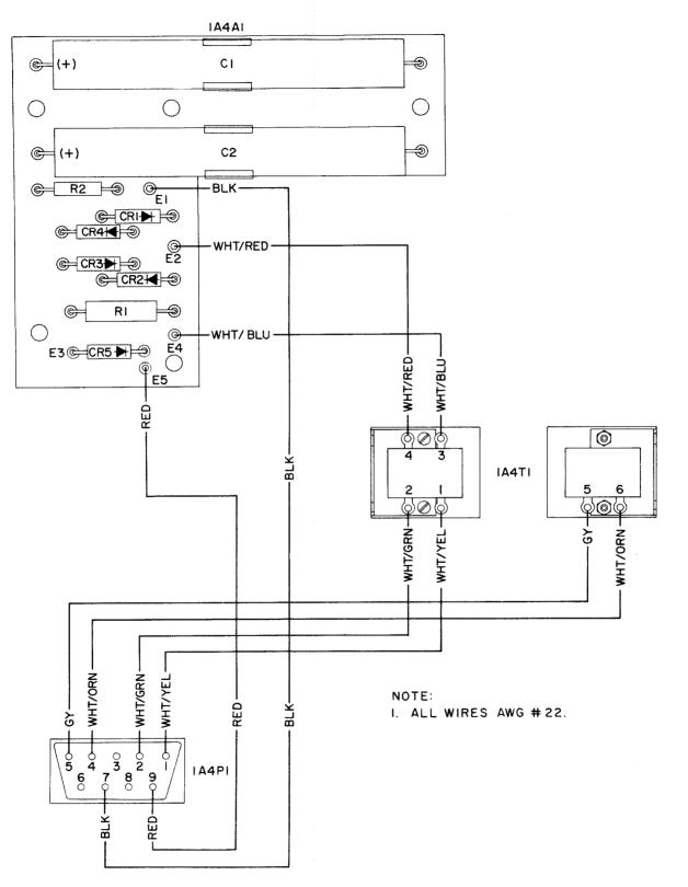
Figure 5-89. Signal Line Power Supply, Wiring Diagram
