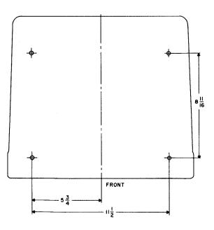
Figure 2-3. Tactical Case CY-2976/PG, Low Vibration Installation, Mounting Holes Location
