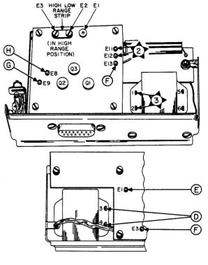
Figure 4-13. Line Sensor 1A3, Location of Test Points
