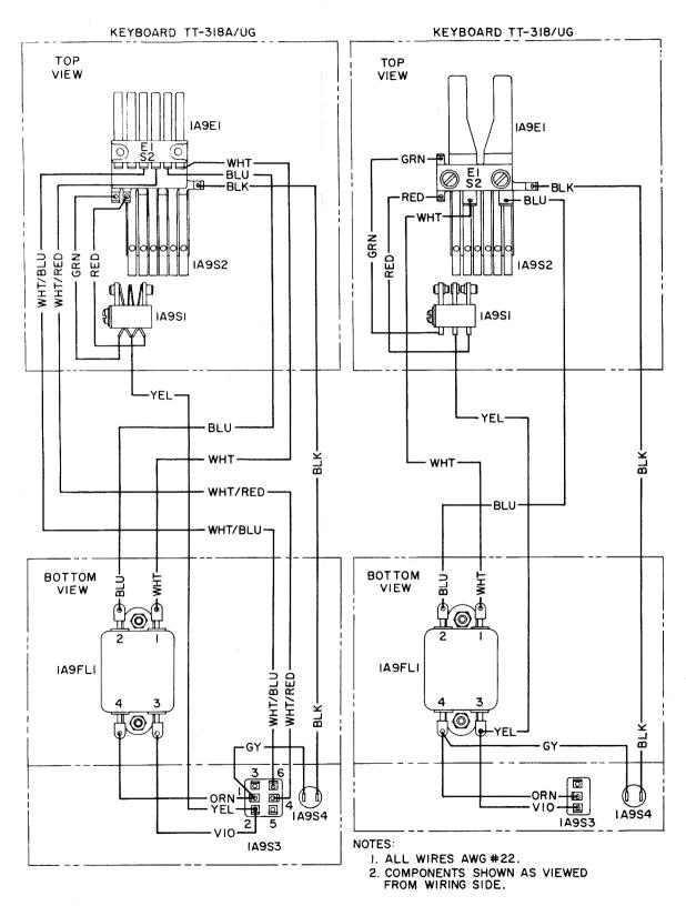
Figure 5-90. Keyboard TT-318/UG and TT-318A/UG, Wiring Diagram
