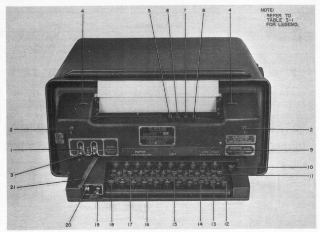
Figure 3-1. Operator's Controls
