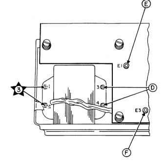
Figure 4-36. Signal Line Power Supply 1A4, Location of Test Points
