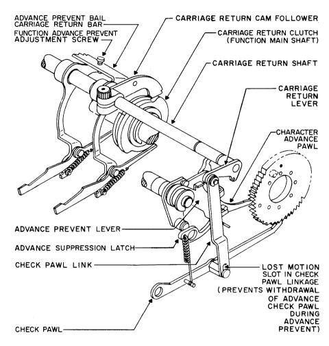
Figure 4-31. Function Selector, Character Advance Prevent Linkage
