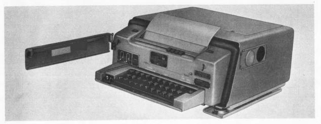
C. Installed in Shock-Mounted Non-Tactical Case CY-2977A/UG
