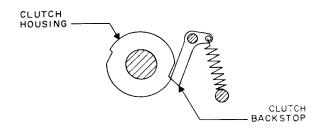
Figure 5-77. Backstop Eccentric Adjustment
