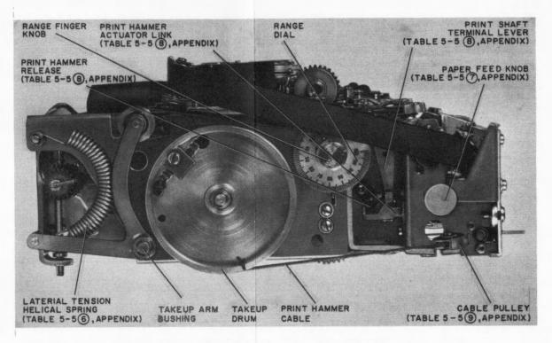
Figure 5-2. Printer Assembly, Left-Side View
