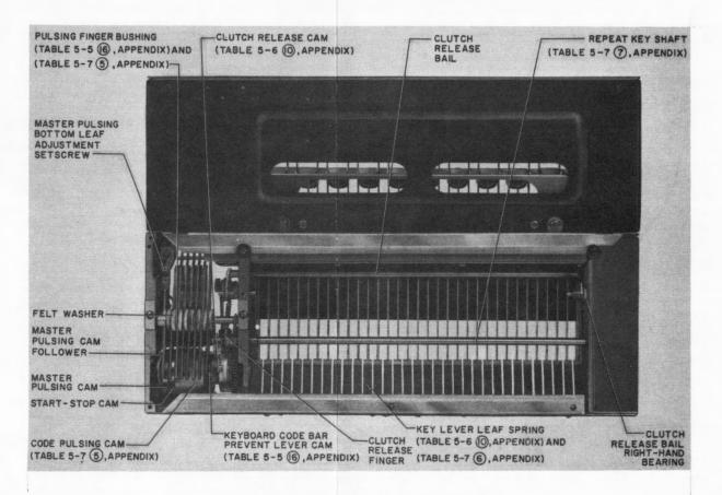
Figure 5-8. Keyboard Assembly, Bottom View
