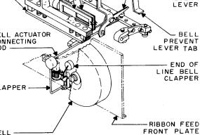
Figure 5-64. Bell Function Linkage
