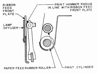
Figure 5-67. Print Hammer Backstroke Adjustment
