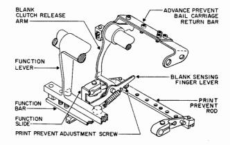
Figure 4-26. Function Selector, Blank Linkage
