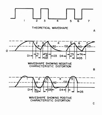
Figure 4-39. Waveshapes Showing Characteristic Distortion
