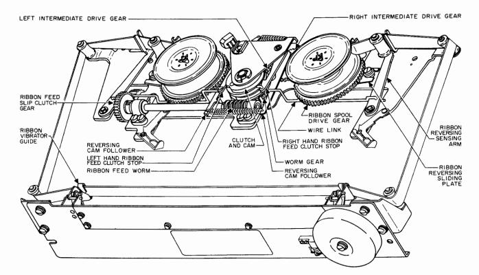
Figure 4-33. Ribbon Feed Mechanism
