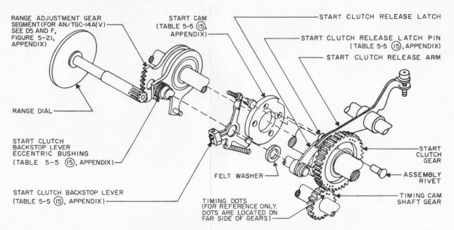
Figure 5-7. Start Clutch Release Mechanism, Exploded View
