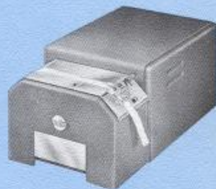
Teletype Model 28 Tape Reader (multi- contact)—Reads 5-, 6-, 7- or 8-level punched tape for sequential (serial) transmission to local or remote receiving equipment. Twin-shaft design offers parallel- wire read-out facilities for business machines or other signal activated equipment.
