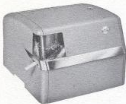
Teletype Model 28 Tape Punch — Receives incoming electrical signals, punches a 5-level "common language" paper tape, and prints the message right on the tape. Accessory reading contacts enable 5-level parallel- wire output to control auxiliary equipment.
