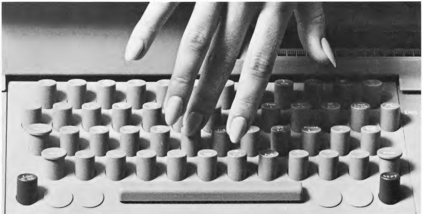
The Eight-Level Keyboard-Punch perforates an eight-level code that is compatible with the American Standard Code for Information Interchange. This means it can communicate with most
