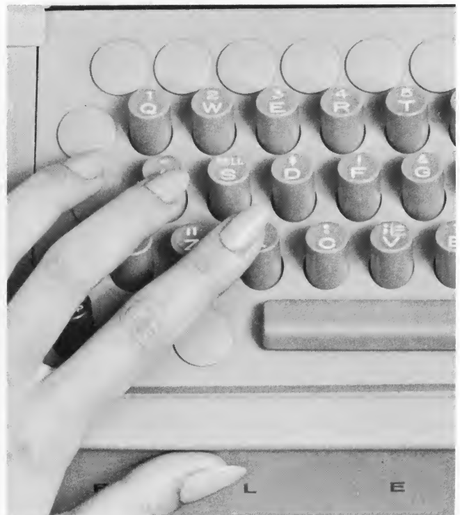
The Five-Level Keyboard-Punch perforates a five-level code. It has a three-row keyboard that uses the "LTRS-FIGS" shift.
