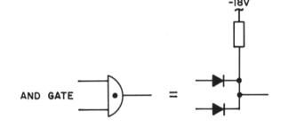
Output is "1" when both inputs are "1".
