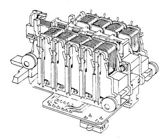
Driving these 9 print wires is a print head consisting of 9 basic units, 5 on the left and 4 on the right, as illustrated above.
