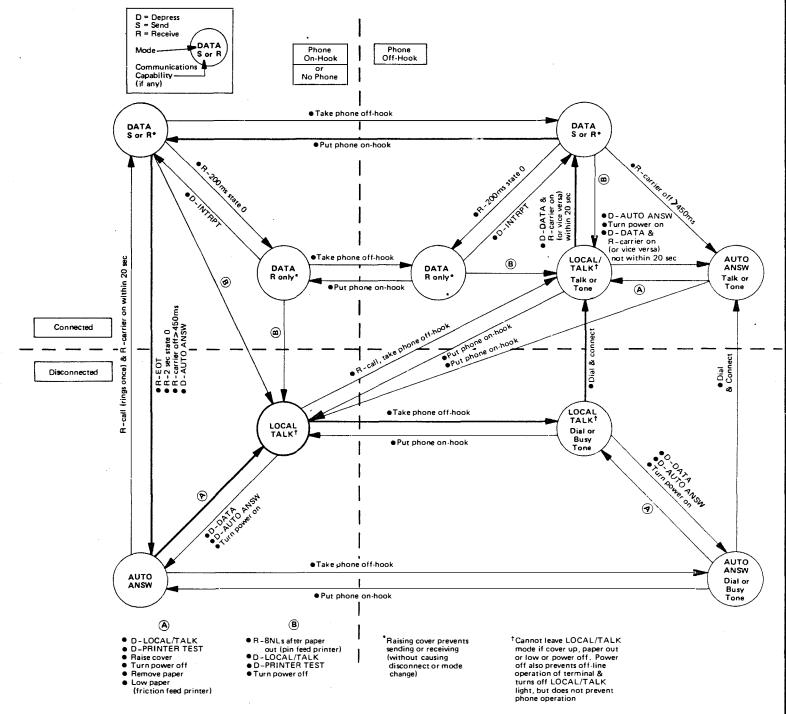
Operating Sequence Diagrams for a KSR with a 103-Type Built-In Modem Interface
