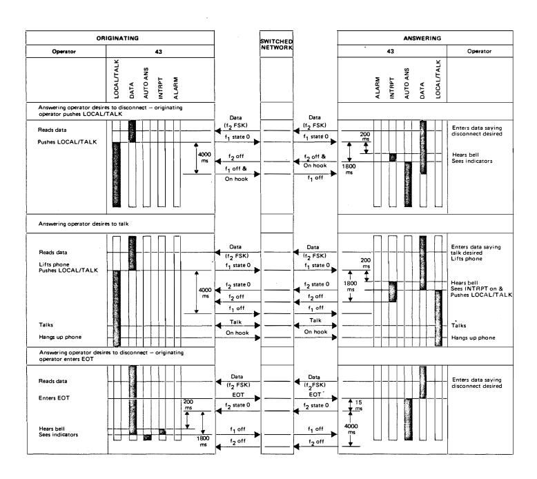
Operating Sequence Diagrams for a KSR with a 103-Type Built-In Modem Interface (cont'd)
