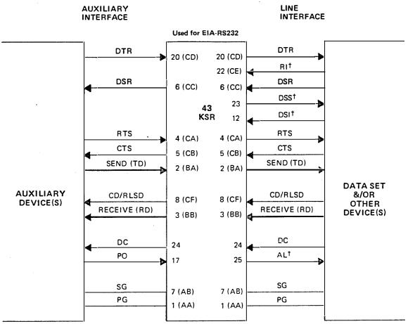
For limited—EIA applications connect pins 5, 6 & 8 (& possibly 20) together to permit operation
