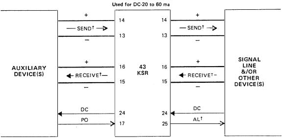
For Full-Duplex current-loop applications connect pins 2 & 6 on auxiliary interface together and connect pins 3, 4, 5, 6 & 8 on line interface together.
