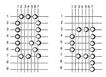
The left-hand character is an upper-case Q, the right-hand a lower-case q. As shown, the printer prints the characters by impacting a column of wires up to 7 at a time and up to 7 times in a row, depending on the character being printed.
