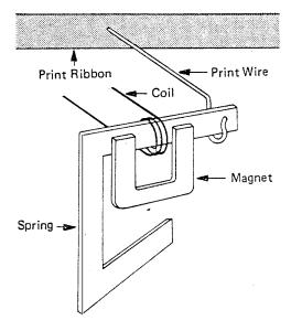
The C shaped part is spring steel and is twisted and held by the magnet as shown. When operated, an electrical pulse in the coil cancels the effect of the magnet on the spring, allowing the spring to push the print wire into the print ribbon and onto the paper as indicated by the arrow. The coil does not move with the spring but allows it to move between preset stops within the coil core.
