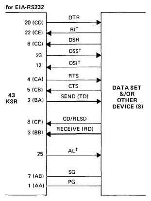
For limited—EIA applications connect pins 5, 6 & 8 (& possibly 20) together to permit operation
