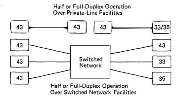
43 terminals can be used for basic terminal-to-terminal data communications over point-to-point or switched-network facilities, in the half or full-duplex mode, to permit alternate or simultaneous sending and receiving between terminals in the system.
