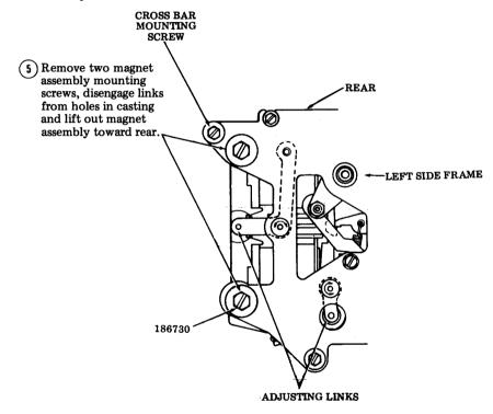
Note: When replacing magnet assembly. use rubber bands, or other means, to hold armatures in engaged position, separated by nylon finger guides.
