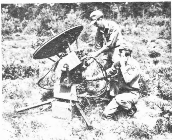
RADIO TERMINAL, SATELLITE COMMUNICATIONS (SHF) AN/USC-79
