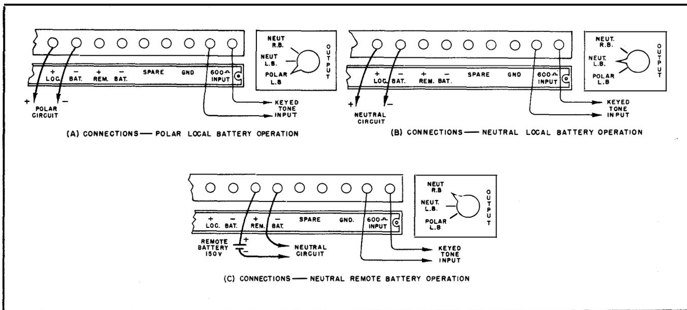
**Figure 3-4. Receiver, Carrier Telegraph R-466/UC, Output Connections**
