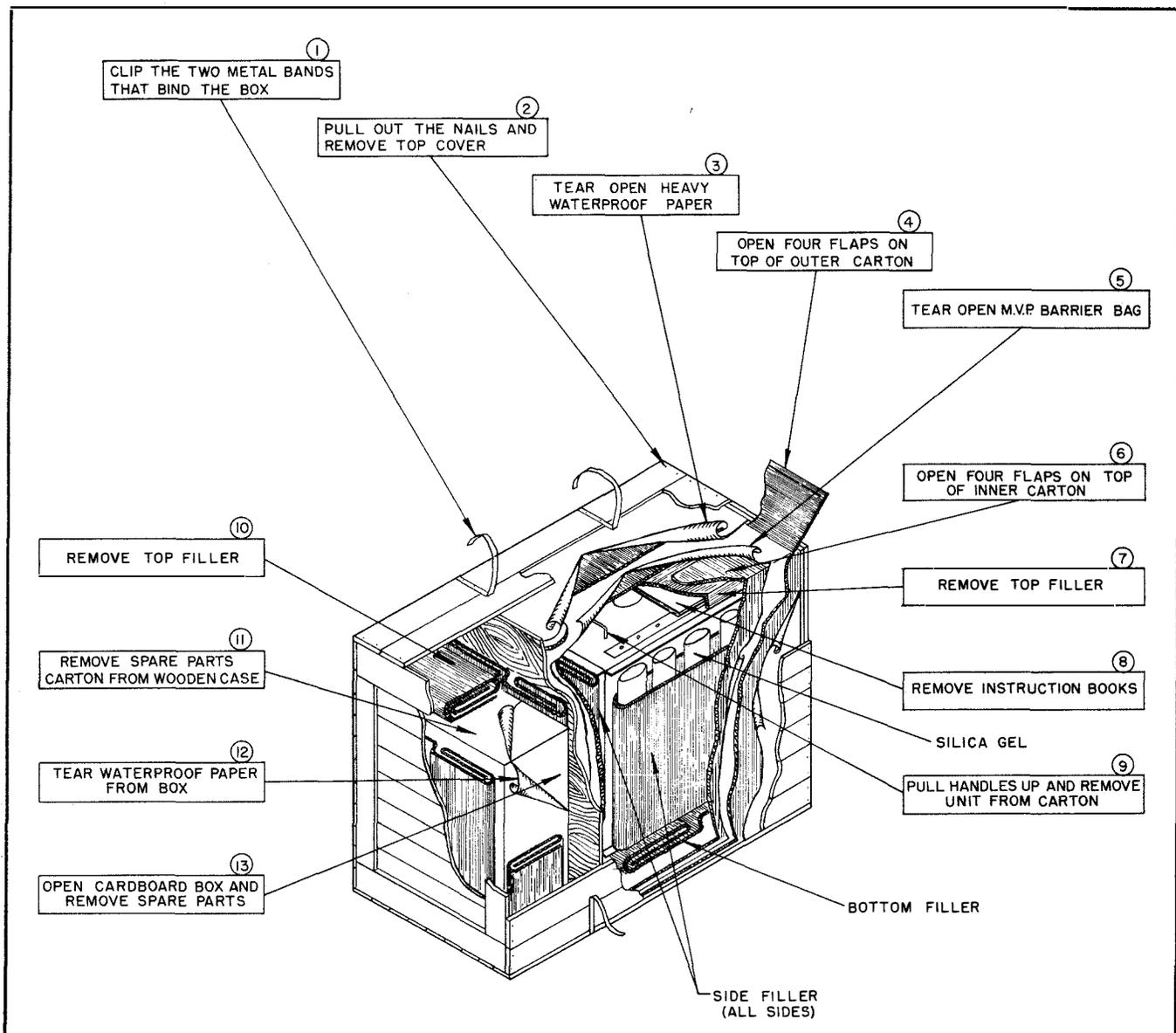
Figure 3-1. Receiver, Carrier Telegraph R-466/UC, Unpacking Procedure
