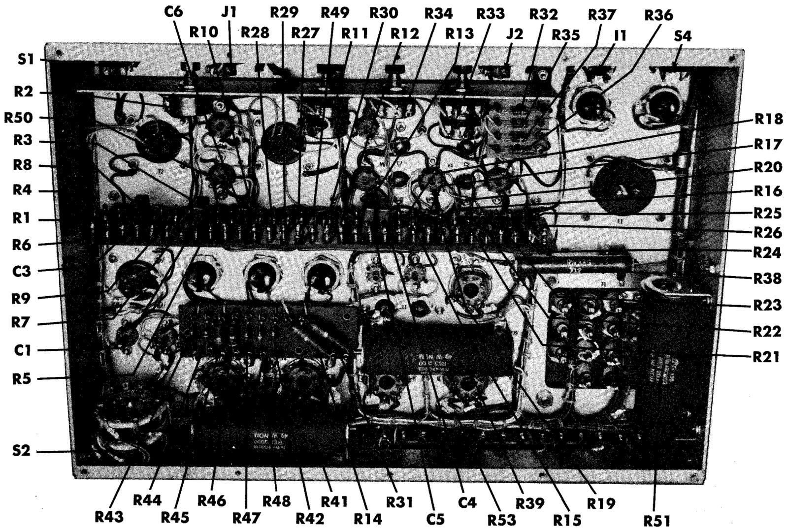
Figure 7-2. Receiver, Carrier Telegraph R-466/UC,
