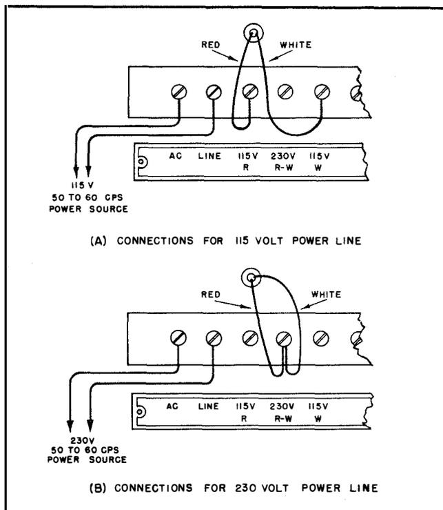
**Figure 3-3. Receiver, Carrier Telegraph R-466/UC, A.C. Power Line Connections**
