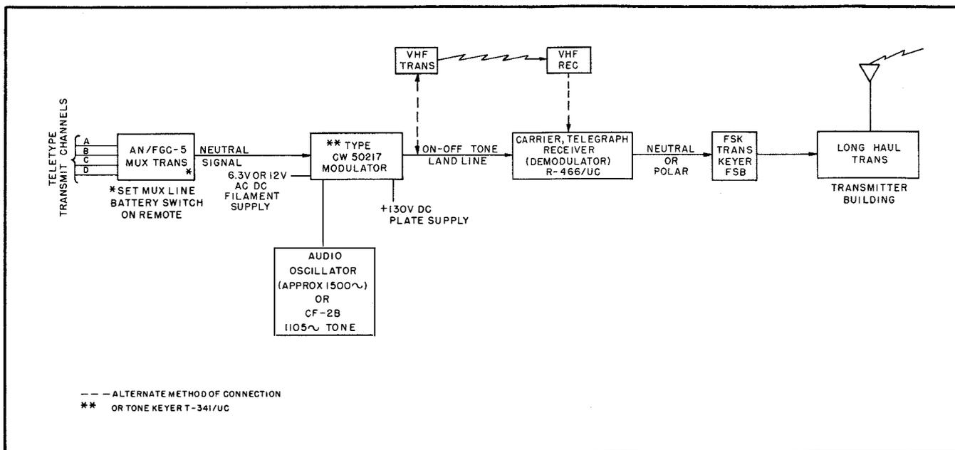
Figure 1-3. Receiver, Carrier Telegraph R-466/UC, Application
