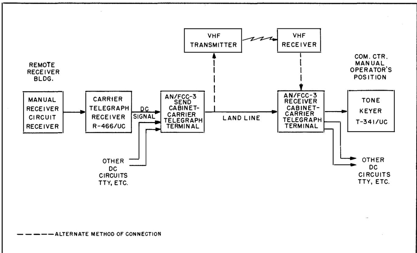
Figure 1-2. Receiver, Carrier Telegraph R-466/UC, Application
