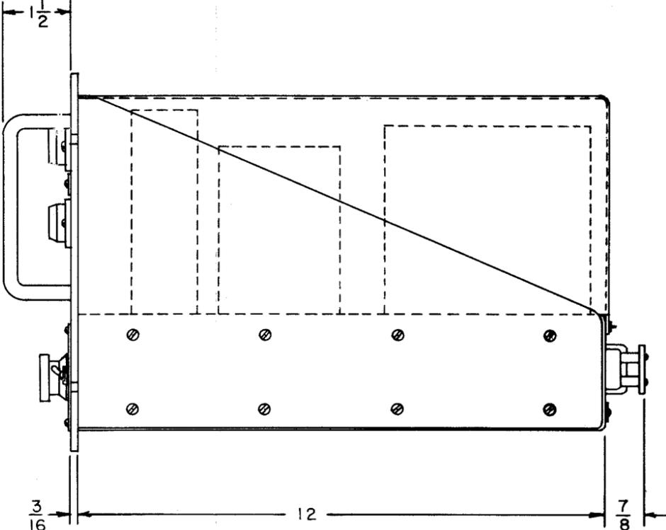
Figure 3-2. Receiver, Carrier Telegraph R-466/UC, Outline Drawing
