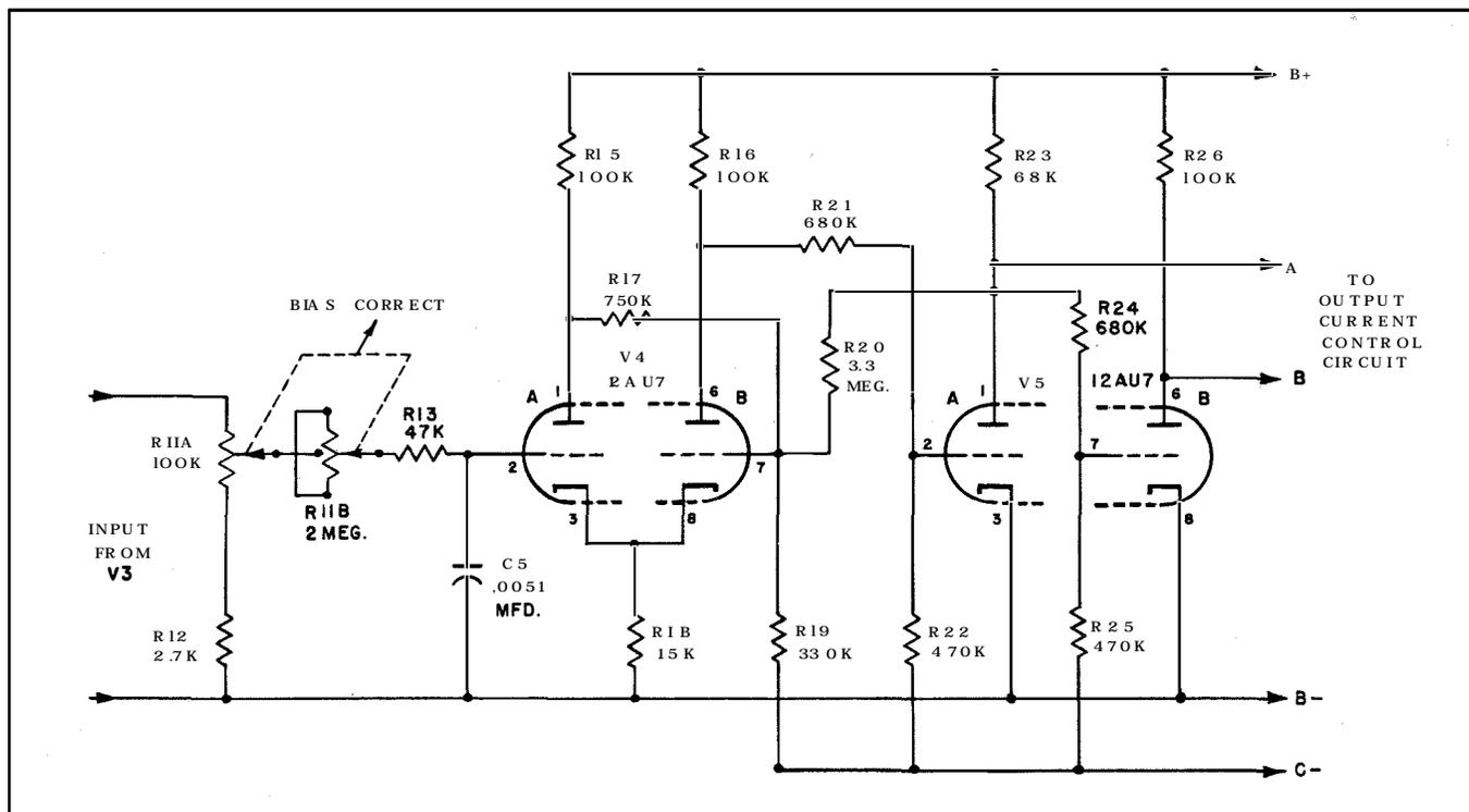
Figure 2-4. Bias Correct and D.C. Squaring Circuits
