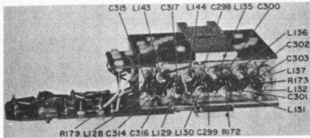
Figure 6-56A. Signal Data Translator CV-1377A/ PRC-47 (A3), VFO Subassembly, Bottom View, Parts Location
