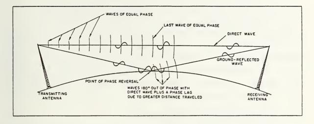
Figure B.9 Direct and ground reflected waves.
