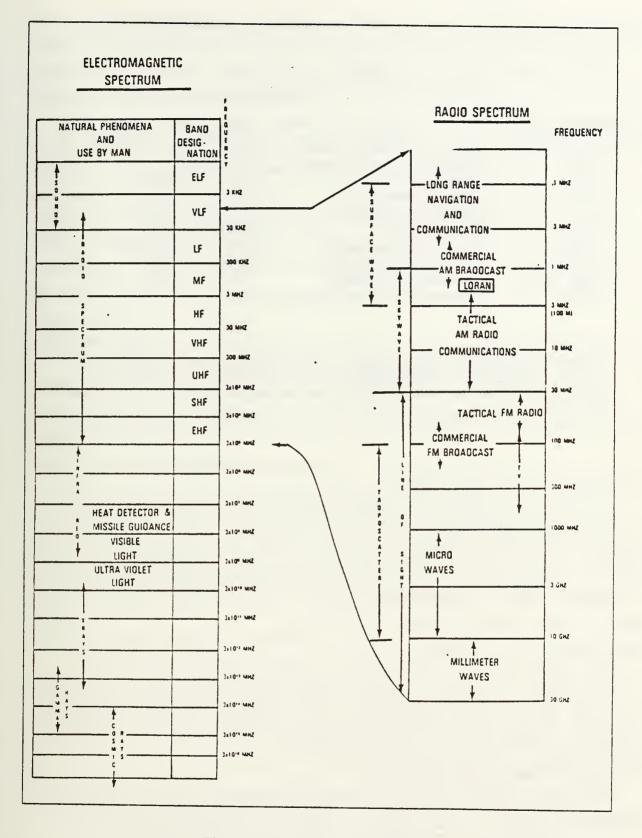
Figure 5.1 Frequency Spectrum.
