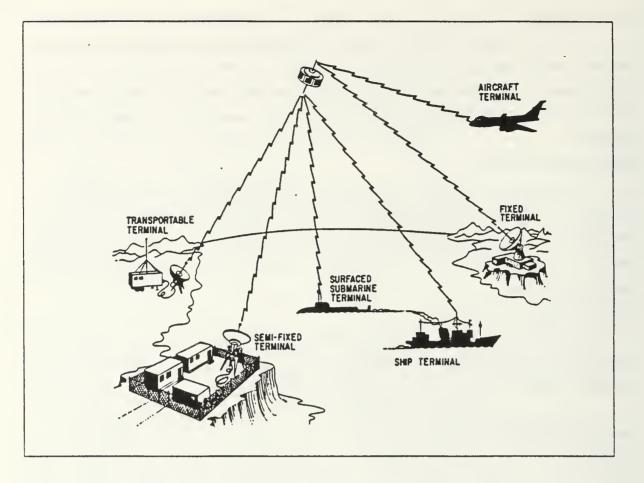
Figure 5.2 Basis Satellite Communications Operations.
