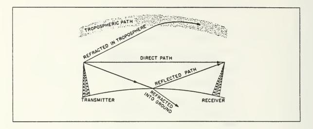
Figure B.8 Possible routes for ground waves.
