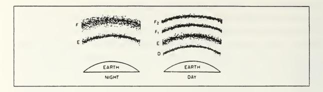
Figure B.12 Ionospheric layers at night and day.
