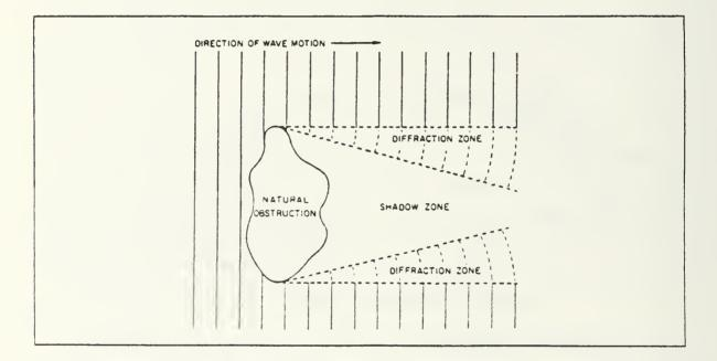
Figure B.2 Diffraction of Waves.
