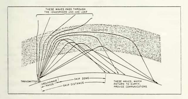
Figure B.10 Possible paths for radio waves.
