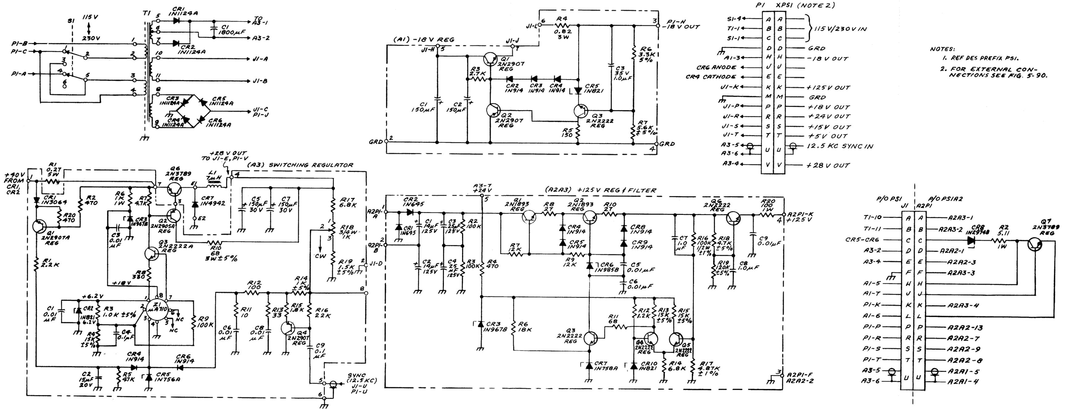
Figure 5-63. Power Supply PS1, Schematic Diagram (Sheet 1 of 2)
