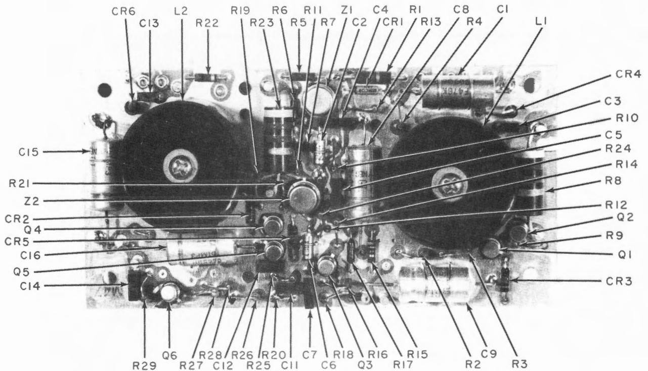
Figure 5-52. +5 and +18 Volt Regulator A2A1, Part of Power Supply PS1, Parts Location
