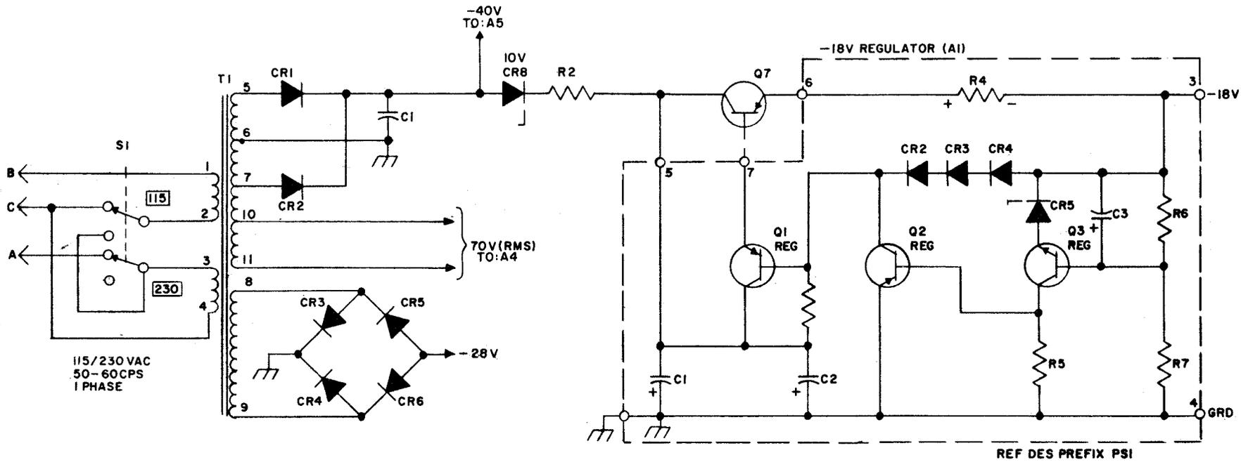
Figure 4-38. Power Transformer and -18 Volt Regulator, Simplified Schematic Diagram
