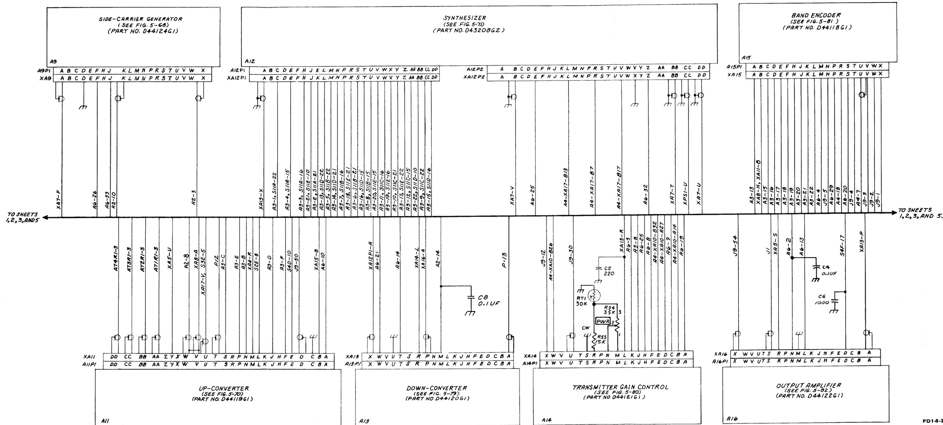
Figure 5-90. Modulator-Synthesizer MD-777/FRT, Front Panel and Chassis Assembly, Interconnection Diagram (Sheet 4 of 5)
