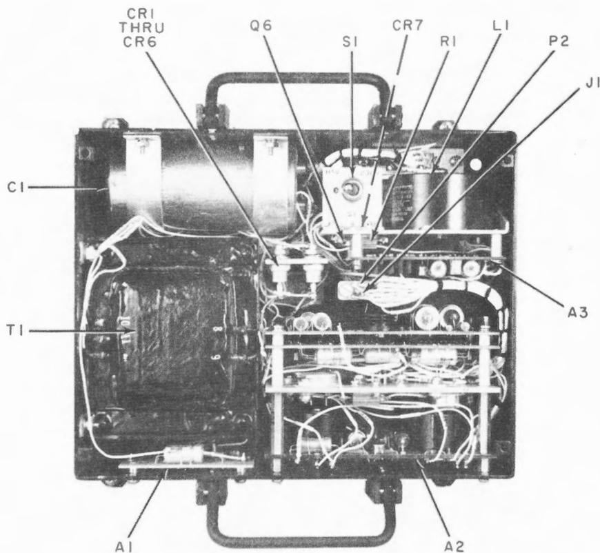
Figure 5-49. Power Supply Module PS1
