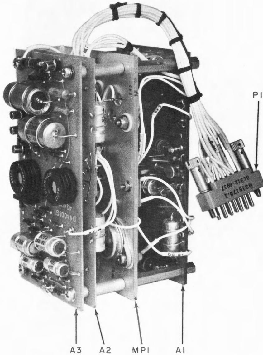
Figure 5-50A. Power Supply Regulator Assembly A2,
