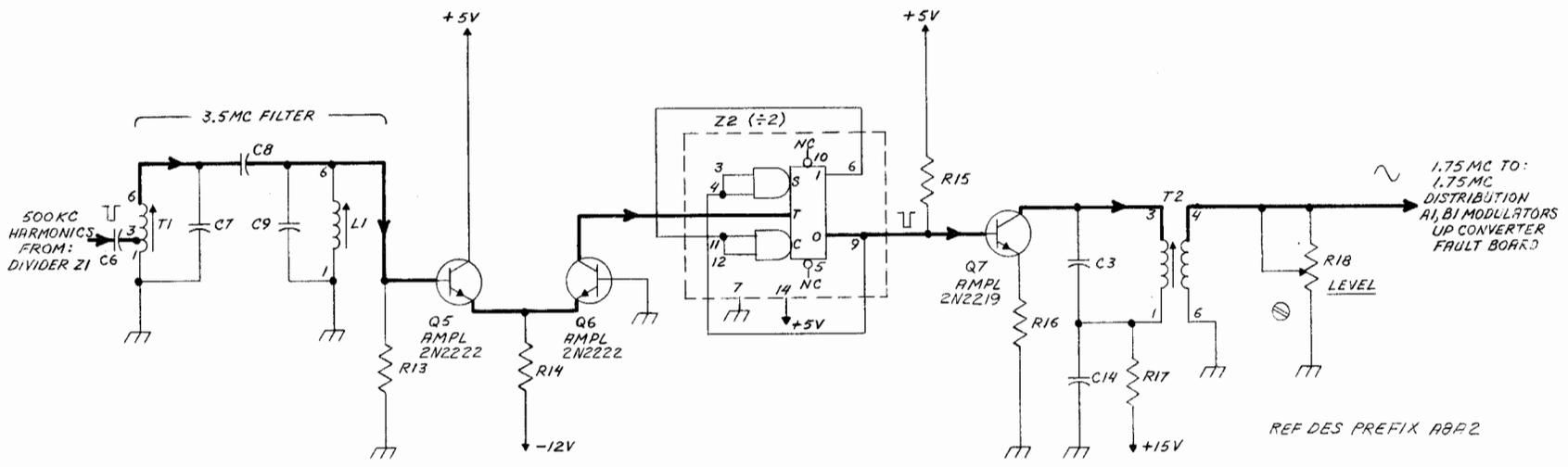
Figure 4-8. 1.75 Mc Frequency Divider, Simplified Schematic Diagram
