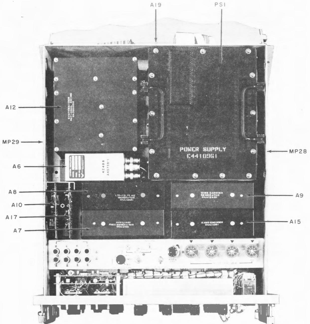
Figure 5-1. Modulator-Synthesizer MD-777/FRT, Top View Case Removed
