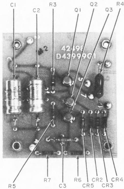
Figure 5-51. -18 Volt Regulator A1, Part of Power Supply PS1, Parts Location
