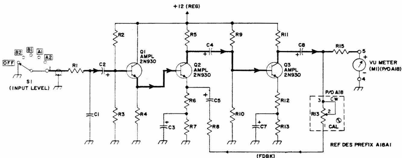
Figure 4-32. VU Meter Amplifier, Simplified Schematic Diagram
