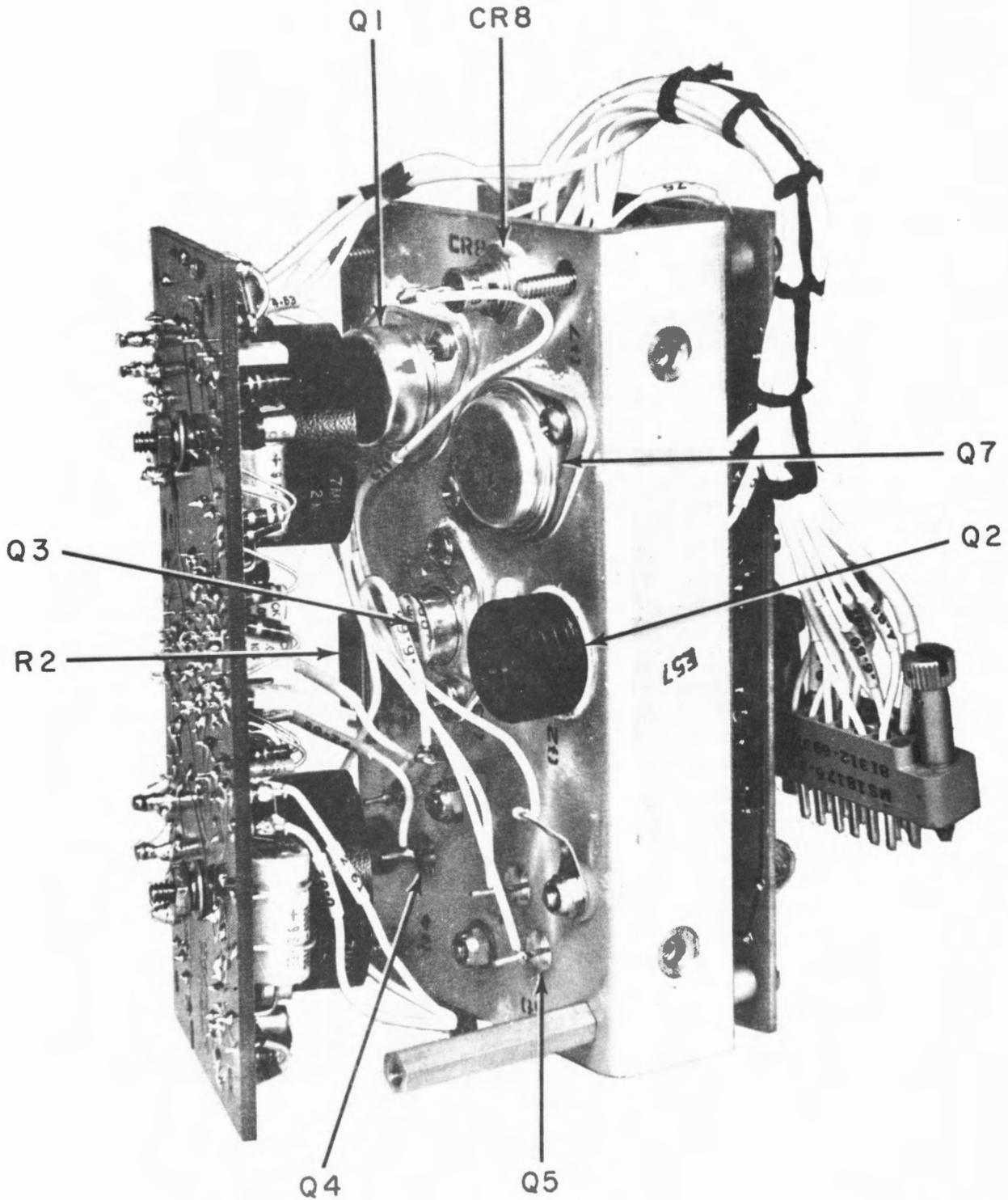
Figure 5-50B. Bracket Subassembly A2MP1,
