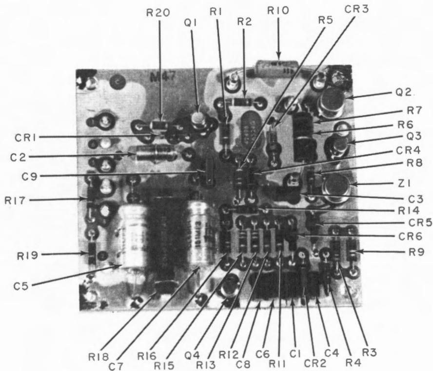
Figure 5-54. A3 Switching Regulator, Part of Power Supply PS1
