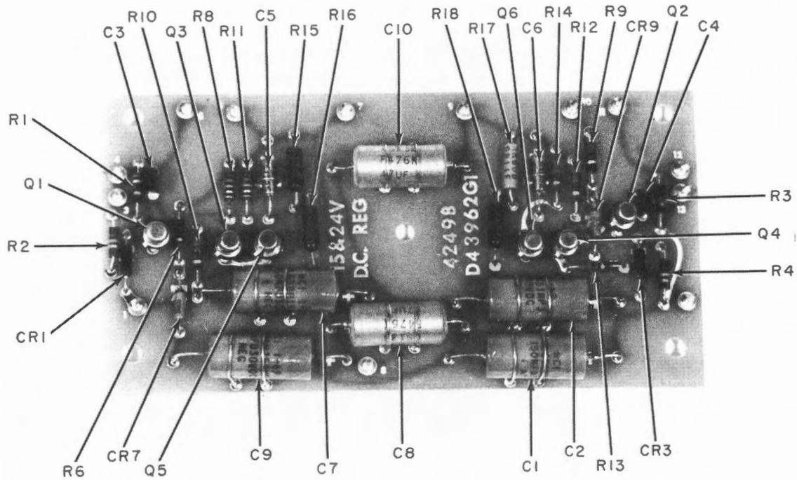
Figure 5-53. +15 and +24 Volt Regulator A2A2, Part of Power Supply PS1, Parts Location
