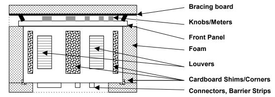
Bracing example: Top View – R-388/390x Style w/Rack Handles
