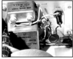
The main change you will notice when turning the radio on is that the antenna relay now does a slow "ka-chunk" – which means you've been successful!
