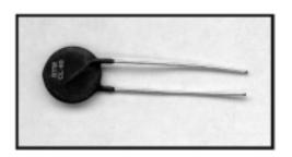
to handle current. At room temp it exhibits some resistance. As current passes through and it warms up, this resistance drops by a factor of a hundred or so. Keystone limiters are rated by current handling capability (1.1 to 16 amps) and cold resistance (0.7 to 120 ohms). Not all possible combinations of resistance and current are available, but my Mouser catalog lists about twenty to choose from. They cost a couple of bucks each, which is cheap insurance!
