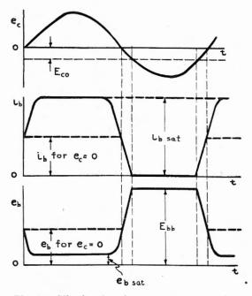
Fig. 11. Clipping by plate-current saturation.
