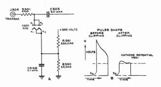
Indicator Limiter Stage-Circuit and Wave Shapes.
