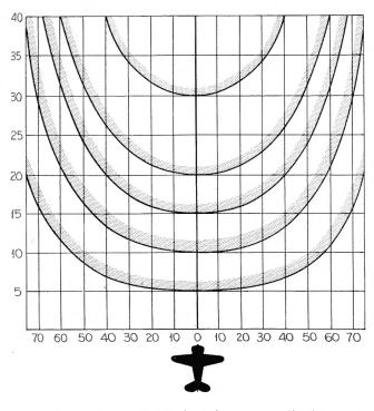
Figure 2. If an aircraft is flying perpendicular to an approximately straight coastline, the shore will appear as above. The closer the aircraft, the broader the indication will "fan out".
