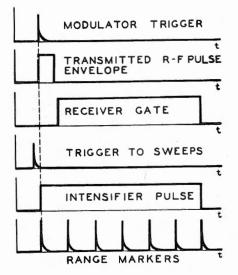
Fig. 2. Control pulses furnished by the timer of Fig. 1.
