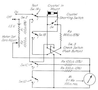
This schematic shows the wiring arrangement of the crystal checker described in this article
