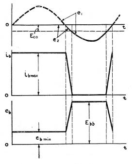
Fig. 10. Waveforms in clipper.
