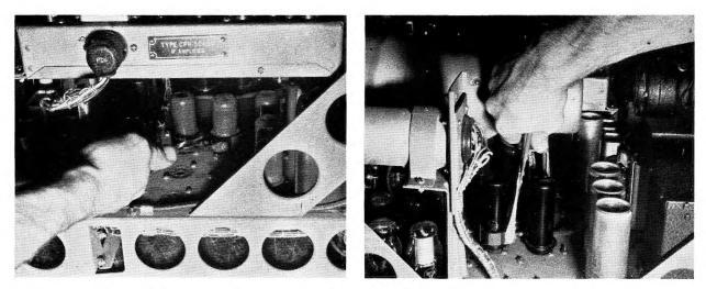
The above photos demonstrate how the vacuum tube extractor may be used in tight and awkward places.
