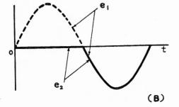
Fig. 5. Alternate diode clipper.
