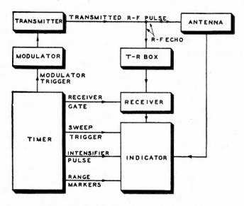
Fig. 1. Possible functions of a radar timer.
