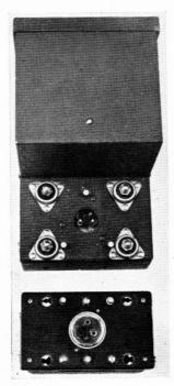
The Magnavox Company, Fort Wayne, Indiana, is now procuring improved dynamotor plugs assembled on a micabase insulation material known as Micelroy which will be used on all AM-40/AIC and all future RL-7 interphone amplifiers. Micelroy insulation has extremely low moisture absorption under the most adverse conditions and will not carbonize in the presence of heat.
