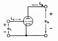
Fig. 6. Voltages and currents in amplifier-type tube.
