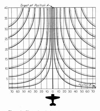
Figure 1. If an aircraft is flying <u>parallel</u> to an approximately straight coastline and its radar sights a target at position A, the target indication will move down the scope and veer off to the right as the plane approaches. When the aircraft is almost abeam of the target, the indication is at point B.
