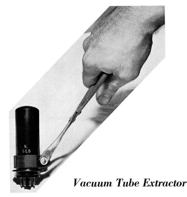
A versatile vacuum tube extractor for removing hot, broken and inaccessible glass and metal receiving type tubes was designed and built by A. E. D'Emidio, ART1c, of Blimp Headquarters Squadron ONE, Detachment TWELVE.
