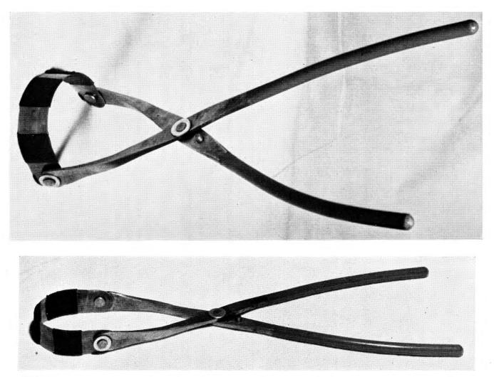
The two views above show how the band on the vacuum tube extractor is flexible so that it may be used in flat or or upright position.
