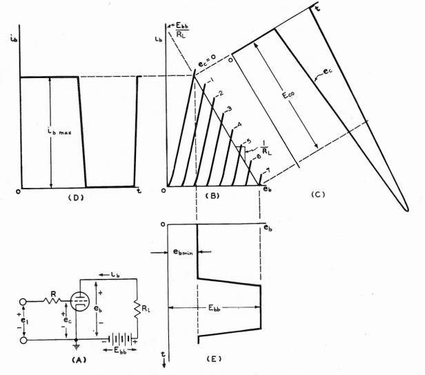
Fig. 9. Formation of a square wave by clipping a sine wave.
