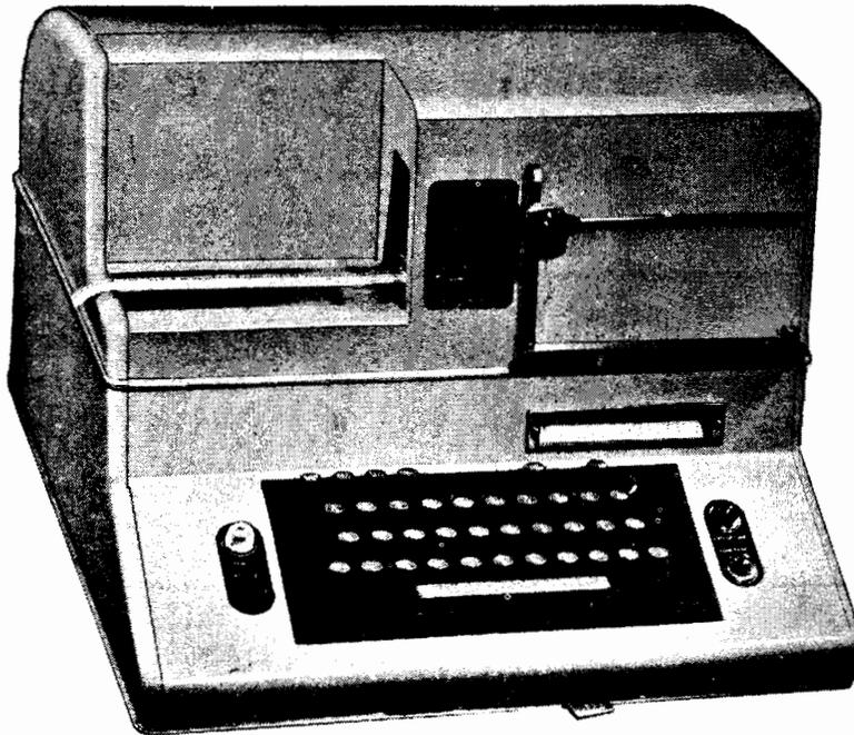
PERFORATOR-REPERFORATOR, TELETYPEWRITER TT-253A/UG
