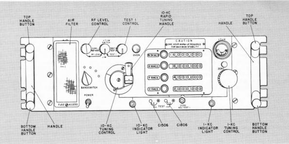
Figure 4. Front panel of synthesizer.
