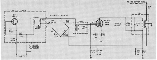
Figure 9. Meacham oscillator schematic.
