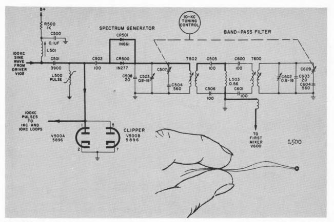
Figure 7 (above). Pulse generator.
