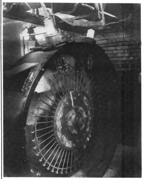
OLD NAA – CLOSE UP OF THE SYNCHRONOUS ROTARY GAP OF THE  $100\ \mbox{KW}$  SPARK TRANSMITTER FURNISHED THE NAVY BY
