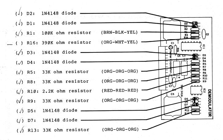
Install the following parts on the DEMODULATOR board.
