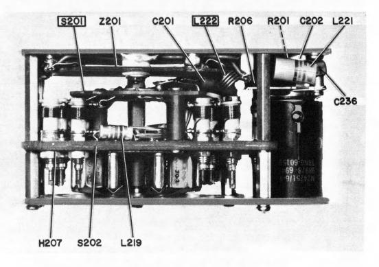
Figure 5-38. Frequency Multiplier-Oscillator, Master Oscillator, Right Side
