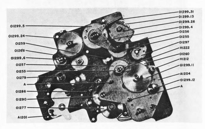
Figure 5-71. Frequency Selector, Front View of Rear Plate (AN/URC-9, -9Y, -9AY)
