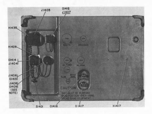
Figure 5-61. Receiver-Transmitter Case CY-2959/URC-9, Rear View
