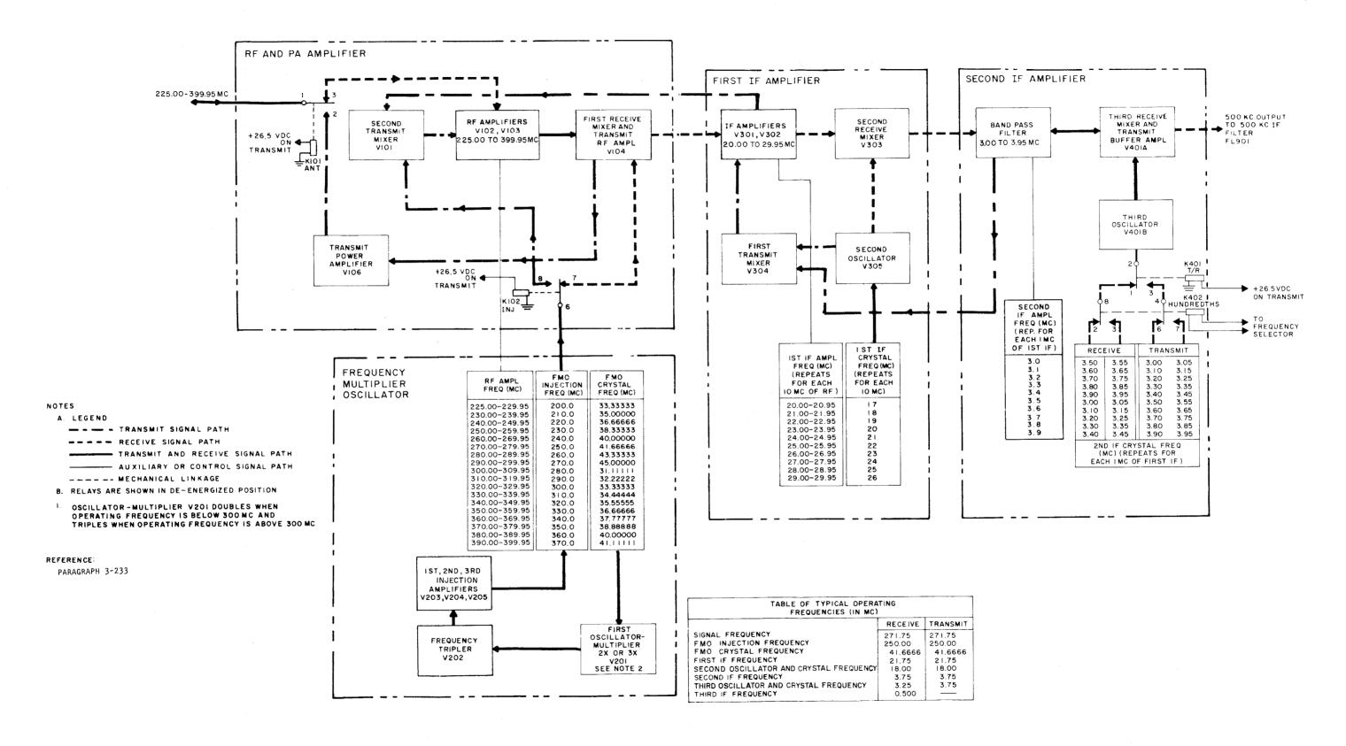
Figure 3-13. Radio Set AN/URC-9A Frequency Conversion System, Functional Block Diagram
