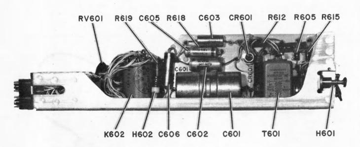
Figure 5-53. Relay-Filter Assembly, Left Side
