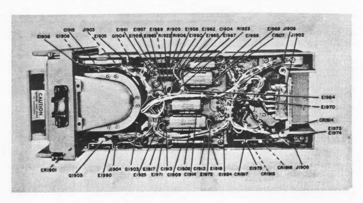
Figure 5-93. Power Supply PP-4706A/URC-9Y, Bottom View
