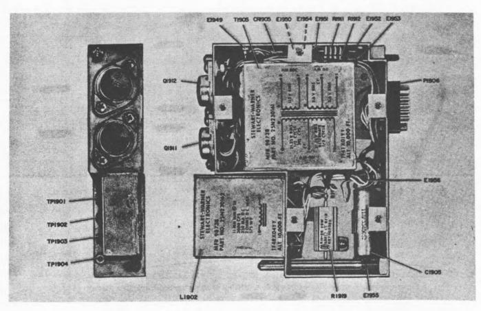
Figure 5-97. Power Supply PP-4706A/URC-9Y, Power Supply Module (A1904)
