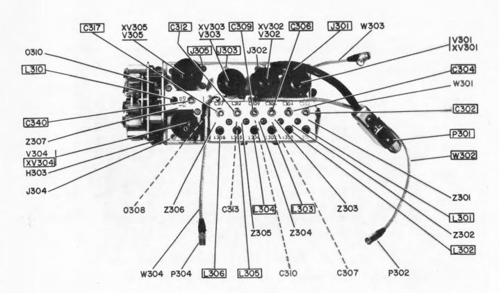
Figure 5-39. First IF Amplifier, Top View
