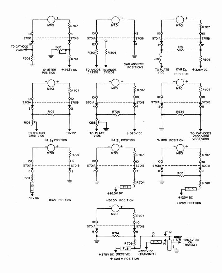
Figure 3-10. Metering Circuits, Simplified Schematic Diagram
