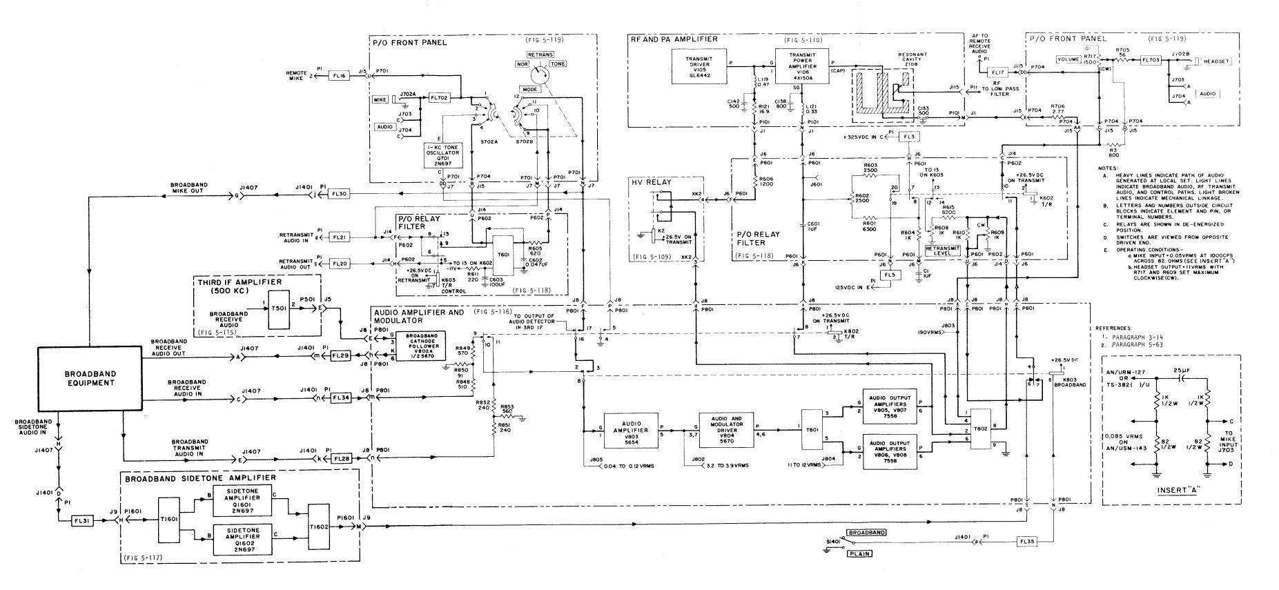
Figure 5-3. Radio Set AN/URC-9(), Transmit Audio Function and Broadband Mode Troubleshooting Block Diagram
