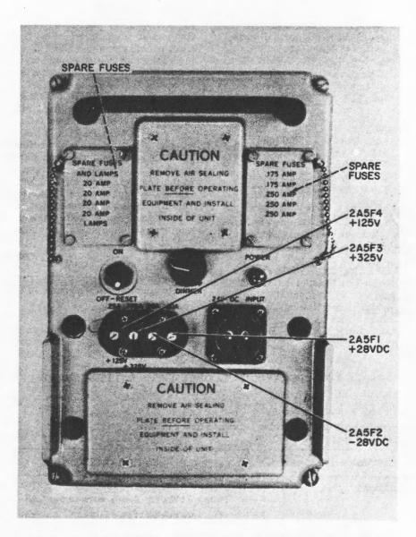
Figure 2-7. Radio Set AN/URC-9Y, Fuse Location
