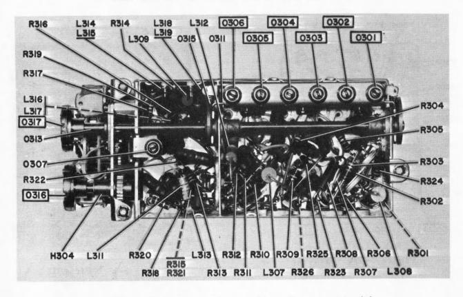
Figure 5-40. First IF Amplifier, Bottom View (A)
