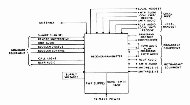
Figure 3-1. Radio Set AN/URC-9(), Basic Block Diagram
