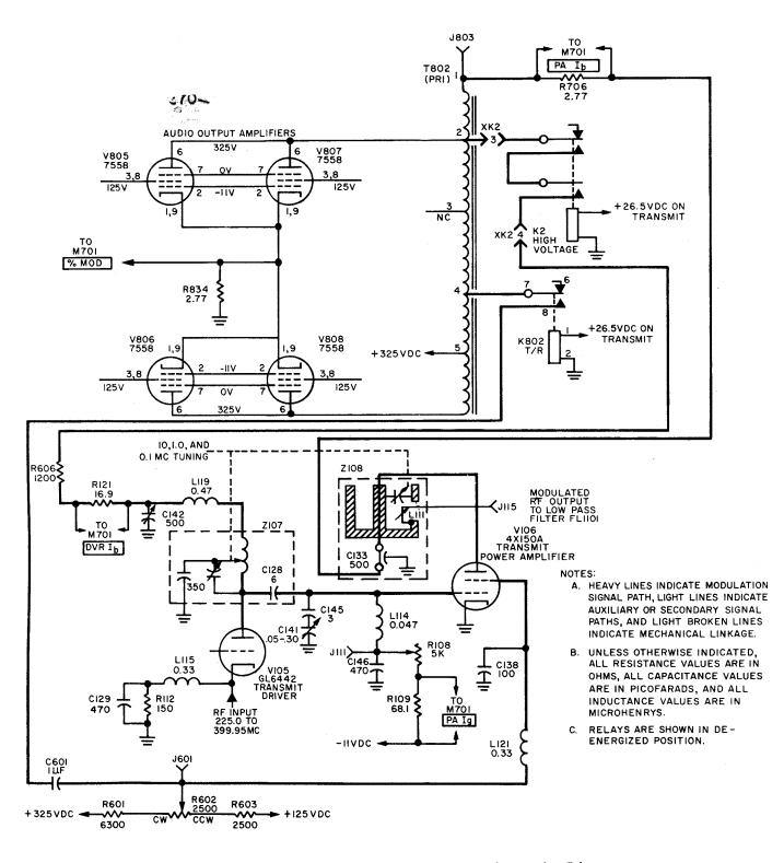
Figure 3-4. Modulation Circuits, Schematic Diagram
