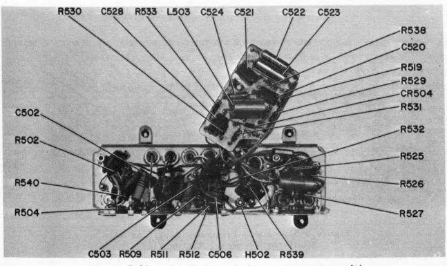
Figure 5-49. Third IF Amplifier, Bottom View (B)
