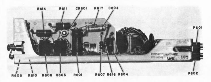
Figure 5-54. Relay-Filter Assembly, Right Side
