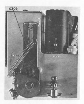
Figure 5-43. First IF Amplifier, Synchronization
