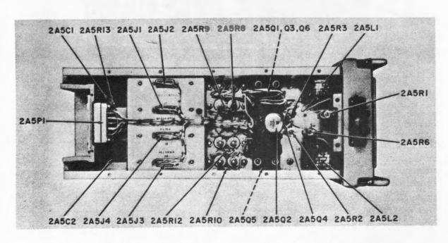
Figure 5-86. Power Supply PP-4706/URC-9Y, Bottom View
