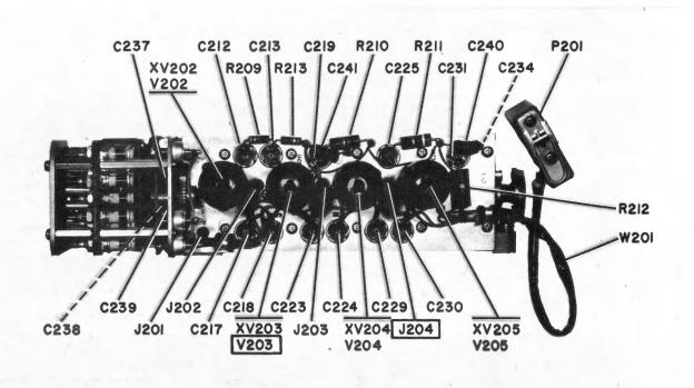
Figure 5-33. Frequency Multiplier-Oscillator,
