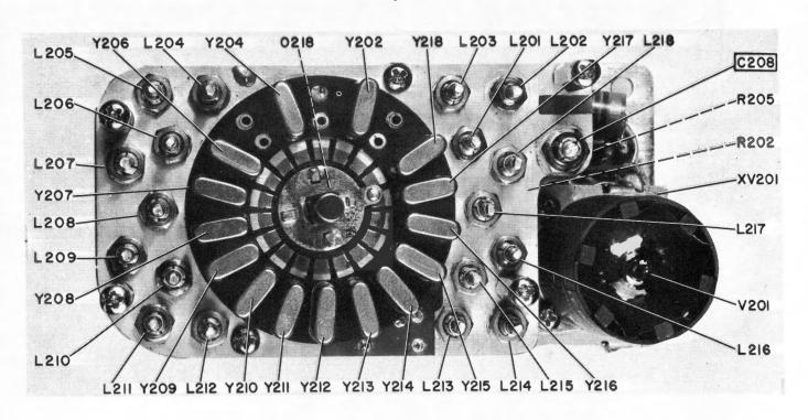
Figure 5-34. Frequency Multiplier-Oscillator, Master Oscillator (V201), Rear View
