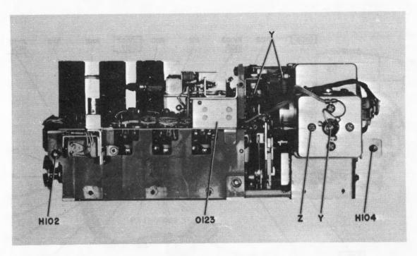
Figure 5-20. RF and PA Amplifier Assembly, Right Side, Disassembly Points
