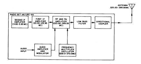
NOTE: FREQUENCIES SHOWN ARE FOR AN/URC-9A. FREQUENCIES FOR AN/URC-9, 9Y, AND 9AY ARE THE SAME LESS THE HUNDREDTHS POSITION.
