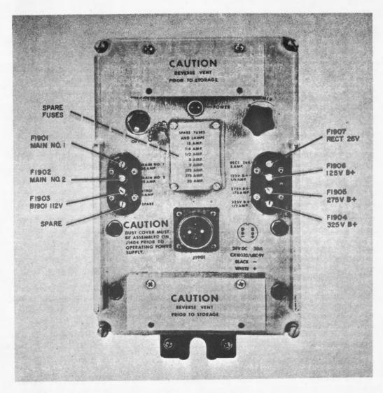
Figure 2-8. Radio Set AN/URC-9AY, Fuse Location
