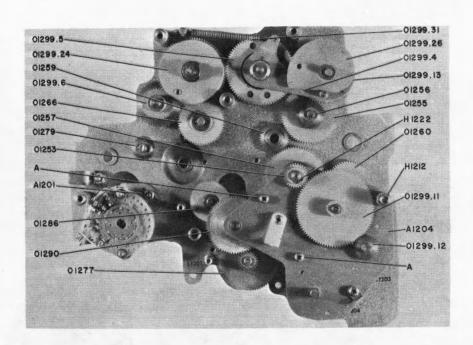
Figure 5-72. Frequency Selector, Front View of Rear Plate (AN/URC-9A)
