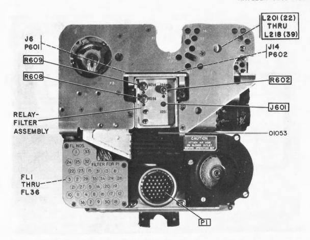
Figure 5-15. Receiver Transmitter RT-581()/URC-9. Rear View
