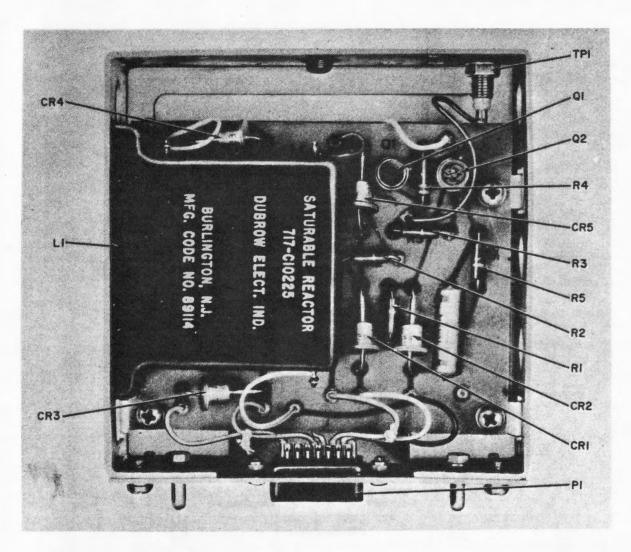
Figure 5-88. Power Supply PP-4706/URC-9Y, Frequency Control Module 2A5A2
