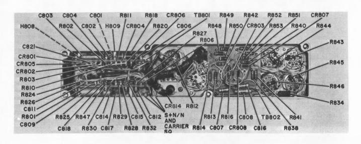
Figure 5-51. Audio Frequency Amplifier and Modulator Assembly, Bottom View
