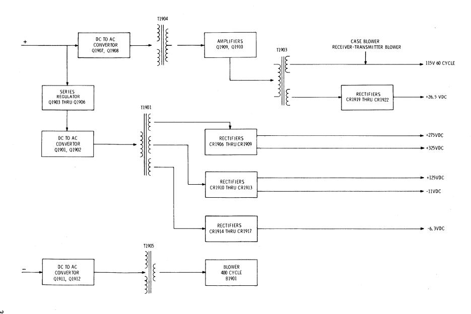
Figure 3-12. Power Supply PP-4706A/URC-9Y, Block Diagram
