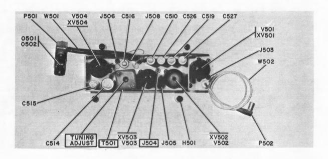
Figure 5-47. Third IF Amplifier, Top View
