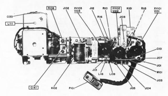
Figure 5-22. RF and PA Amplifier Assembly, Top View
