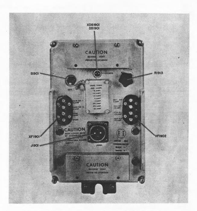
Figure 5-91. Power Supply PP-4706A/URC-9Y, Front View
