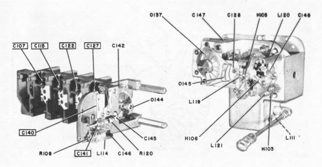
Figure 5-27. RF and PA Amplifier Assembly, Power Amplifier Stage Removed
