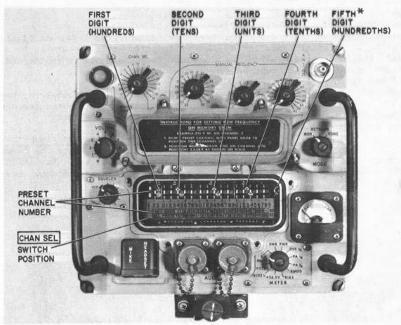
\*Only on AN/URC-9A Figure 2-5. Radio Set AN/URC-9, Preset Channel Memory Drum
