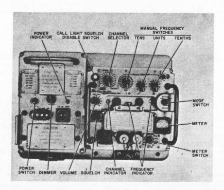
Figure 2-2. Radio Set AN/URC-9Y, Controls and Indicators
