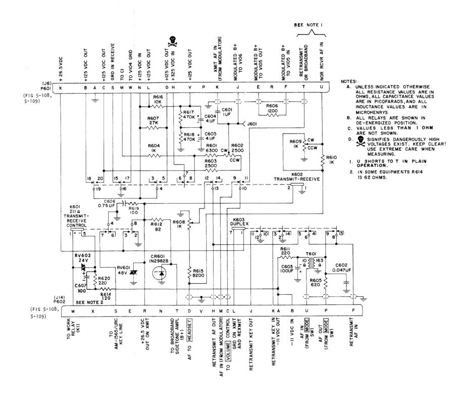
Figure 5-118. Relay-Filter Assembly, Schematic Diagram
