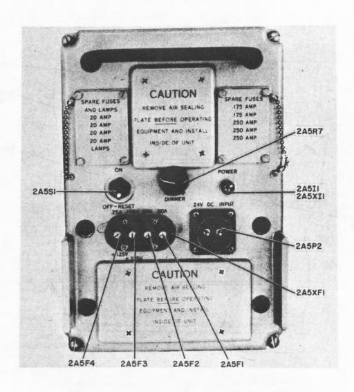
Figure 5-84. Power Supply PP-4706/URC-9Y, Front View
