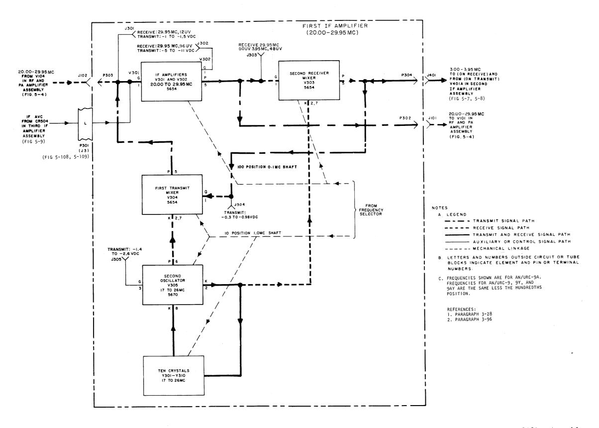
Figure 5-6. First IF Amplifier Assembly, Servicing Block Diagram
