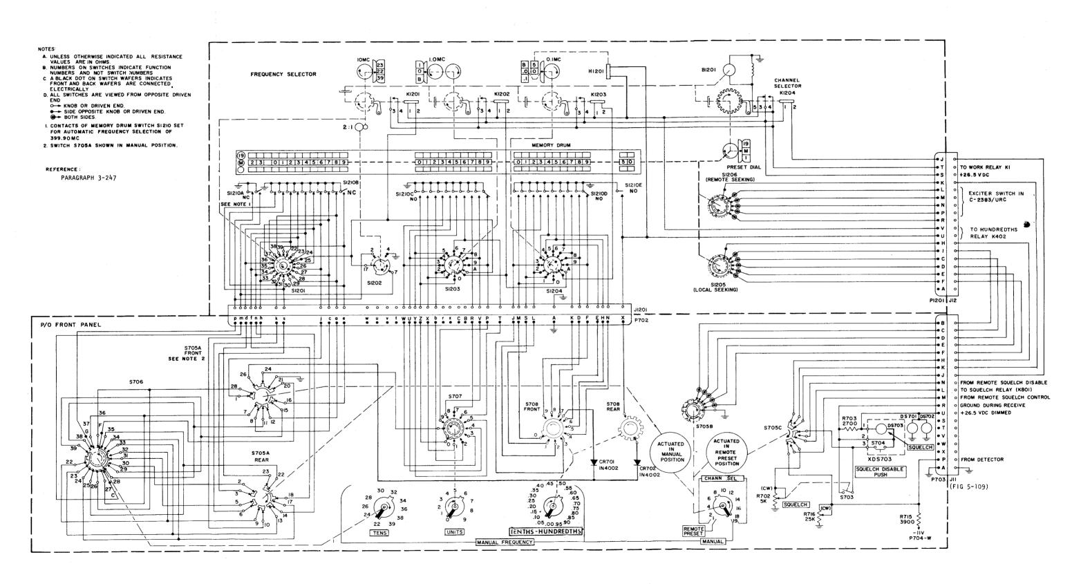
Figure 5-121. Part of Front Panel Assembly and Frequency Selector Assembly, Schematic Diagram (AN/URC-9A)
