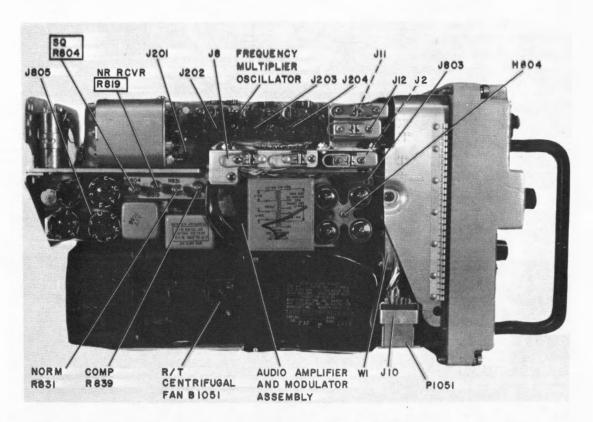
Figure 5-13. Receiver Transmitter RT-581()/URC-9, Left Side
