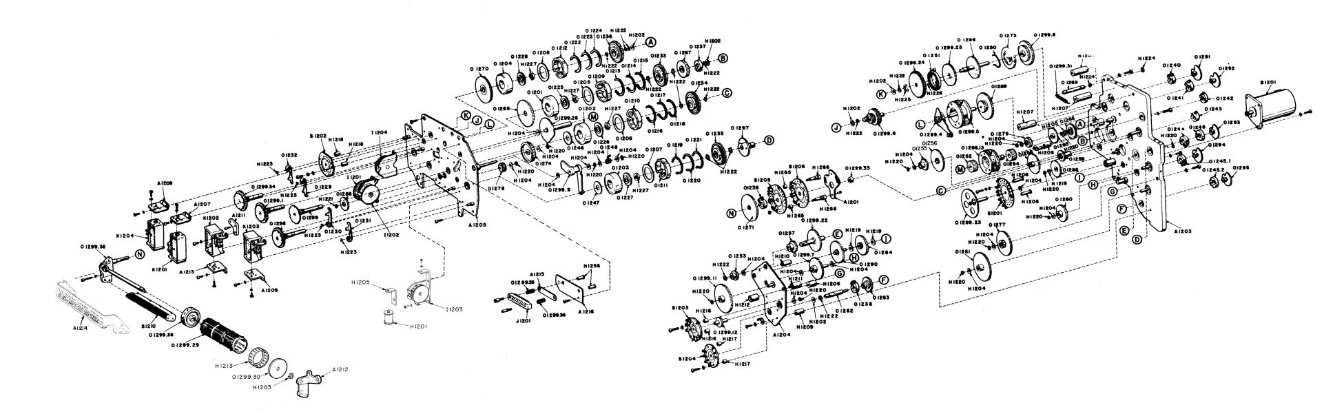
Figure 5-79. Frequency Selector, Exploded View (AN/URC-9A)
