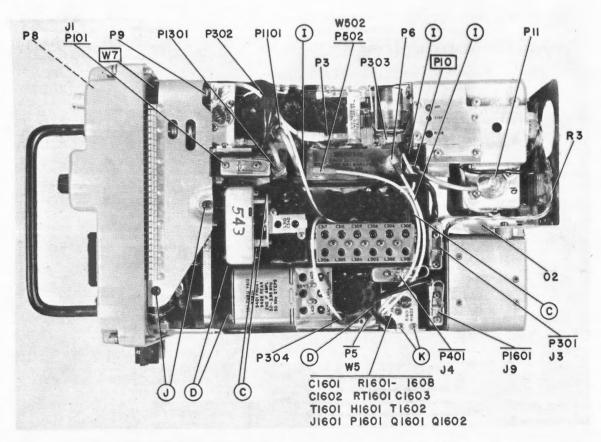
Figure 5-17. Receiver Transmitter RT-581()/URC-9, Right Side, Subassembly Removal
