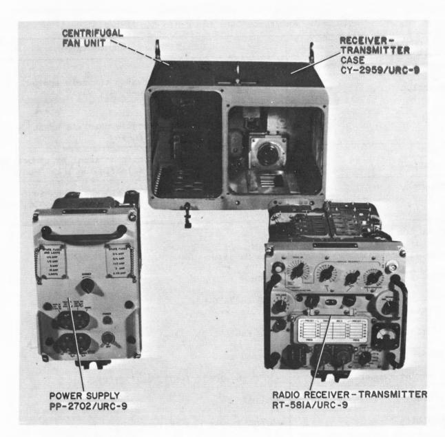
Figure 1-2. Units of Radio Set AN/URC-9(), Typical
