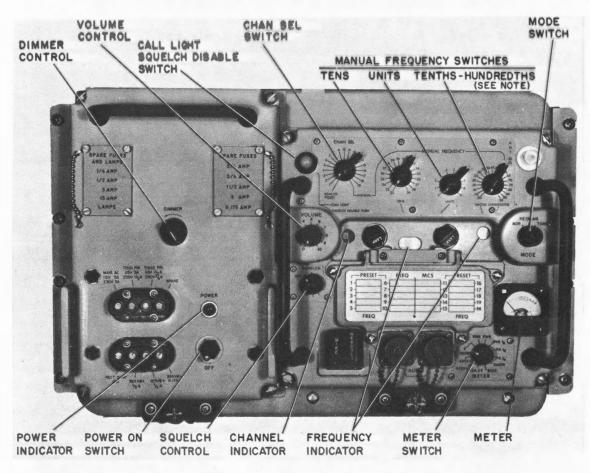
NOTE: Graduated in .1 MHz increments on AN/URC-9
