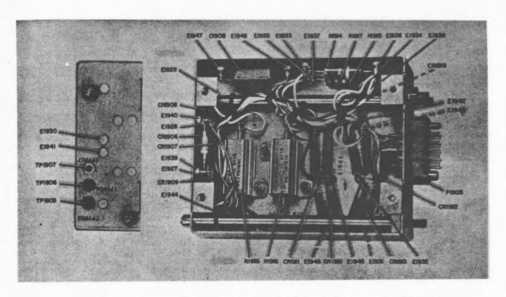
Figure 5-96. Power Supply PP-4706A/URC-9Y, Filter Bias Module (A1903)
