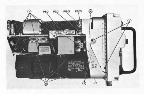
Figure 5-18. Receiver Transmitter RT-581()/URC-9, Left Side, Subassembly Removal
