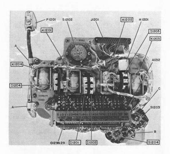
Figure 5-68. Frequency Selector, Front View (AN/URC-9A)
