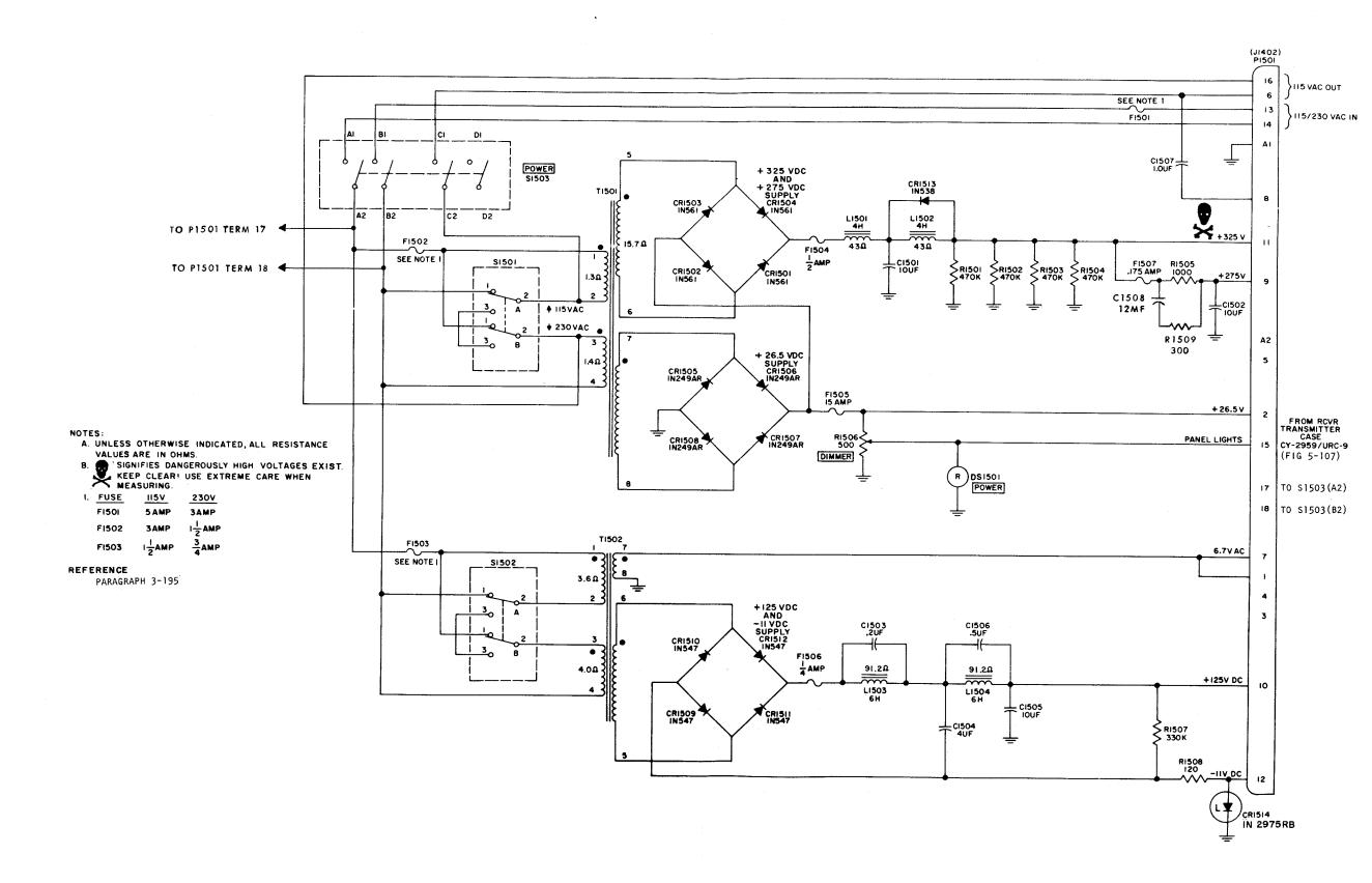
Figure 5-106. Power Supply PP-2702/URC-9, Schematic Diagram
