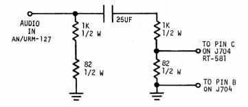
This Impedence Matching Network is used to match the output impedence of the URM-127 to the input of the RT-581. It is used in the RT-581 Modulator checks.
