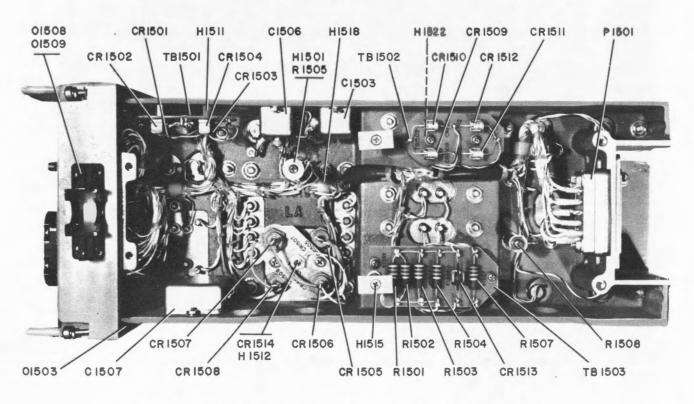
Figure 5-82. Power Supply PP-2702/URC-9, Bottom View
