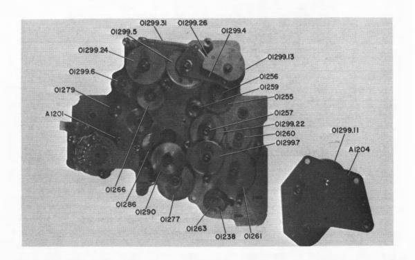
Figure 5-74. Frequency Selector, Front View of Rear Plate, Small Gear Plate Removed (AN/URC-9A)
