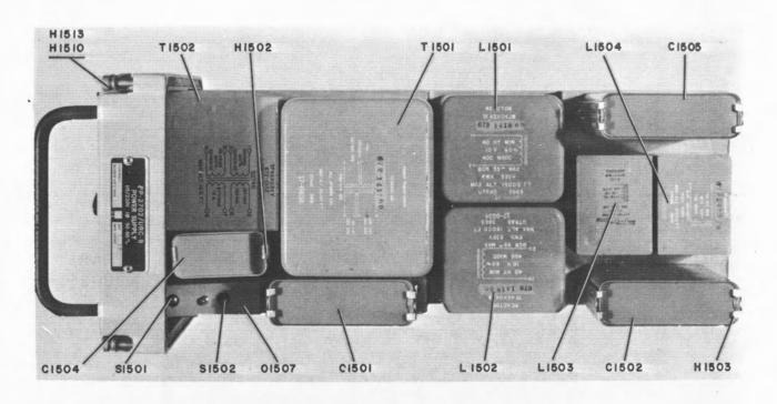
Figure 5-81. Power Supply PP-2702/URC-9, Top View
