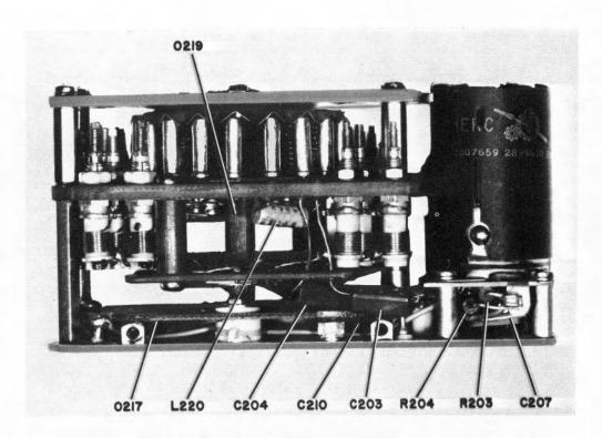
Figure 5-37. Frequency Multiplier-Oscillator, Master Oscillator, Left Side
