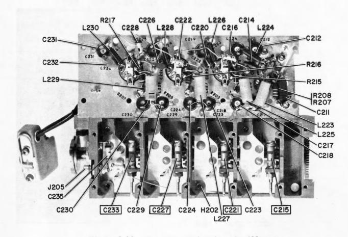
Figure 5-36. Frequency Multiplier-Oscillator, Chassis, Bottom View
