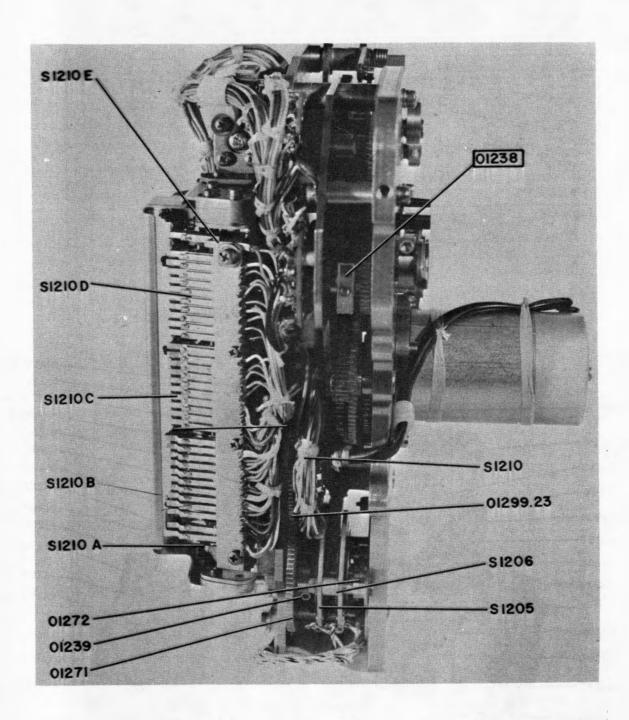
Figure 5-69. Frequency Selector, Bottom View
