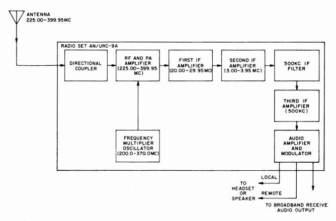
NOTE: Frequencies shown are for AN/URC-9A. Frequencies for AN/URC-9, 9Y, and 9AY are the same less the hundredths position.
