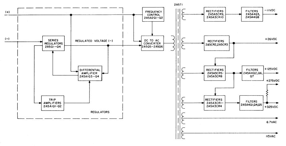
Figure 3-11. Power Supply PP-4706/URC-9Y, Block Diagram
