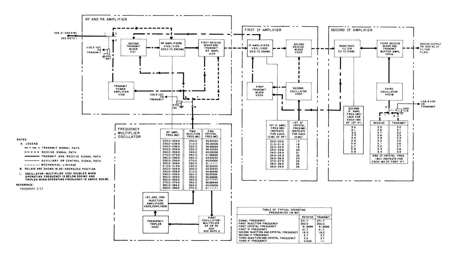
Figure 3-14. Radio Set AN/URC-9, -9Y, -9AY, Frequency Conversion System, Functional Block Diagram
