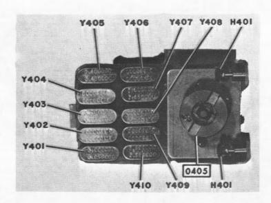
Figure 5-46. Second IF Amplifier, Front View
