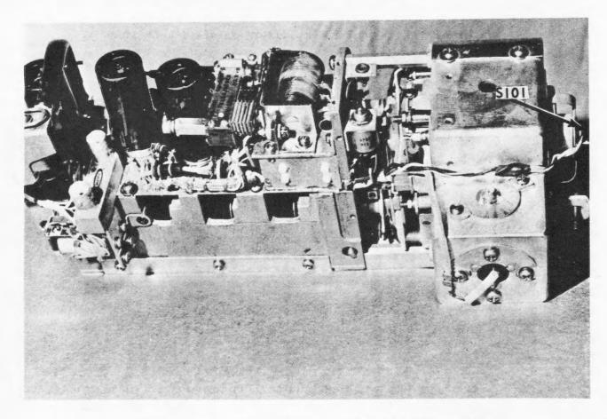
Figure 5-24. RF and PA Amplifier Assembly, Side View Showing Thermal Sensor
