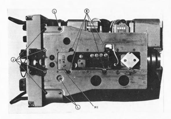
Figure 5-19. Receiver Transmitter RT-581()/URC-9, Bottom View, Subassembly Removal
