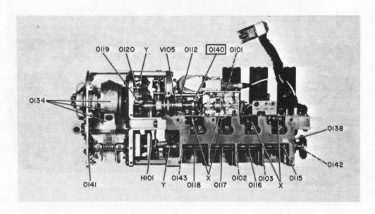
Figure 5-21. RF and PA Amplifier Assembly, Left Side, Disassembly Points
