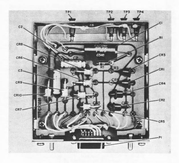
Figure 5-89. Power Supply PP-4706/URC-9Y, Rectifier Module 2A5A3
