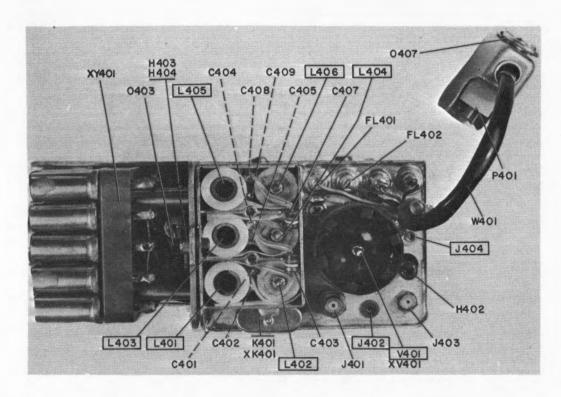
Figure 5-44. Second IF Amplifier, Top View
