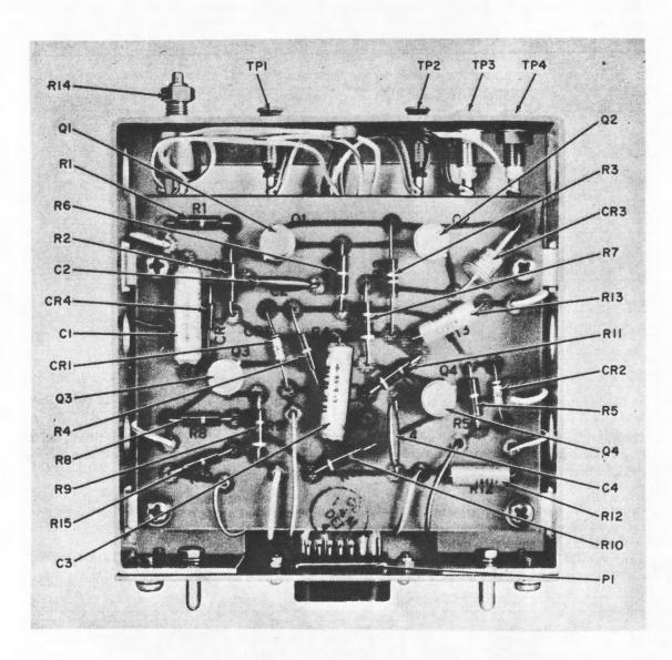
Figure 5-87. Power Supply PP-4706/URC-9Y, Regulator Module 2A5A1
