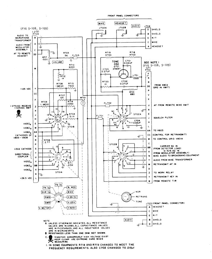
Figure 5-119. Part of Front Panel Assembly, Schematic Diagram (AN/URC-9())
