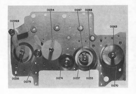
Figure 5-75. Frequency Selector, Rear View of Front Plate
