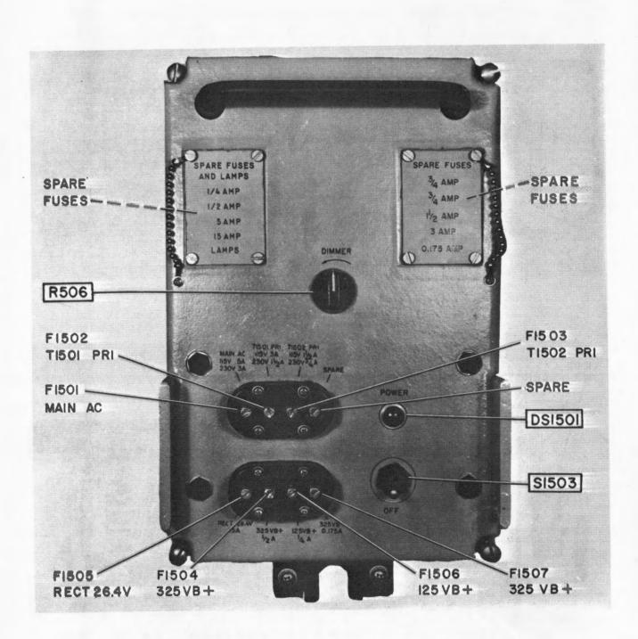
Figure 5-80. Power Supply PP-2702/URC-9, Front View
