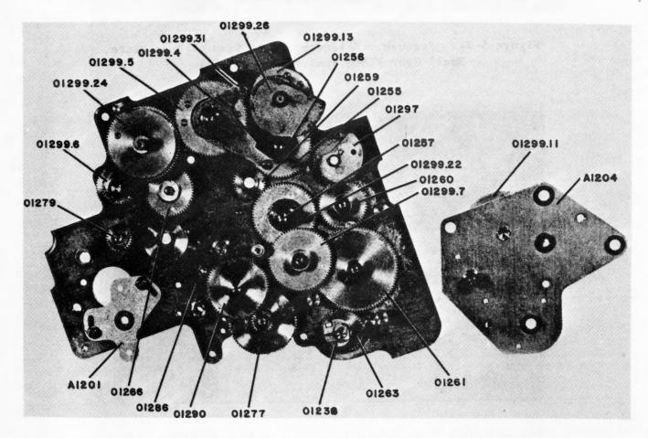
Figure 5-73. Frequency Selector, Front View of Rear Plate, Small Gear Plate Removed (AN/URC-9, -9Y, -9AY)
