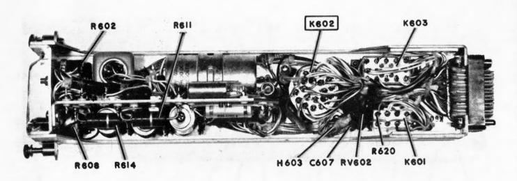
Figure 5-52. Relay-Filter Assembly, Top View
