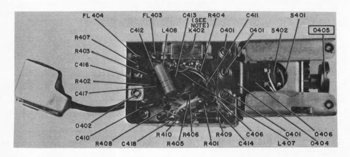
Figure 5-45. Second IF Amplifier, Bottom View
