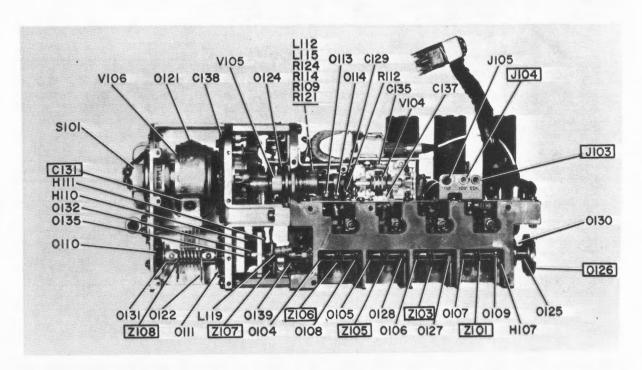
Figure 5-25. RF and PA Amplifier Assembly, Left Side
