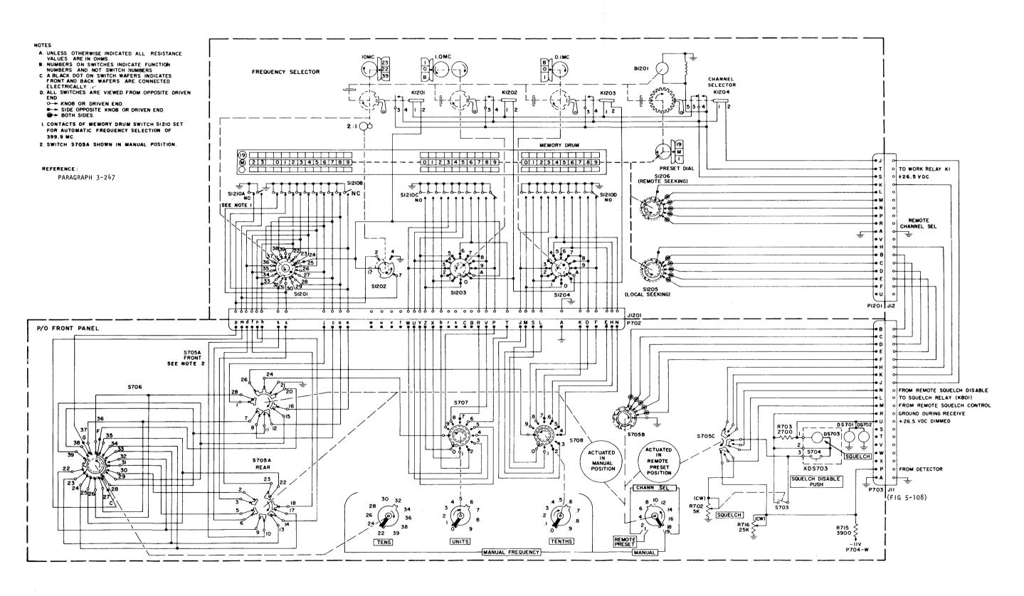
Figure 5-120. Part of Front Panel Assembly and Frequency Selector Assembly, Schematic Diagram (AN/URC-9, -9Y, -9AY)
