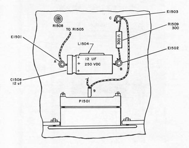
Figure 5-83. Power Supply PP2702/URC-9, R1509 and C1508 Location
