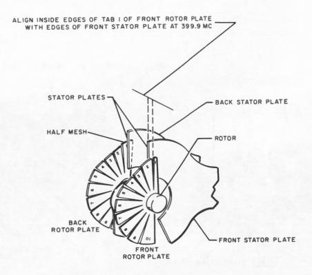
FMO, RF AND PA ASSEMBLIES TUNER CAPACITOR PLATES (Z202, Z204, Z206, Z208, Z101, Z103, Z105, AND Z106)
