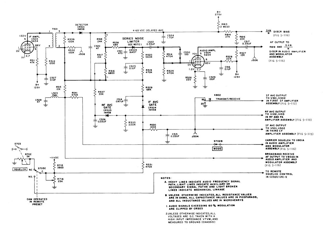
Figure 3-8. Radio Set AN/URC-9(), Detector, Noise Limiter, and AVC Circuits, Simplified Schematic Diagram
