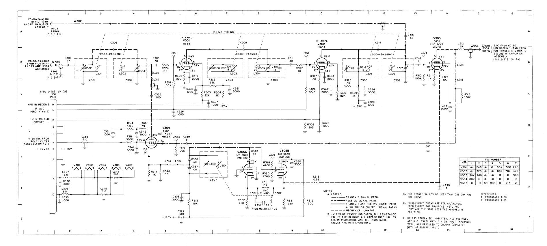
Figure 5-112. First IF Amplifier Assembly, Schematic Diagram
