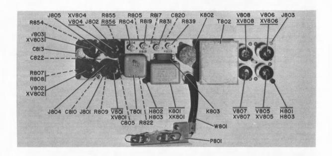
Figure 5-50. Audio Frequency Amplifier and Modulator Assembly, Top View
