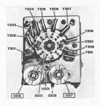
Figure 5-42. First IF Amplifier, Front View
