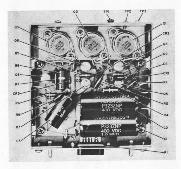
Figure 5-90. Power Supply PP-4706/URC-9Y, Filter Module 2A5A4
