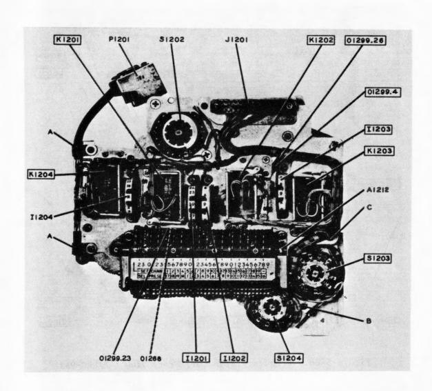
Figure 5-67. Frequency Selector, Front View (AN/URC-9, -9Y, -9AY)
