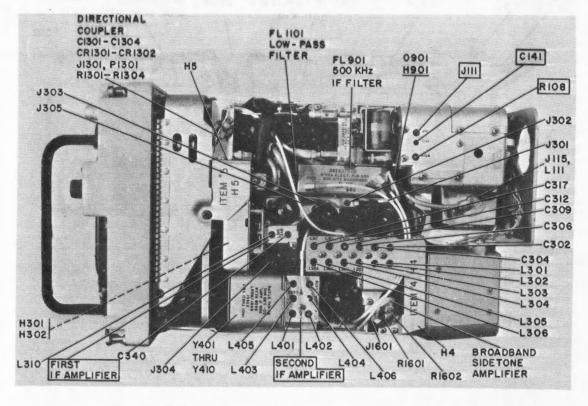
Figure 5-12. Receiver Transmitter RT-581()/URC-9, Right Side
