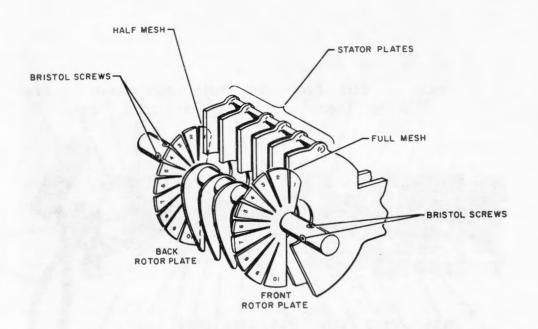
Figure 5-31. RF and PA Amplifier Assembly, Tuner Z108
