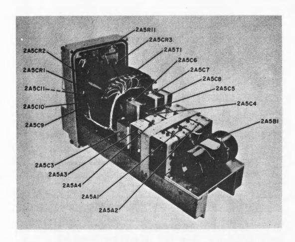
Figure 5-85. Power Supply PP-4706/URC-9Y, Top View
