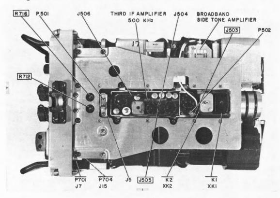
Figure 5-14. Receiver Transmitter RT-581()/URC-9, Bottom View
