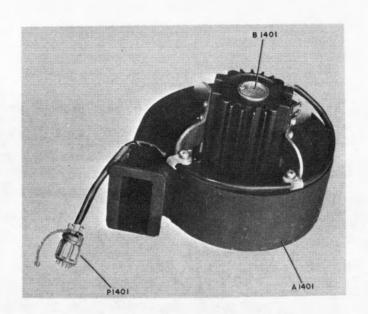
Figure 5-62. Receiver-Transmitter Case CY-2959/URC-9, Centrifugal Fan
