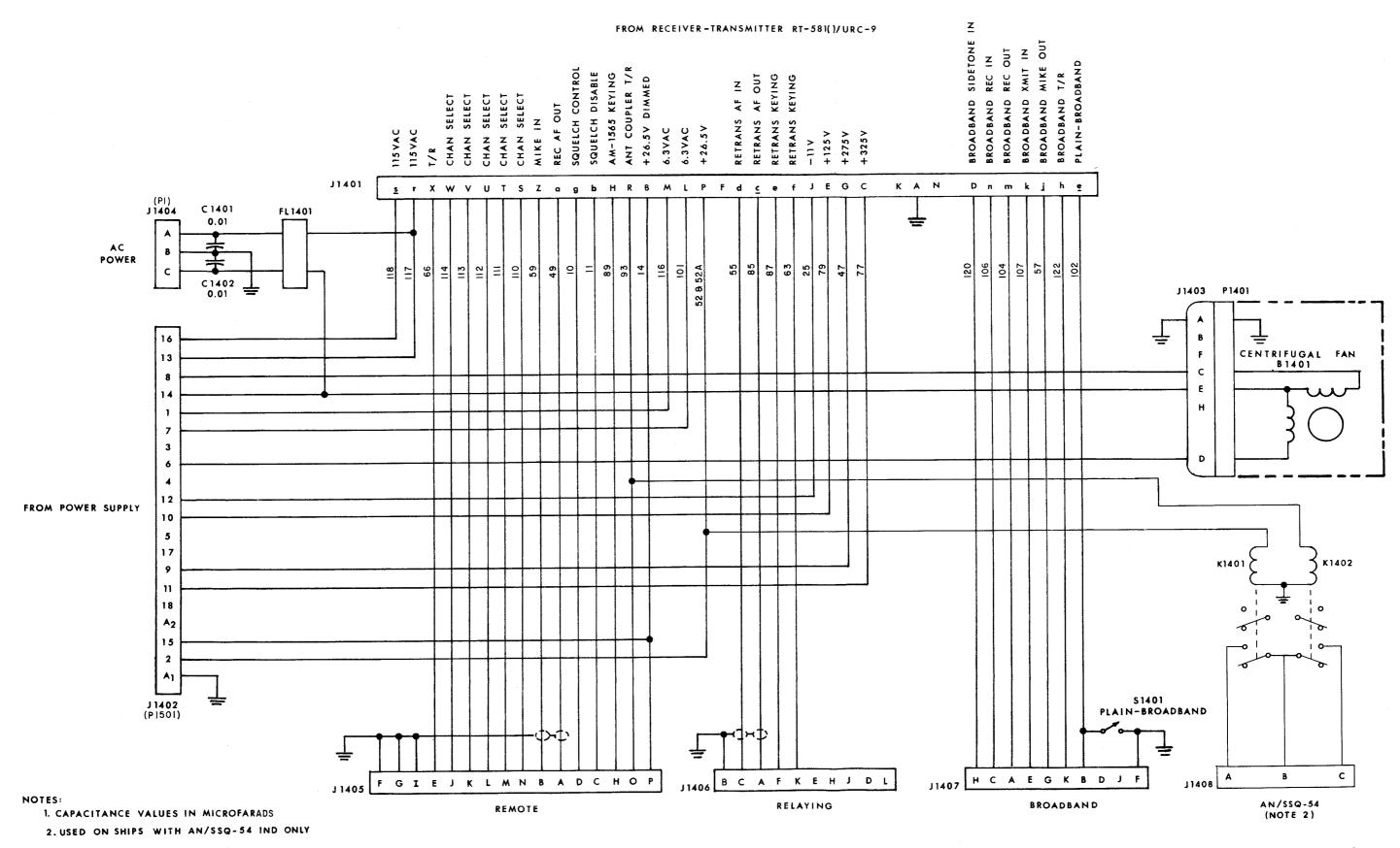
Figure 5-107. Receiver-Transmitter Case CY-2959/URC-9, Schematic Diagram
