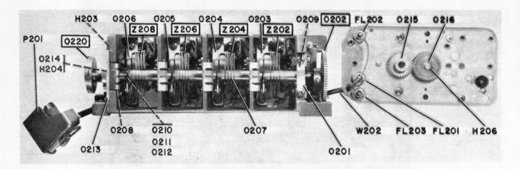
Figure 5-35. Frequency Multiplier-Oscillator, Bottom View, Master Oscillator Removed
