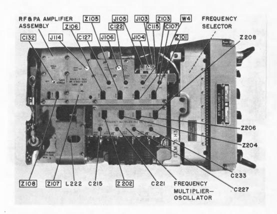
Figure 5-11. Receiver Transmitter RT-581()/URC-9, Top View
