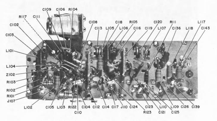
Figure 5-26. RF and PA Amplifier Assembly, Bottom View
