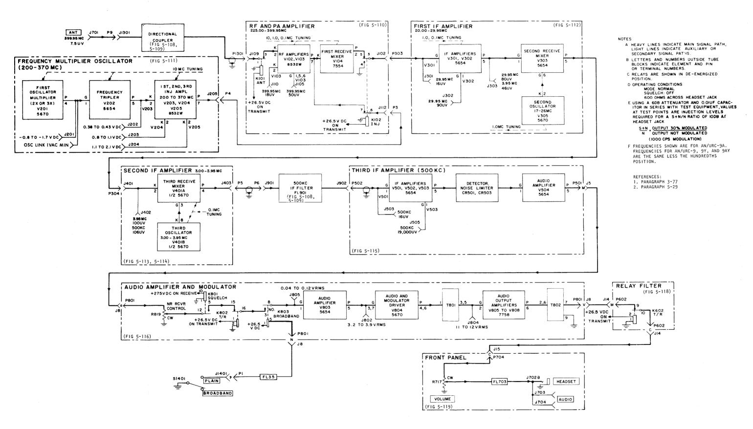
Figure 5-1. Radio Set AN/URC-9(), Receive Function Troubleshooting Block Diagram
