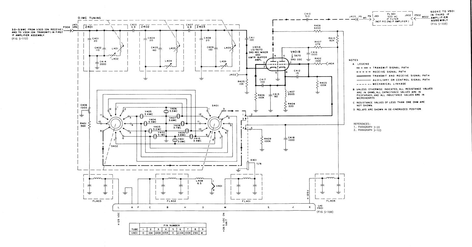
Figure 5-113. Second IF Amplifier Assembly, Schematic Diagram (AN/URC-9, -9Y, -9AY) 5-187/(5-188 blank)
