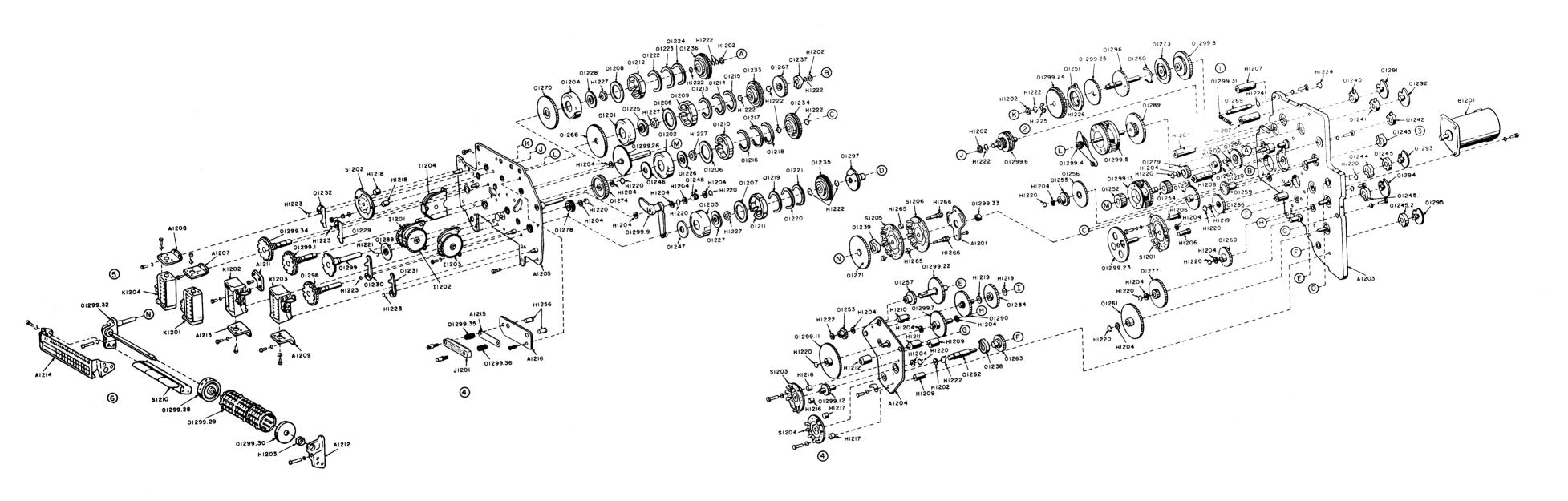
Figure 5-78. Frequency Selector, Exploded View (AN/URC-9, -9Y, -9AY)
