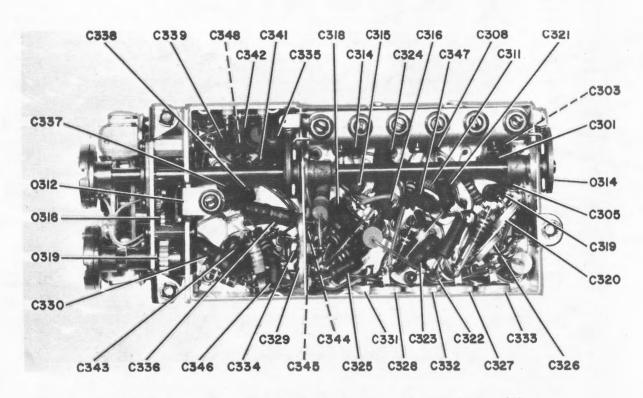
Figure 5-41. First IF Amplifier, Bottom View (B)
