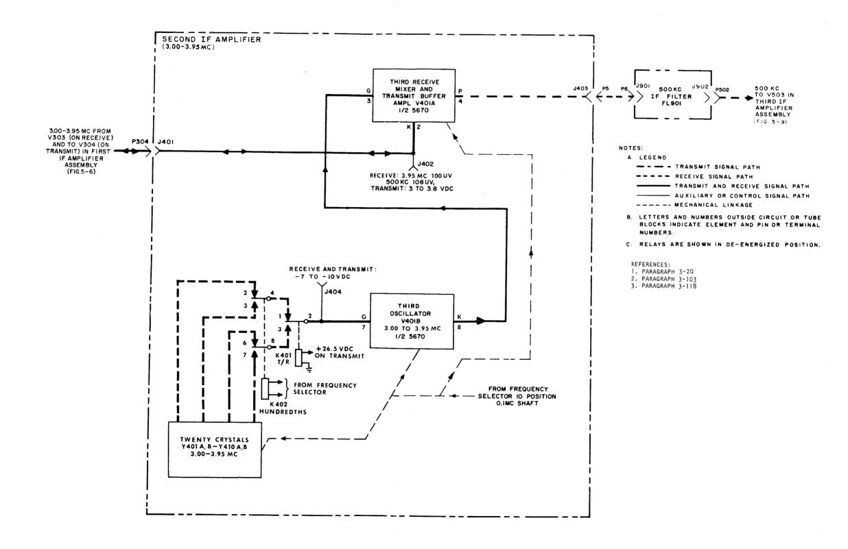
Figure 5-8. Second IF Amplifier Assembly, Servicing Block Diagram (AN/URC-9A)
