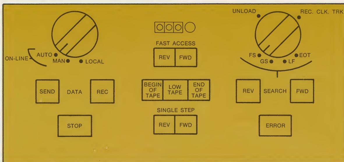
This is the standard control panel found on stand alone terminal and those compatible with model 33, model 35 and model 37 Teletype equipment.
