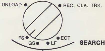
You can locate the exact beginning of a block of data on the magnetic tape by using the search controls. The 4210 magnetic tape data terminal recognizes four control characters recorded in data format for this purpose. These are ASCII control codes for:
