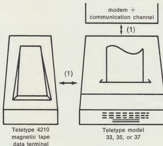
This Stand Alone configuration provides a common, on-line send-receive terminal for location with a number of data preparation terminals.
