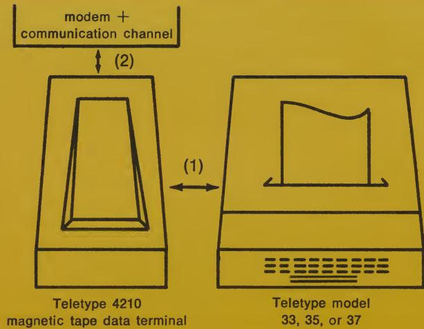
This configuration will send and receive at 1200 baud, 120 char/sec and provide immediate page copy.
