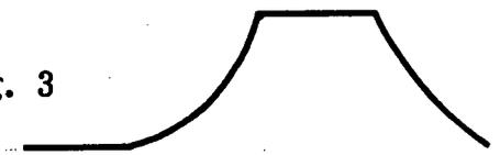
The impulse in Figure 3 is more likely to be found at the receiving printer than the one impressed at the transmitter, (Figure 1). The impulse seen in Figure 3, as applied to the selector magnets of the printer, will be used to illustrate Bias Distortion. It will be noted that this waveshape builds up to its 500 ma level gradually.
