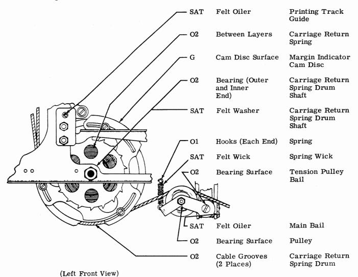
2.31 Spacing Drum Feed Mechanism
