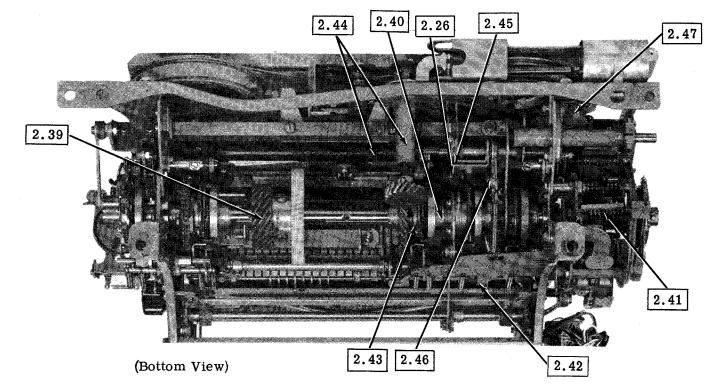
2.39 Main Shaft (Clutches, Gears, etc)
