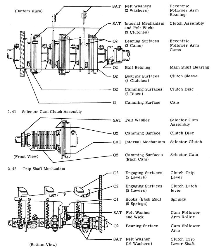
2.40 Main Shaft (Clutches, Gears, etc) (continued)
