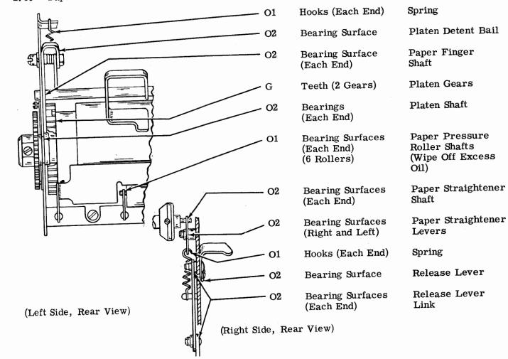
2.09 Paper Feed Mechanism (Friction Feed)
