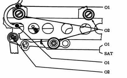
Bearing Surface Typebox Latch Toggle Bearings Typebox Carriage Rollers (3 Rollers) Hook (Each End) Spring Felt Wick Spring Bearing Surface Typebox Latch Bearing Surface Typebox Carriage Link
