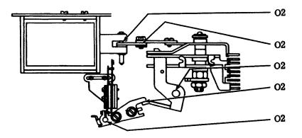
Pivot PointExtension LinkPivot PointBlocking BailBlocking SurfaceBlocking Bail<br/>ExtensionPivot PointTrip Arm
