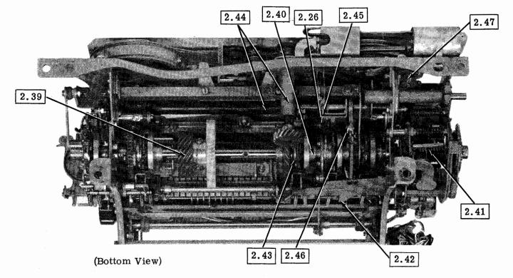
2.39 Main Shaft (Clutches, Gears, etc)
