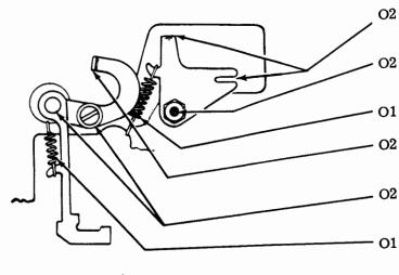
**Engaging Surfaces** Automatic Carriage (2 Places) Return Bellcrank Bearing Surface Automatic Carriage Return Bellcrank Hooks (Each End) Spring Engaging Surface Spacing Drum Feed Pawl Release Link Bearing Surfaces Spacing Drum Feed Pawl Release Link (2 Places) Hooks (Each End) Spring
