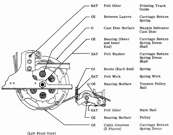
2.31 Spacing Drum Feed Mechanism
