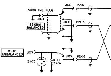
FIELD CHANGE NO.5(EIB 664) ANTENNA INPUT MODIFIED ON SHIPBOARD INSTALLATIONS -USE JIO3 AS ANTENNA INPUT JACK. REVERSE CABLES TO JIO5 AND JIO6
