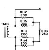
FIELD CHANGE NO. 2 CONVERSION TO 450 OHM SHUNT LOAD
