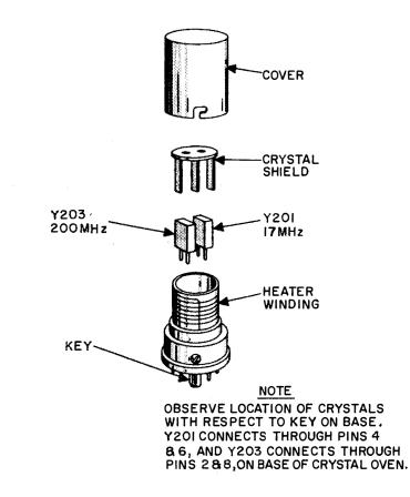
Figure 6-11. Location of Crystals Y201 and Y202
