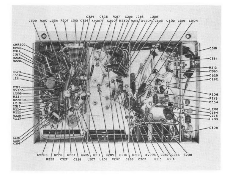
Figure 6-21. RF Subchassis, Bottom View, Rear Section
