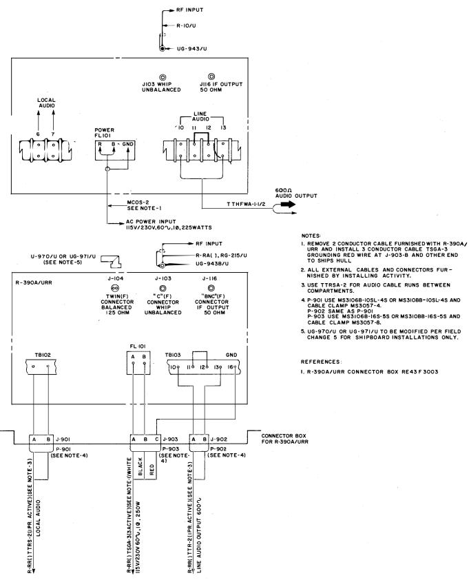
Figure 8-4. Interconnecting Cabling
