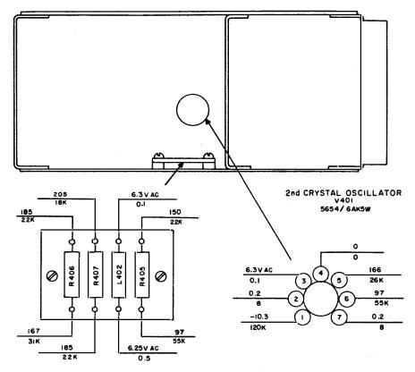
Figure 5-5. Crystal Oscillator Subchassis, Voltage Resistance Diagram
