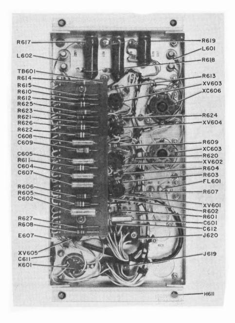
Figure 6-28. AF Subchassis, Bottom View
