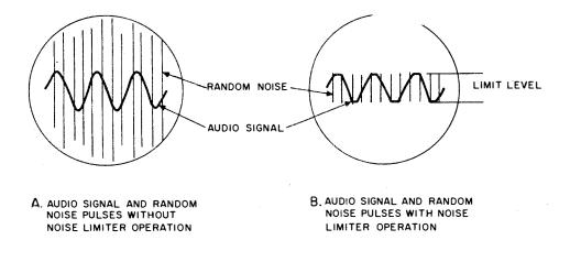
Figure 3-8. Typical Oscilloscope Presentation of Limiter Operation
