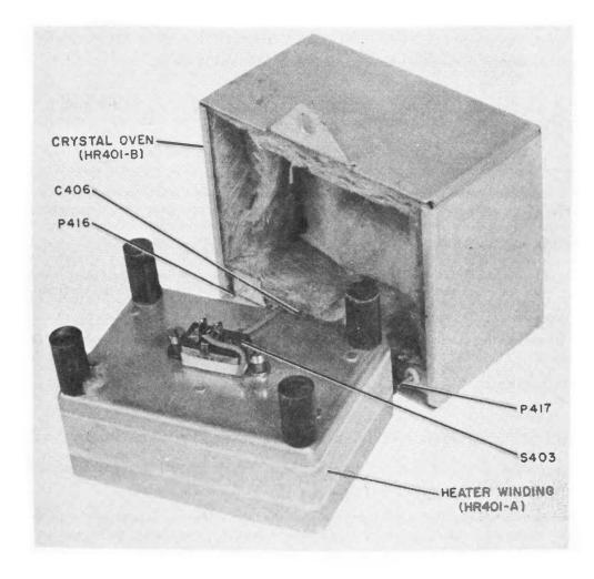
Figure 6-24. Crystal-Oscillator Subchassis, Internal View of Crystal Oven
