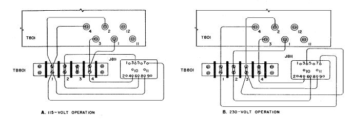
Figure 8-3. Connections for 115-Volt or 230-Volt Operation
