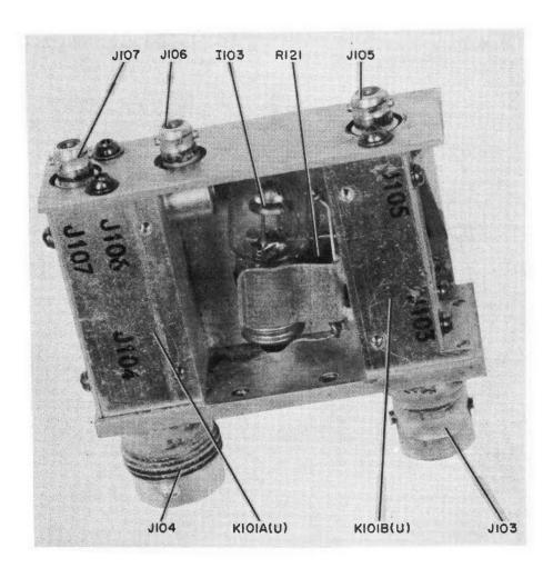
Figure 6-31. Antenna Relay Assembly, Internal View
