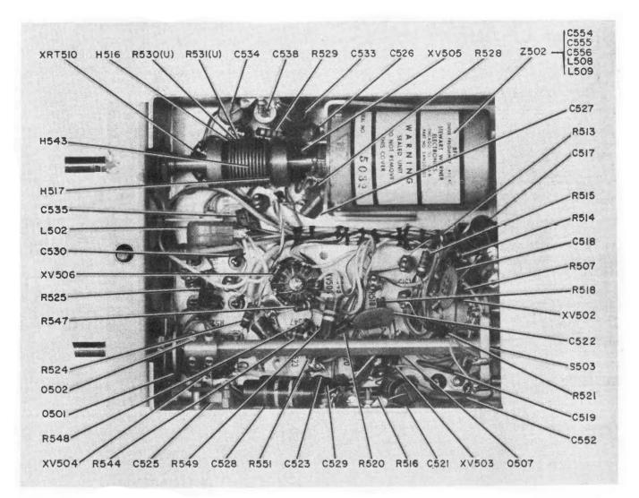
Figure 6-17. IF Subchassis, Front Section
