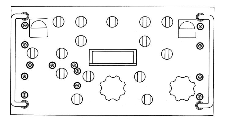
Figure 6-9. Location of Panel Mounting Screws
