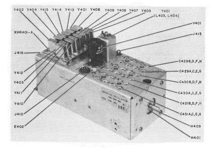
Figure 6-22. Crystal-Oscillator Subchassis, Top View
