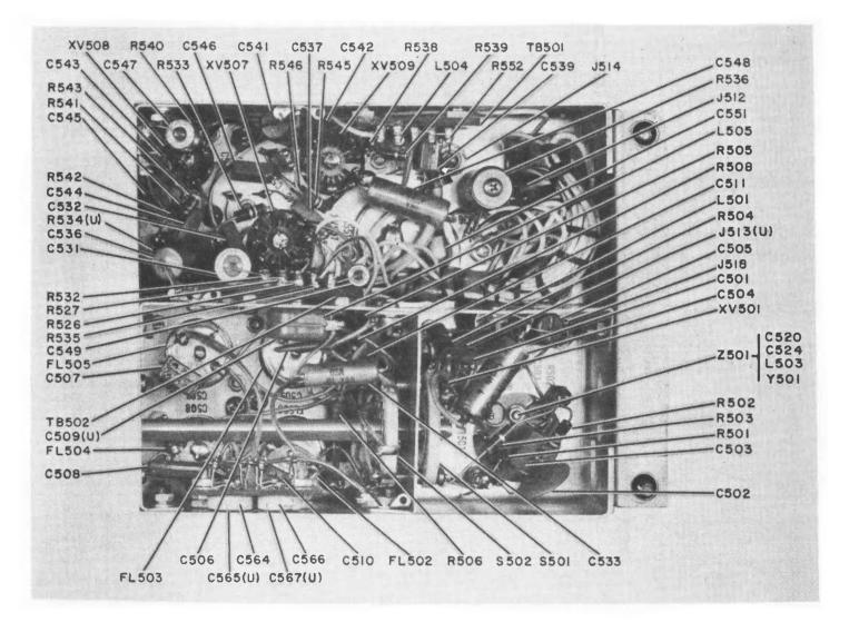
Figure 6-18. IF Subchassis, Rear Section
