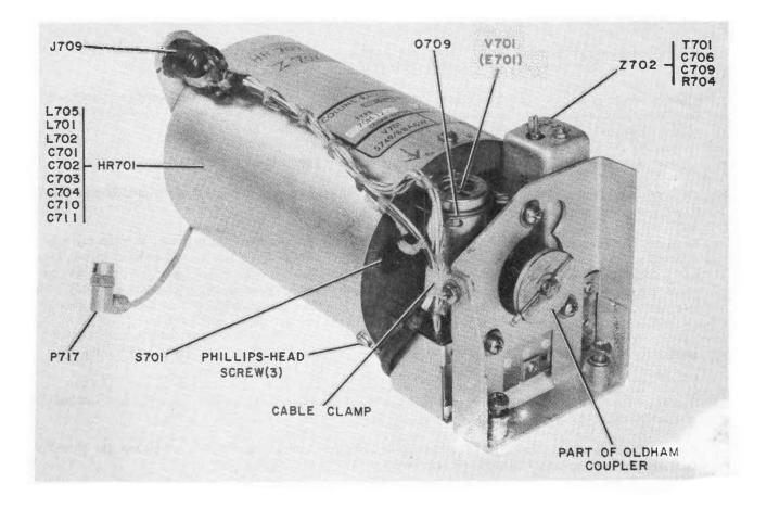
Figure 6-25. VFO Subchassis, Top View
