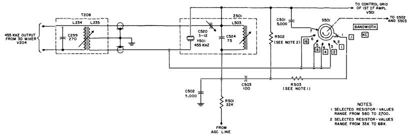
Figure 3-4. Crystal Filter, Simplified Schematic Diagram
