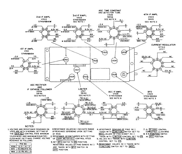
Figure 5-6. IF Subchassis, Voltage and Resistance Diagram
