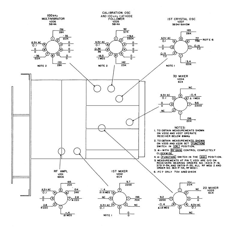
Figure 5-4. RF Subchassis, Voltage and Resistance Diagram
