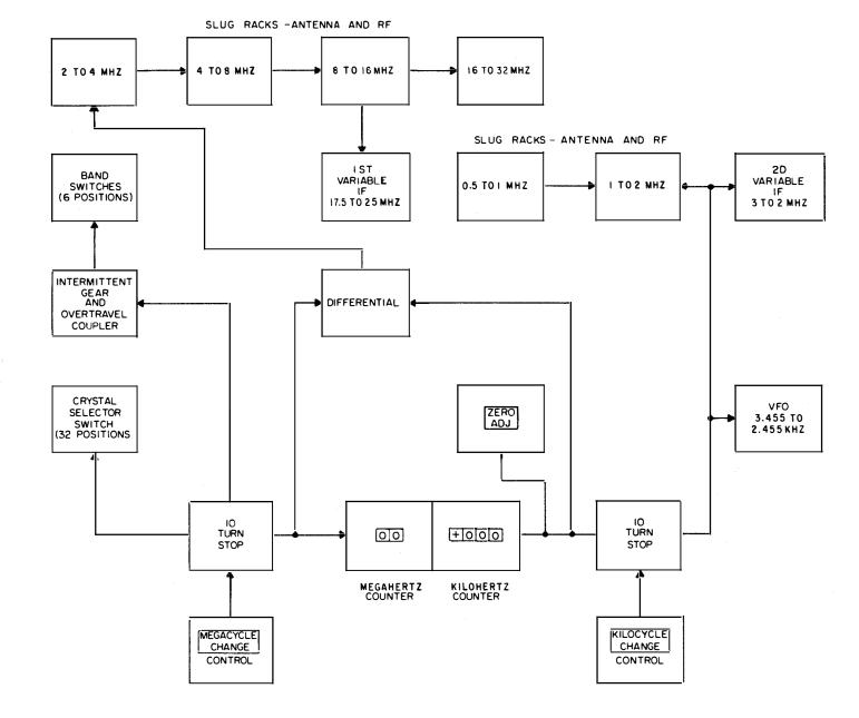
Figure 3-9. Tuning System, Mechanical Block Diagram
