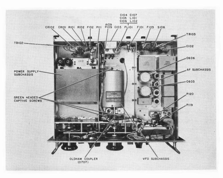
Figure 6-15. Radio Receiver R-390A/URR, Bottom View
