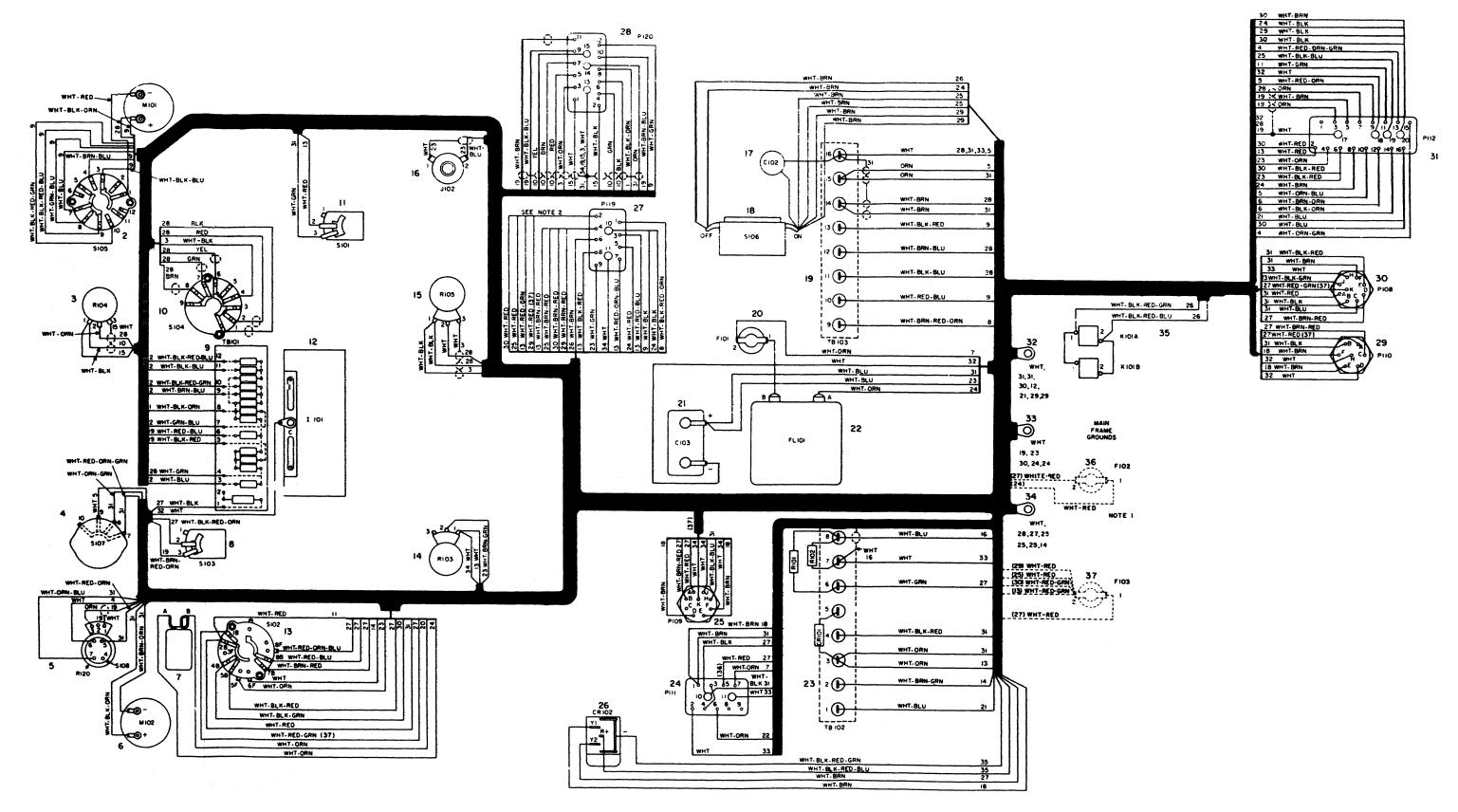
Figure 6-35. Radio Receiver R-390A/URR Main Frame Wiring Diagram
