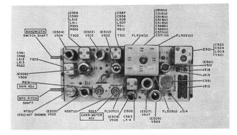
Figure 6-16. IF Subchassis, Top View
