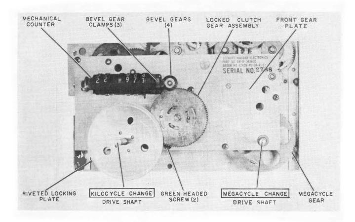
Figure 6-1. RF Gear Train Assembly, Location of Parts
