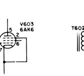
FIELD CHANGE NO. I SUPPRESSOR GRID CONNECTED TO CATHODE
