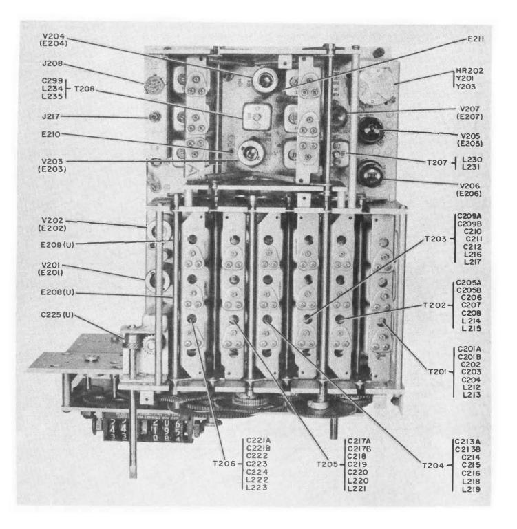
Figure 6-19. RF Subchassis, Top View (Sheet 1 of 2)
