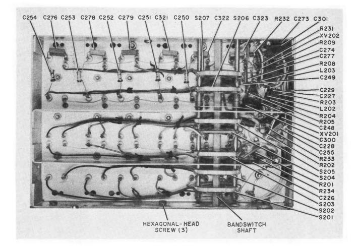
Figure 6-20. RF Subchassis, Front Section
