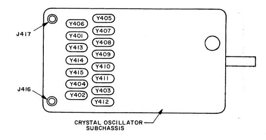
Figure 6-12. Location of Crystals Y401 through Y415
