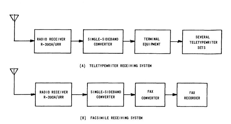
Figure 1-2. System Applications for Teletypewriter and Facsimile Equipment
