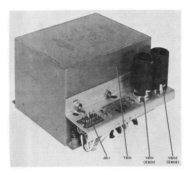
Figure 6-29. Power-Supply Subchassis, Top View
