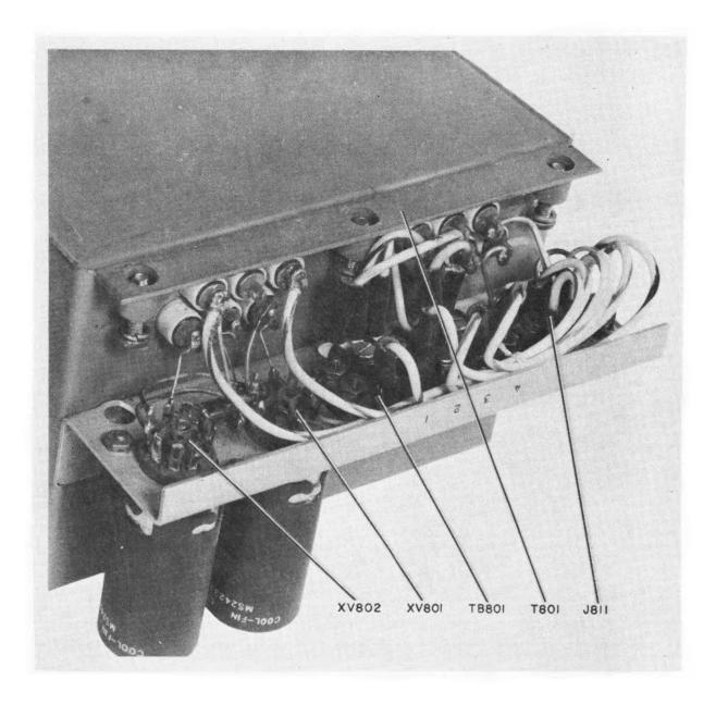
Figure 6-30. Power-Supply Subchassis, Bottom View
