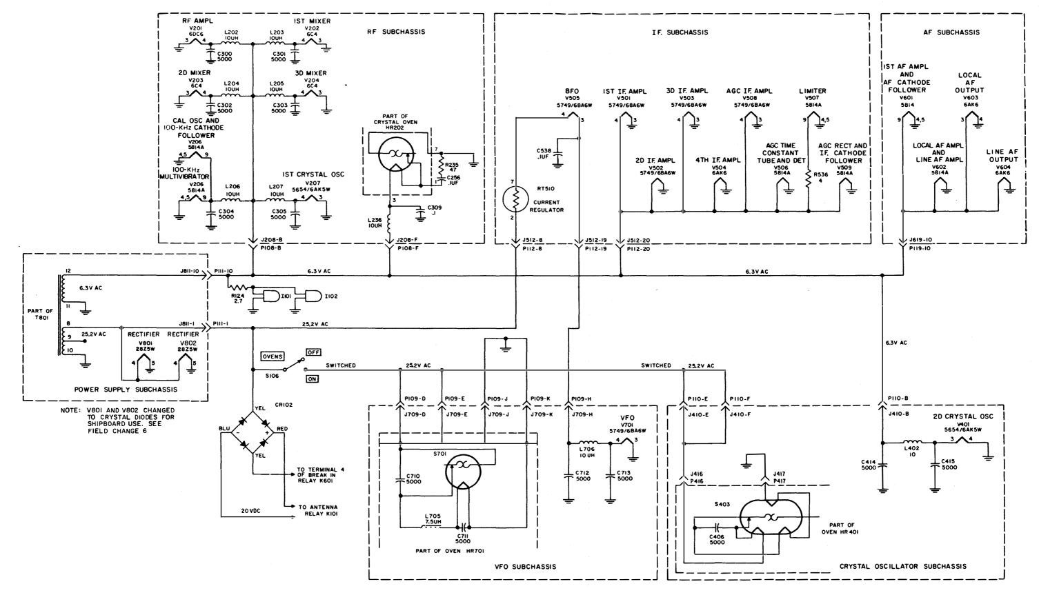
Figure 5-14. Filament and Oven Circuits
