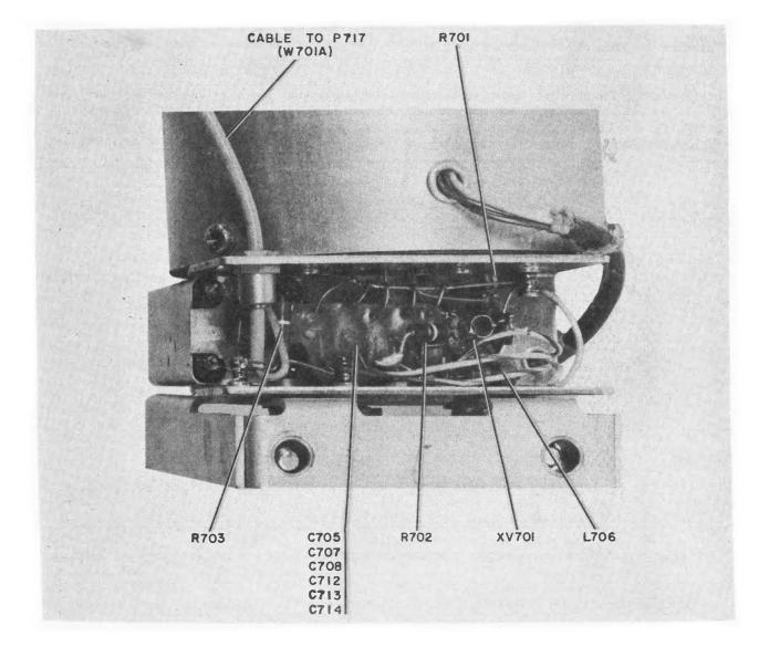
Figure 6-26. VFO Subchassis, Bottom View
