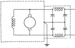
FIGURE 2-More effective interference suppression is obtained with this inductance-capacitance filter.
