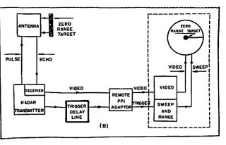
Block diagram showing location of the delay line to compensate for fixed range-error.
