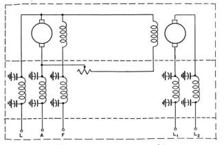
FIGURE 3-All external connections to this motor-generator unit are filtered.
