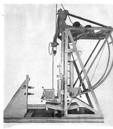
Light-weight shock-testing machine at N.R.L. The equipment under test is shown at A, mounted on fixture equipment is attached to the anvil plate. B and C are the D, which is attached horizontal and vertical hammers.
