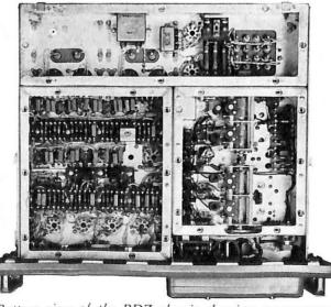
Bottom view of the RDZ chassis showing arrangement of components to provide maximum accessibility.
