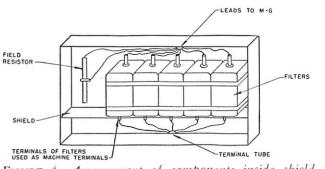
FIGURE 4—Arrangement of components inside shield case of filter unit.
