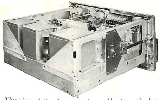
This view of the chassis-panel assembly shows the handle-operated locking device. Chassis may be locked when fully extended and, if desired, may then be tilted up 35 or 90° and locked in that position for servicing.
