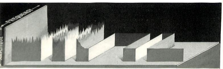
FIGURE 3.—Three-dimensional representation of a frequency-shift keyed telegraph signal.
