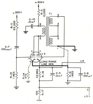
Circuit changes for increased long-range line brilliance. Added wires are shown heavy, and dashed lines indicate wires removed.
