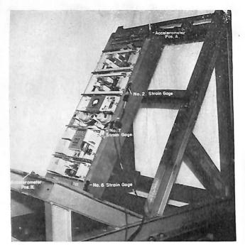
Typical arrangement of jigs and gauges for shock-testing equipment with the medium-weight shock-testing machine.
