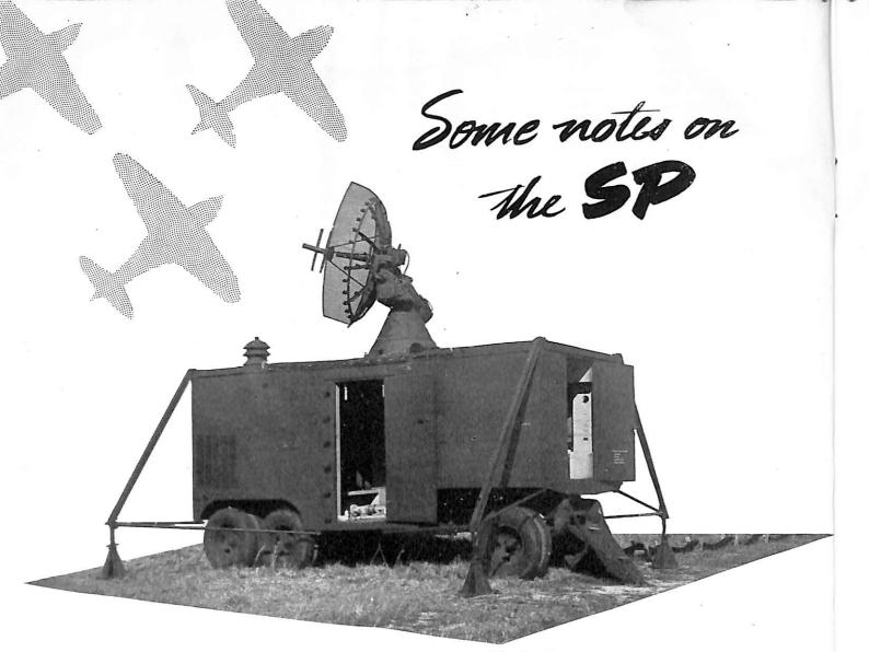
The Model SP-1M is an SP mounted in a trailer.
