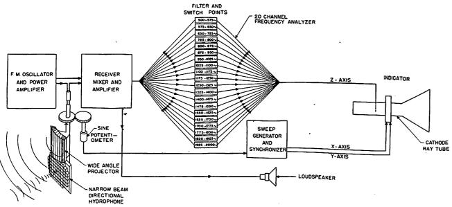
FIGURE 1-Block Diagram of Model QLA Sonar Equipment
