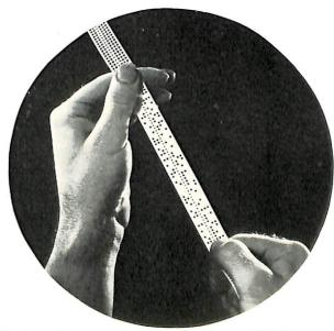
Perforated tape produced by the No. 19 TTY Set can be transmitted automatically.
