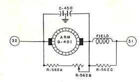
(c) Connect both a 250-ohm 10-watt wire-wound resistor and a 1500-ohm 25-watt variable potentiometer (if available) in series. This combination should then be connected in parallel with the armature as shown in the figure.
