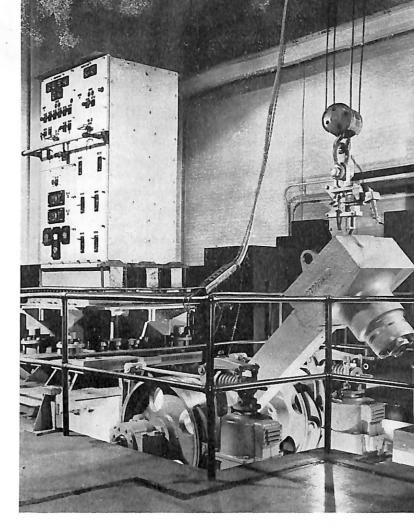
The medium-weight shock-testing machine at Westinghouse. When released, the hammer starts downward, then swings upwards to strike the anvil plate from
