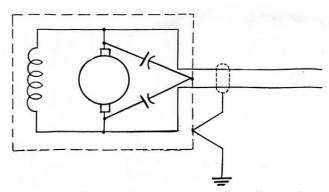
FIGURE 1—Simple filter consisting of small capacitors connected between brushes and motor frame.
