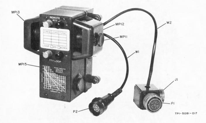
Figure 5-6. CV-2455/PRC-47, External Connection Identification
