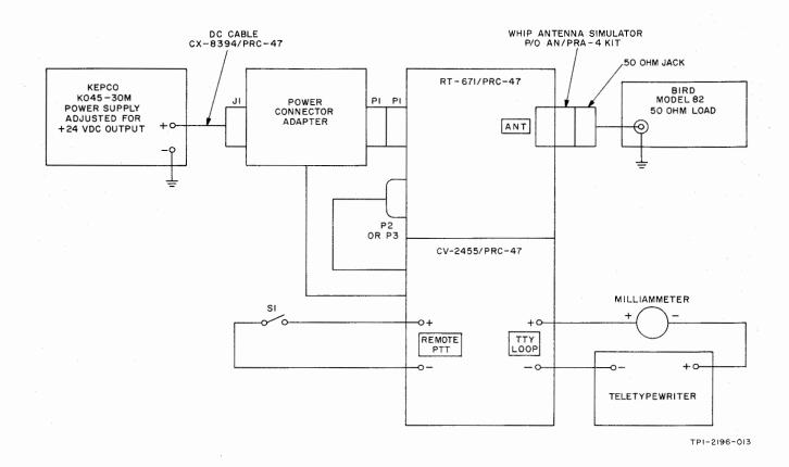
Figure 4-4. System Checkout, Test Setup
