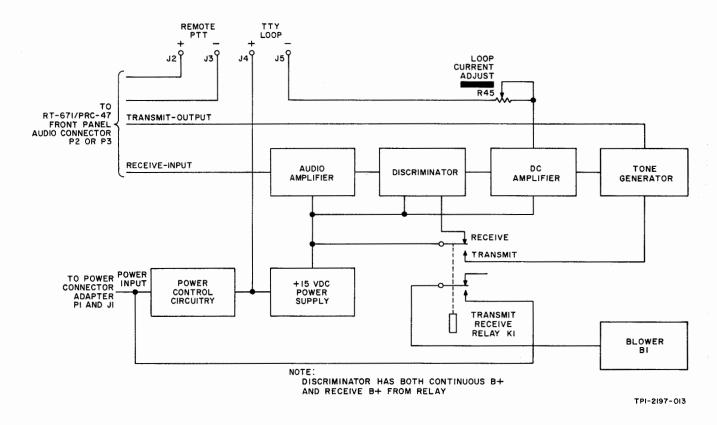
Figure 4-1. Converter-Blower CV-2455/PRC-47, Functional Block Diagram
