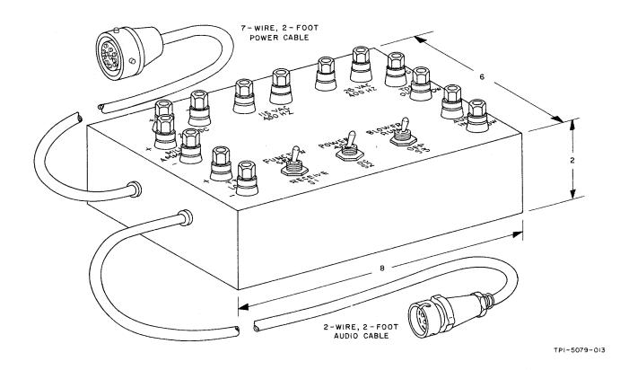
Figure 5-1. Suggested Fabrication Layout For Junction Box to Test Converter-Blower CV-2455/PRC-47
