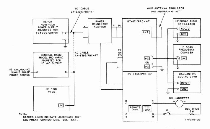
Figure 4-3. Receive Operation, Test Setup
