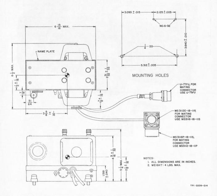
Figure 2-1. Converter-Blower CV-2455/PRC-47, Outline and Mounting Dimensions
