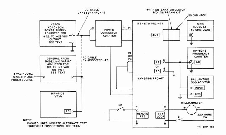
Figure 4-2. Tone Generator Operation, Test Setup
