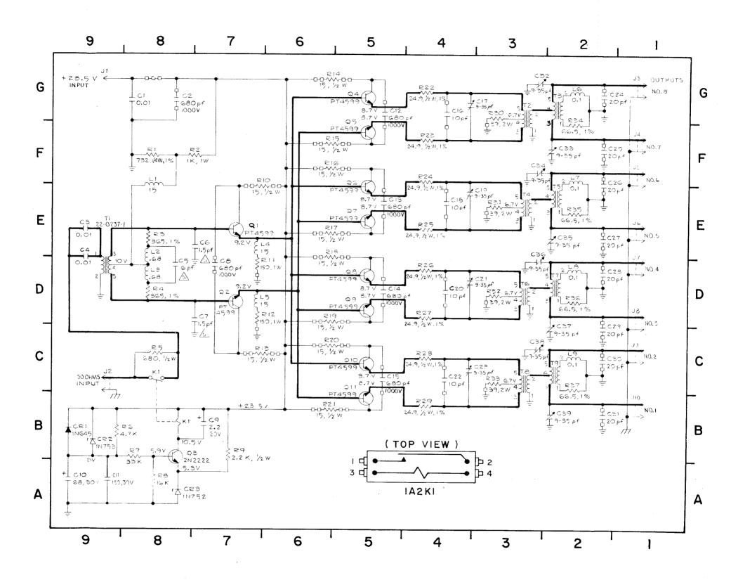
Figure 5-9. Divider Assembly, 1A2, 34-0086-2, Maintenance Schematic Diagram
