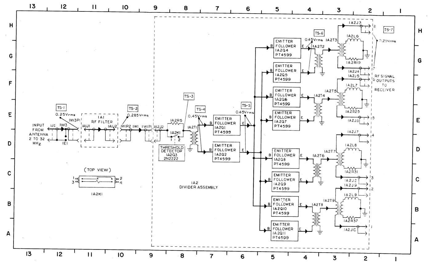
Figure 5-1. RF Signal Flow Diagram
