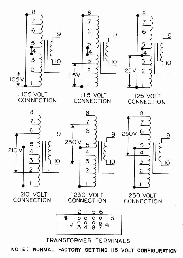
Figure 8-2. Transformer Connections
