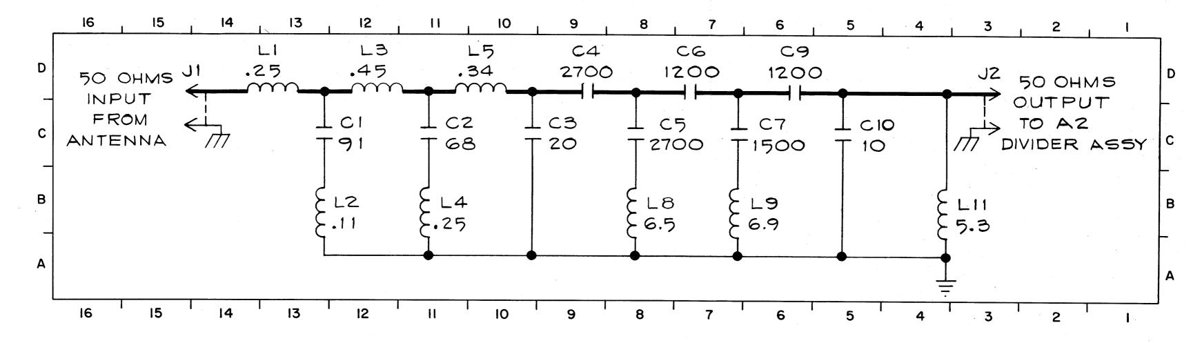
Figure 5-7. RF Filter, 1A1, 34-0122, Maintenance Schematic Diagram
