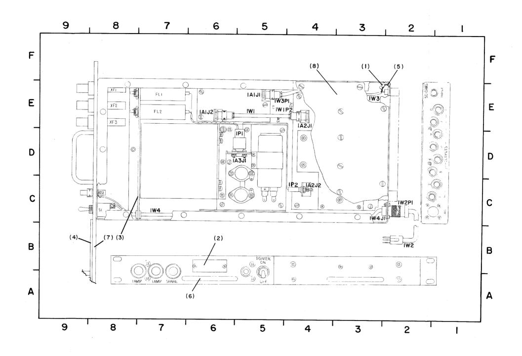
Figure 7-1. Antenna Coupler, Parts Location
