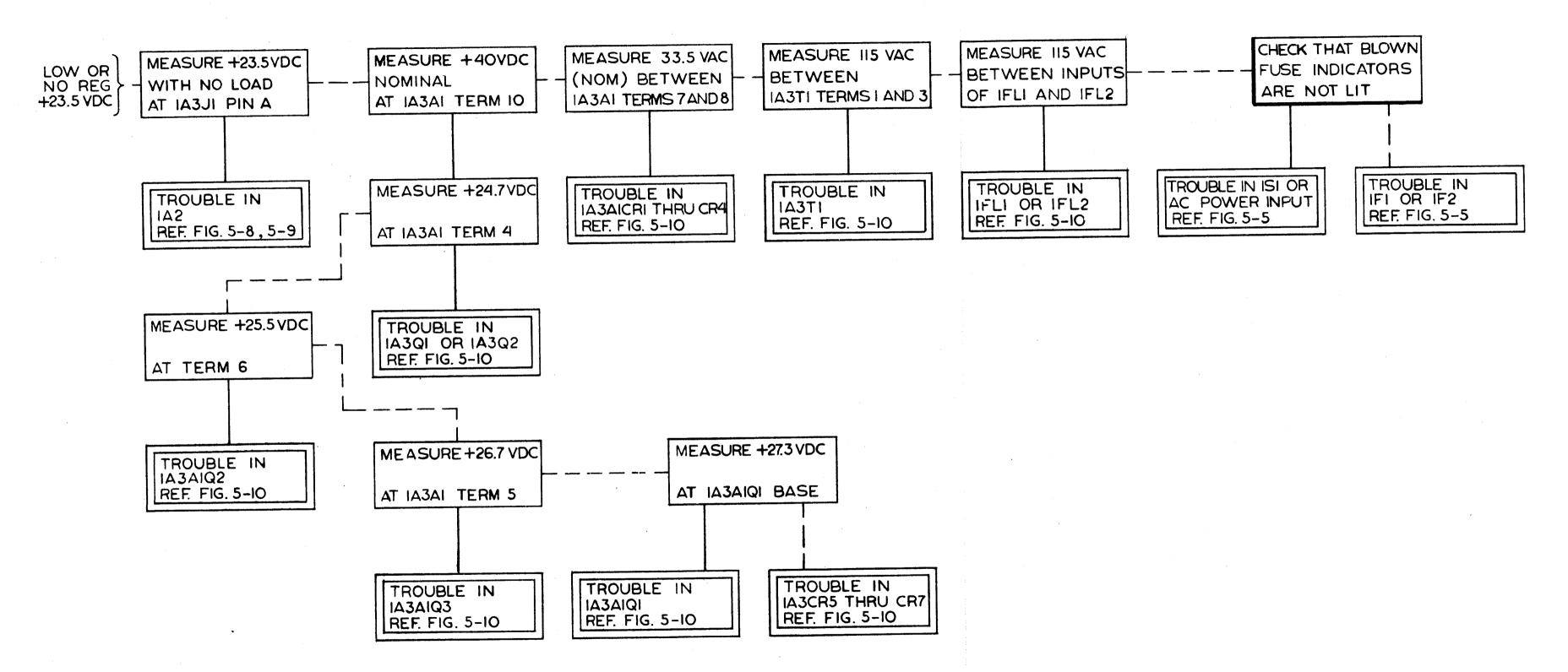
Figure 5-4. Power Distribution Fault Logic Diagram
