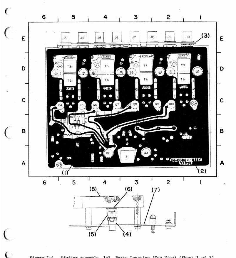
Figure 7-4. Divider Assembly, 1A2, Parts Location (Top View) (Sheet 1 of 2)
