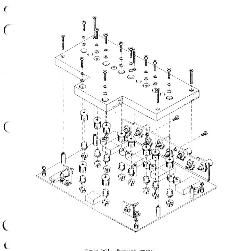
Figure 5-11. Heatsink Removal
