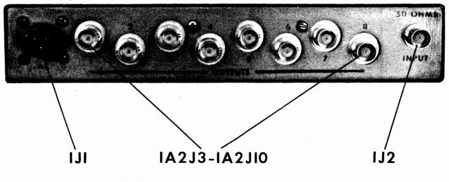
Figure 2-2. Antenna Coupler, Rear Panel Connectors
