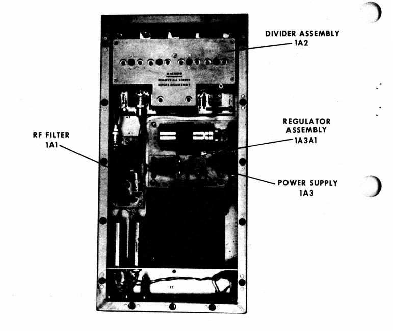
Figure 1-2. Antenna Coupler, Top View, Cover Removed
