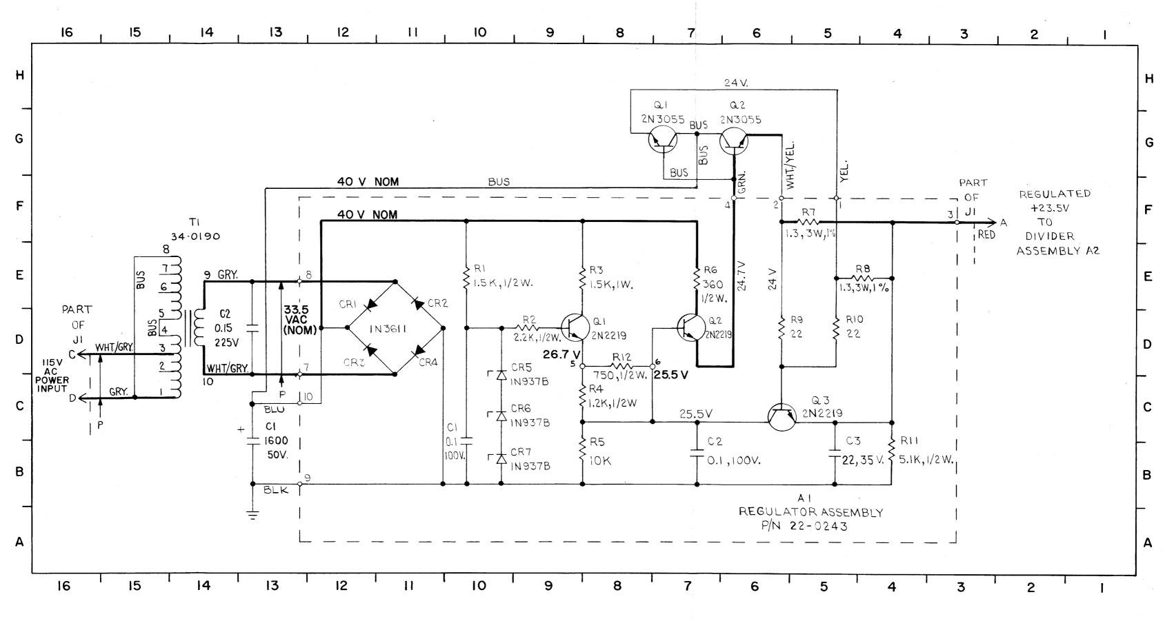
Figure 5-10. Power Supply, 1A3, Maintenance Schematic Diagram 5-51/(5-52 blank)
