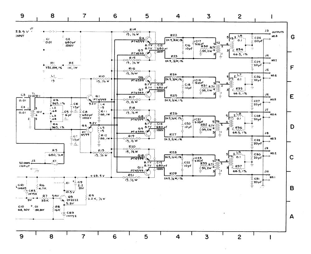
Figure 5-8. Divider Assembly, 1A2, 34-0086-1 Maintenance Schematic Diagram
