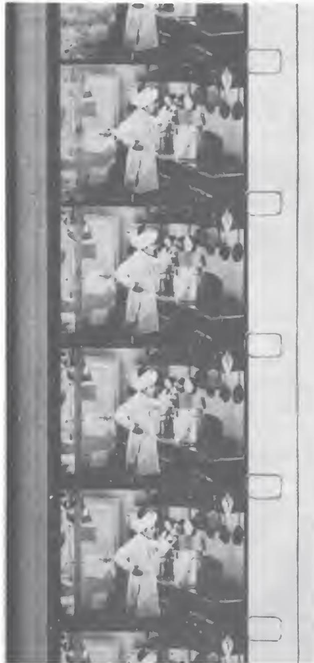
**Figure 11-6.—Section of a 16mm sound motion picture film.**
