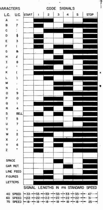
The standard Teletypewriter Code, used by the Model 28 Teletypewriter.
