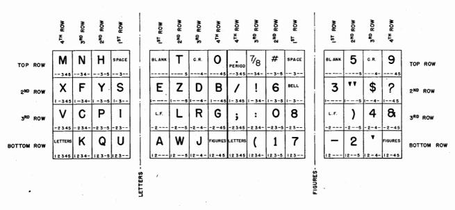
the hammer hits the pallet and the type box is returned CHARACTERS to the neutral position. There are two good reasons for having the type box return to the neutral position after each character is printed. First, it allows the operator to see what is being printed, and second, it eliminates the necessity for the type box to move more than four spaces horizontally during the positioning cycle or more than nine spaces during the shifting cycle.
